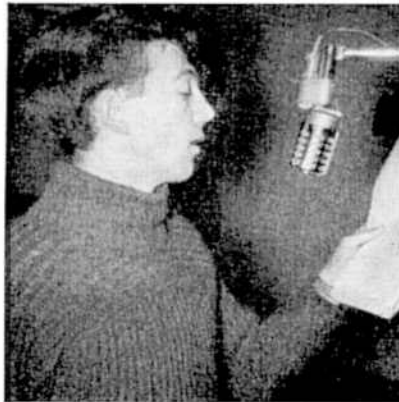
Illustrating professional boom suspension of Reslo Ribbon microphone
