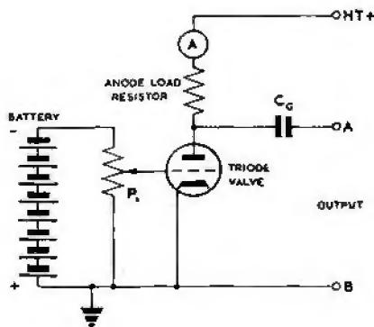
TEST CIRCUIT. IN THIS DIAGRAM A 12 VOLT BATTERY IS USED TO PROVIDE A NEGATIVE GRID BIAS VOLTAGE ON THE GRID OF THE TRIODE VALVE. THE THICK LINES — DENOTE THE NEGATIVE SIDE OF THE BATTERY (-) AND THE LONG LINES — THE POSITIVE SIDE (+). NOTE THAT THE + IS CONNECTED TO EARTH  $\downarrow$ . BY MOVING THE SLIDER OF THE POTENTIOMETER  $P_1$  WE CAN VARY THE VOLTAGE WHICH APPEARS ON THE GRID OF THE VALVE.  $R_A$  IN FIGURE 1 REPLACES THE BATTERY SHOWN IN FIGURE 2 BUT IT DOES THE SAME JOB.
