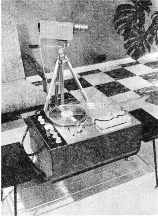
The 'Telcan' video recorder which can be used the way the tape recording enthusiast uses his sound tape recorder today.
