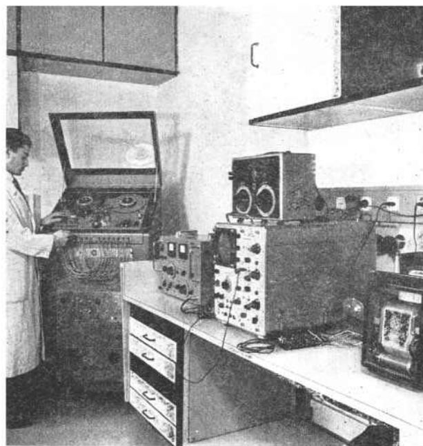
Fig. 3—Equipment for pulse testing of tapes: → one of the many 'electronic' tests that tape undergoes during processing.
