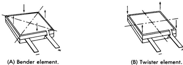
Fig. 4-5. Construction of crystal elements.
