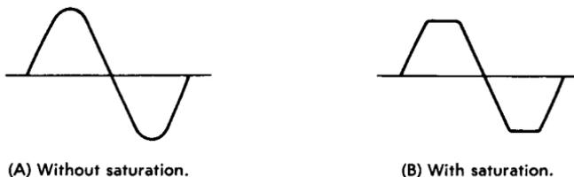
**Fig. 5-12. Waveform of a transformer in which the core is saturating.**
