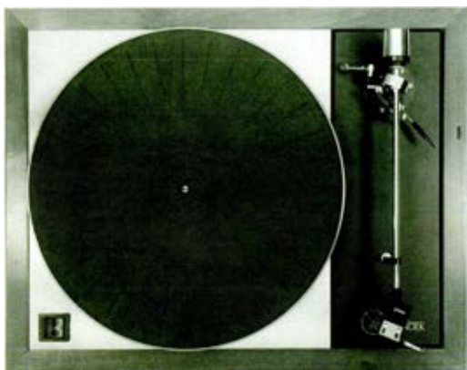
UK classics: Linn Sondek LP12 turntable (with original rubber mat!) fitted with Grace arm and Supex cartridge and (right) the immortal BBC LS3/5A loudspeaker
