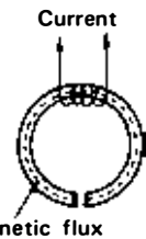
Fig. 4—3 STRUCTURE OF TAPE HEAD
