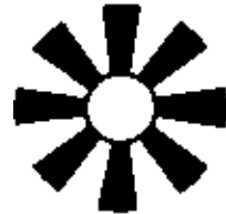
Fig. 2—8 PAIR OF COPPER FILMS ACT AS CAPACITIVE MOTOR CONTROL DEVICE.
