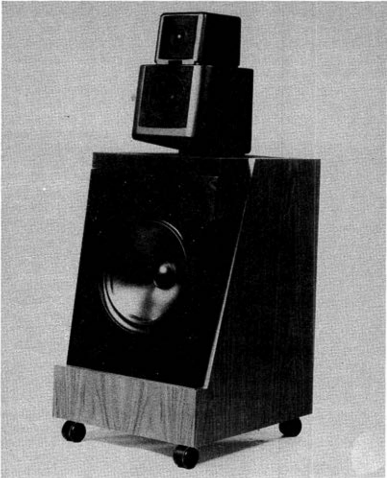
Figure 6.2 (c) A three-way system with time aligned drivers, 24 dB/octave, crossover (acoustic) and low diffraction enclosure forms (courtesy KEF Electronics)
