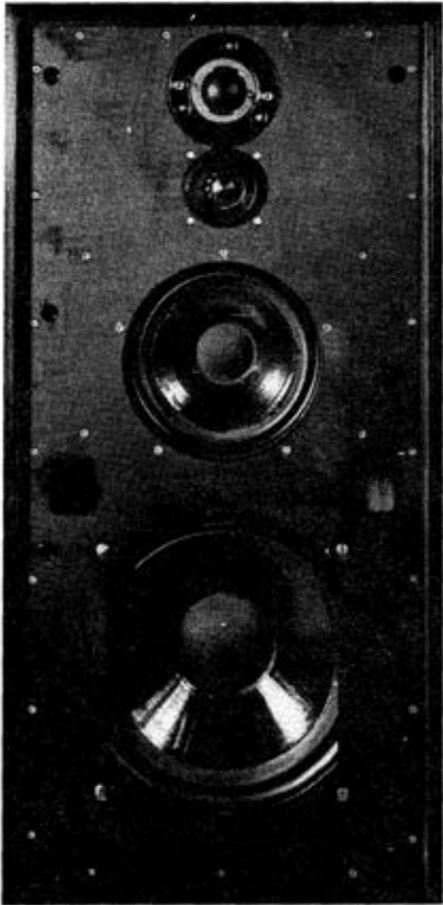
Figure 6.3 A four-way vertical in-line system (18 dB/octave electrical crossover with controlled listening axis) (BC3, courtesy of Spendor Ltd.) (300 mm bass, 200 mm mid, 38 mm and 19 mm treble drivers)
