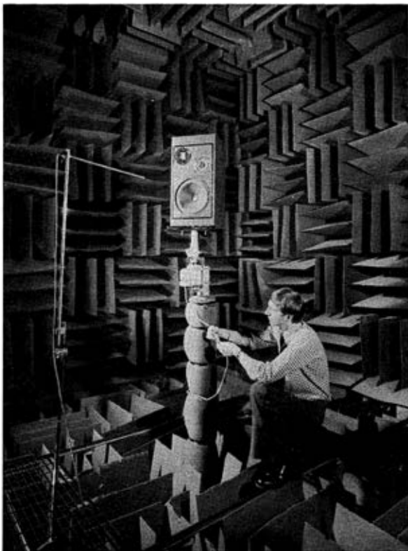
Figure 8.11 Anechoic chamber (courtesy Acoustic Research)
