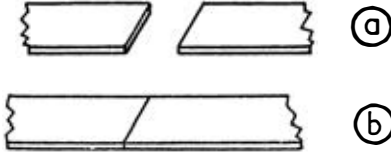
FIG. 101. A DIAGONAL JOIN MAKES THE JOINT MORE SILENT WHEN PASSING OVER THE REPLAY HEAD.
