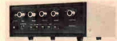
HD  $< 0.8\%$  (at rated output); IM  $< 0.8\%$  (at rated output); hum & noise  $> -60$  dB (at phono input); sensitivities: mag phono 2.0 mV, aux 150 mV, tuner 150 mV, tape 150 mV, tape head 1.5 mV; hi-cut filter; lo-cut filter; loudness compensation (switch); ganged tone controls; headphone output; damping factor 20; tape monitoring;  $4\frac{3}{8}$ " H x  $11\frac{1}{2}$ " W x  $10\frac{1}{2}$ " D; \$119.95.
