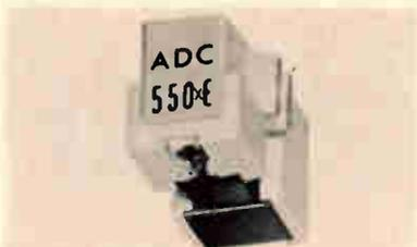
frequency response 10-20,000 Hz at  $\pm 2.0$  dB; stylus  $0.3 \times 0.7$  mil elliptical; tracking force  $\frac{3}{4} \rightarrow 2$  g;  $15^\circ$  tracking angle; channel separation nominally 20 dB from 50-12,000 Hz; compliance  $35 \times 10^{-6}$  cm/dyne; stylus replacement #R-50XE; price \$50.00.
