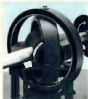
Unique gyrosopic gimbal suspension centers and balances tonearm within two concentric rings. All four pivots have identical low-friction, hardened steel-point bearings. Vertical friction less than 0.007 gram, horizontal friction less than 0.015 gram.
