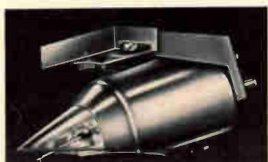
llyptical; tracking force  $1 \rightarrow 1\frac{1}{2}$  g;  $15^\circ$  tracking angle; channel separation  $>25$  dB at 1000 Hz; compliance  $25 \times 10^{-6}$  cm/dyne; stylus replacement #5430; \$69.95.
