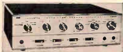
22-20,000 Hz response at  $\pm 1.0$  dB; HD < 1.0% (at rated output); hum & noise -75 dB (at aux input); sensitivities: mag phono 2.2 or 7.0 mV, ceramic phono 75 mV, aux 250 mV, tuner 150 mV, tape 500 mV; hi-cut filter; lo-cut filter; loudness compensation (switch); independent tone controls; multiple speaker switching; headphone output; tape monitoring; 3 $\frac{1}{8}$ " H x 13" W x 9 $\frac{1}{4}$ " D; \$139.95.
