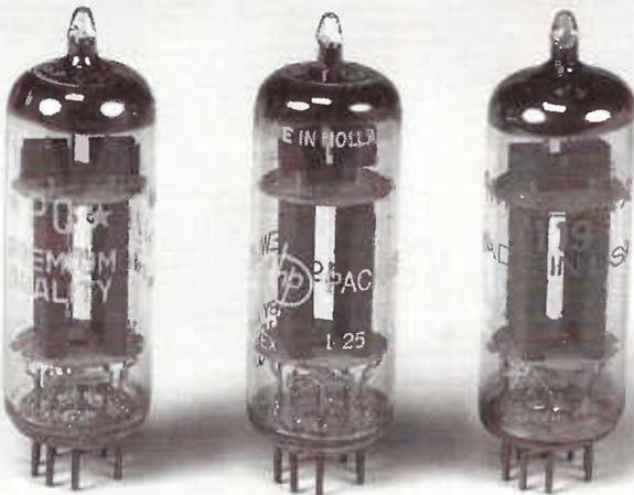
structure and a gm = 15,500  $\mu$ mhos at 36 ma. This type was brought into America as the 7119 by Amperex. Some later military 7119s were built here.
