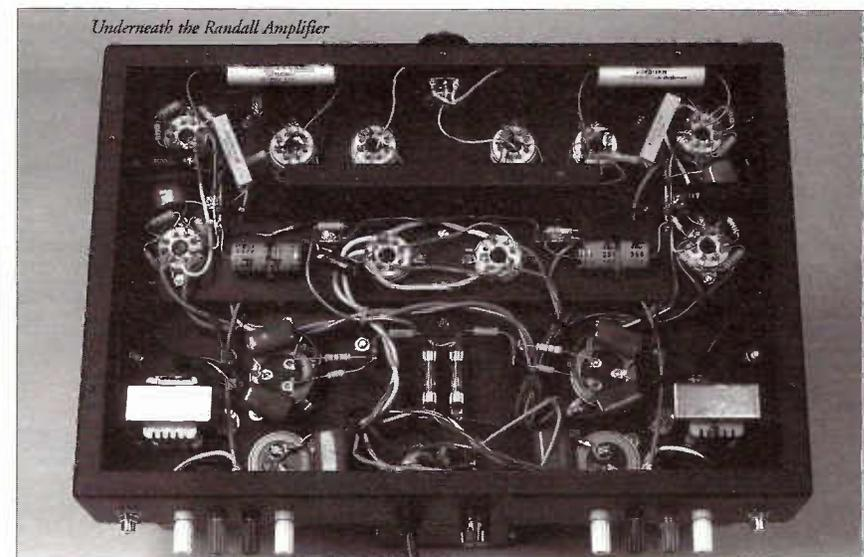
and 16 ohm outputs. The maximum power is about 13 watts per channel before clipping. A small amount (3db) of negative feedback is used to increase the speaker damping factor and reduce distortion. The BFT-1 power transformer
