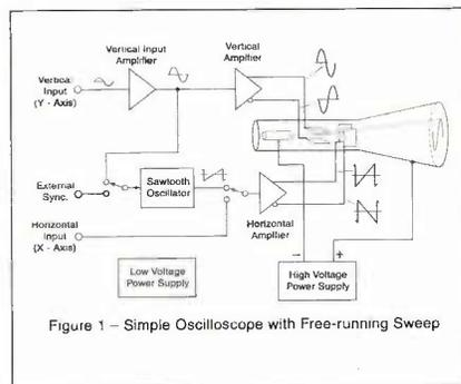
Figure 1 - Simple Oscilloscope with Free-running Sweep
