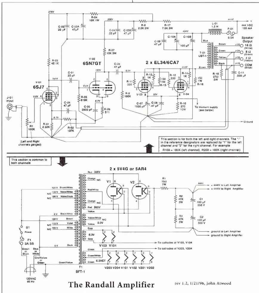
The first stage is a triode-connected 6SJ7 biased at 3 mA. This has a mu of 20, making it similar to a 6J5 or 1/2 a 6SN7GT. The second stage uses a 6SN7GT with both sections paralleled, biased at 11 mA. The small cathode capacitor (C-05) is used to boost the output at high frequencies to compensate for the capacitive loading of the output stage. This technique, called "cathode compensation" was originally developed for use with video amplifiers.
