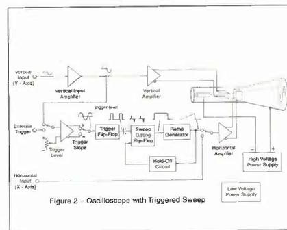
Figure 2 - Oscilloscope with Triggered Sweep
