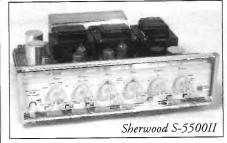
Sherwood integrated amplifiers are attractive, common and can sound good with the servicing and the right upgrades. There are several versions of the S-5000 and S-5500 that can use: 7189s, 7591s or 7868 output tubes. All of the stereo integrated amps have solid-state rectification. Sherwoods have lots of controls for phonograph fanatics including a presence control on some models.
