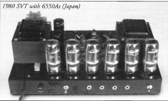
levels. While the 6146B/8298As held up to the mechanically abusive environment of taxi cabs, they were shown to be less tolerant of the abuse provided by the Rolling Stones—they would self-destruct when pushed into clipping for extended periods. Which, of course, the Stones did continuously. The SVT would soon be redesigned for six 6550 beam power tubes.
