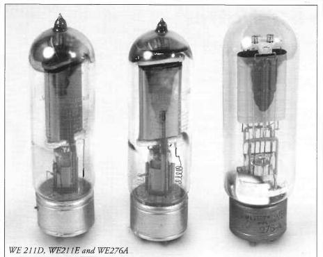
Western Electric's versions started with the 211A; the 211B, C and D were just the same tube with different grades of filament. The 211E was notorious for its use in the WE 43A theater amplifier. A pair of small nichrome-wire inductors were installed in the filament circuit, inside the actual tube, to help stabilize it at high frequencies. This makes old 211Es highly collectible.
