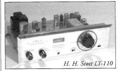
and LT-110B. All of these units have a built-in multiplex decoder and can receive stereo signals. The chassis is aluminum and wiring is point-to-point. Later tuners used solid-state rectification. The Scott tuners are plentiful and cheap, so finding one shouldn't be a problem.
