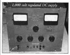
driver stage is obtained by using a standard radio-type power transformer running into a voltage doubler. The 6AX4GT damper tube rectifiers give a nice slow turn-on. The 6AX4GT is abundantly available in North America as a surplus TV tube.
