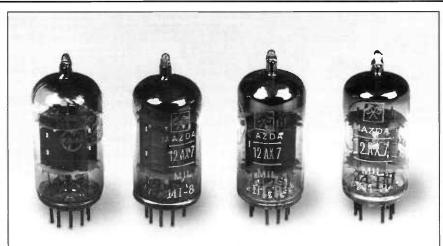
Matsushita 12AX7 1960s, Mazda 12AX7 Long Plate 1955, Mazda 12AX7 Short Gray Plate 1957, Mazda 12AX7 Short Bright Nickel Plate 1963
