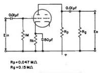
CLASS A RESISTANCE-COUPLED AMPLIFIER, EACH SECTION
