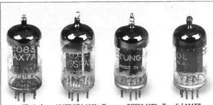
Westinghouse 12AX7 USA 1973s, Tungsram ECC83 1970s, Tung-Sol 12AX7 Black Long Plate 1950s, Tung-Sol 12AX7 Long Gray Plate 1960s
