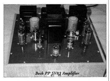
The Svetlana Web Page (www.svetlana.com) has both the data sheets for the SV83 and Application Note #29 for data on wiring in a screen supply with very few parts. Many very highly regarded amps of the past used true pentode connection, including all H. H. Scott amplifiers, the Grommes 260 and some Altec PA amps.
