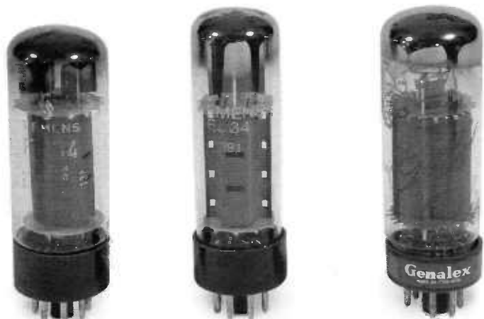
Siemens EL34 (actually an Xf2 Mullard) (1970s), Siemens EL34 Slim Bottle-Dimple Top (1991) and Genalex KT77 Gold Lion Early (1970s)
