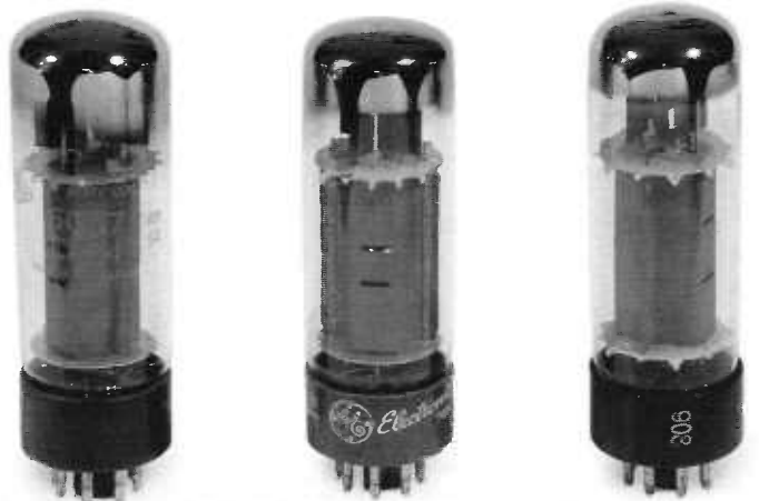
Amperex Branded Xf2 (1960s), GE/Amperex Double-D Getter (1960s) and Telefunken EL34 (1960s)
