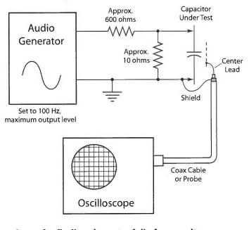
Setup for finding the outer foil of a capacitor.
