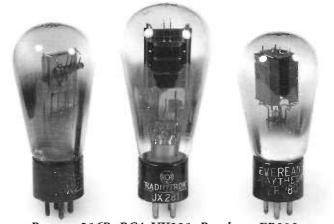
**Rectron 216B, RCA UX281, Raytheon ER280** RV120/350. The Tungsram company started as a firm in Ujpest, Hungary, which had some manufacturing in the
