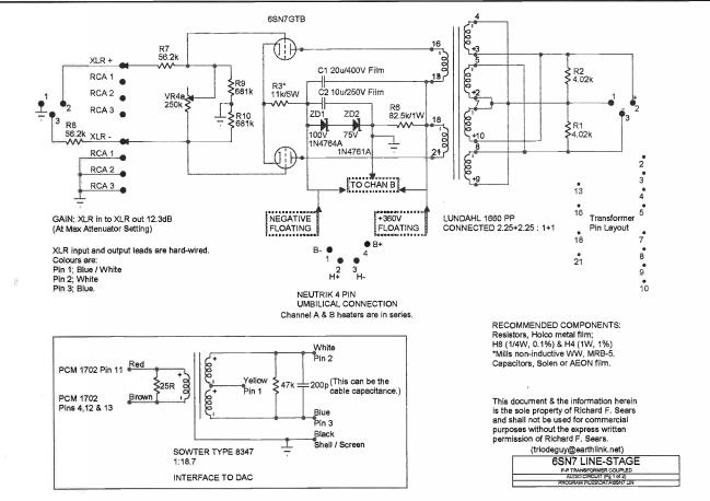
of 8.74k. This is in parallel with a 47k resistor placed across the secondary (per Sowter recommendation) giving a balanced source impedance of 7.4k or 1.84k for each phase. In balanced input mode, the minimum load presented is 2 X 51.1k, thus significantly greater than 10X the source impedance.
