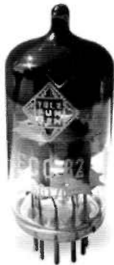
Counterfeit Telefunken 12AU7 (No diamond on the base)
