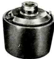
NEW SPECIAL PM HORN UNIT, having Alnico V magnet ring, completely watertight, housed in a heavy aluminum spinning. Provides extremely high efficiency reproduction with minimum input. Handling capacity 35 watts continuous, 60 w. peak.
