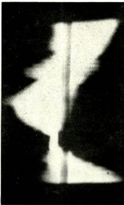
Fig. 3. Half-cycle envelope of noise modulation obtained from playing back tone groove. This is an exaggerated case, however, and Fig. 6 shows a more typical stylus.
