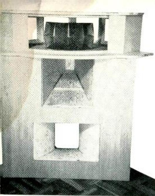
Fig. 3. Front view of the new speaker during construction, showing the speaker well and the TV tube enclosure.
