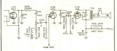
Fig. 1. Audio section schematic of RCA 630TS receiver chassis.
