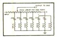
Fig. 3. Electrical circuit of continuous loudness control.
