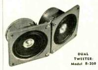
High tones, brought out with new degree of realism, now made acceptable to the ear by Bozak system of rubber damping. Direct radiated highs dispersed over wide angle. Clean smooth response makes high frequency listening a pleasure. No shrill "piercing" Response: 1500—beyond 13,000: Cones: 2½" dia. with aluminum alloy apex; Coverage: 120 deg. at 10 kc., 100 deg. at 13 kc: Rating 5 watts: 7 oz. Alnico V permanent magneta; 327,50 list. (Patents pending).
