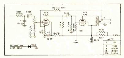
Fig. 3. Circuit used when it is desired to include the output transformer in the feedback loop.
