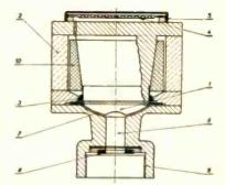
Fig. 3. Cross section of driver unit to show internal construction.
