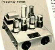
A new design giving a high degree of noise suppression with a frequency range of 40 to 15,000 cycles.
