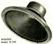
Twelve-inch unit specially developed for low resonance. Not only are low frequency tones distinctly audible, but they have the rich fullness of true orchestral bass. Unique Bozak cone climinates "drumhead" characteristic common to many woofers, Response: 40-3500 cycles: Rating: 12 watts: 22 oz. Alníco V permanent magnet using special low carbon cast pole pieces. \$52.50 list.
