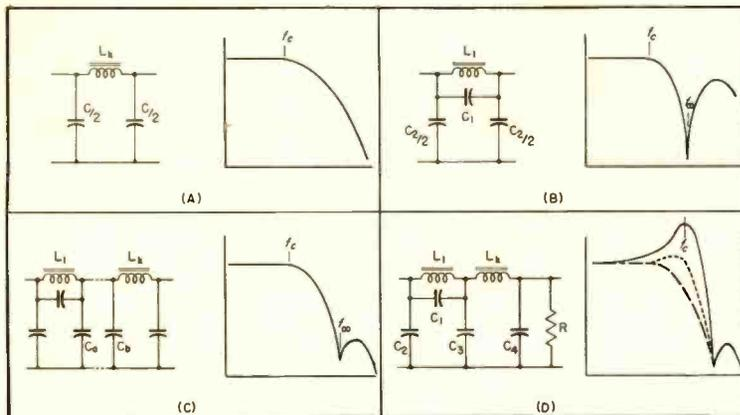
Fig. 3. (A) Constant- $k$  low-pass filter section, with typical response curve; (B)  $m$ -derived section; (C) combined sections with resulting curve; (D) complete filter with terminating resistor. Solid curve shows response when  $R = 0.5$  meg; dashed line is curve for tabular values of  $R$ ; dotted curve for  $R$  above optimum.
