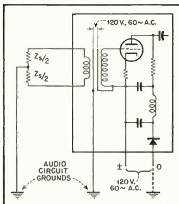
**Fig. 13. Analysis of source of noise in an a.c.-d.c. amplifier.**
