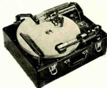
Fairchild Unit 523 is used in fixed studio installations for dubbing sound tracks for motion picture production. Absolute lip synchronism is guaranteed for use with your cameras and projectors. You get this same performance with the portable Fairchild Unit 539-G Disk Recorder shown at left. Many motion picture sound tracks are first recorded on FAIRCHILD SYNCHRONOUS DISK RECORDERS.
