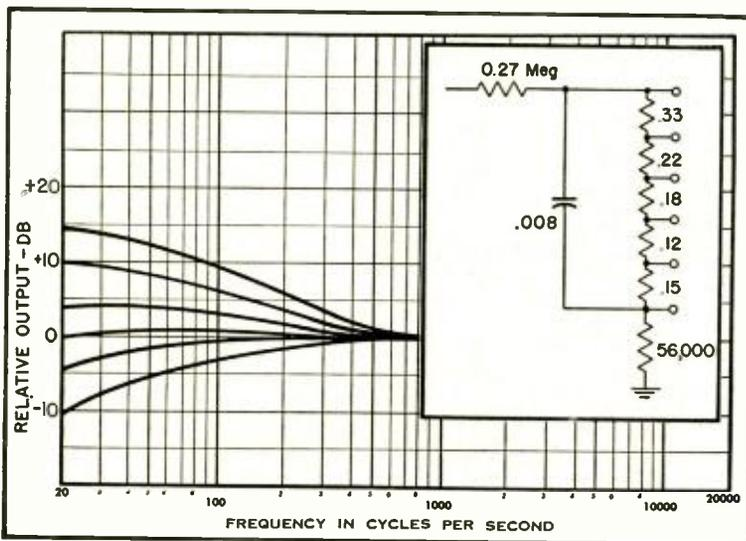
Fig. 2. Circuit of bass-boost control (insert) and curves obtained when working into unloaded grid.
