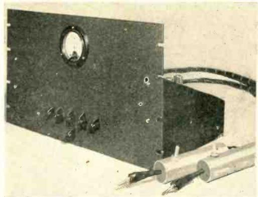
Description of an instrument designed to measure accurately the phase difference between two audio signals of equal or differing magnitude.
