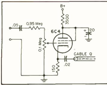
**Fig. 2. Input probe with signal level adjustment built into the tube housing.**
