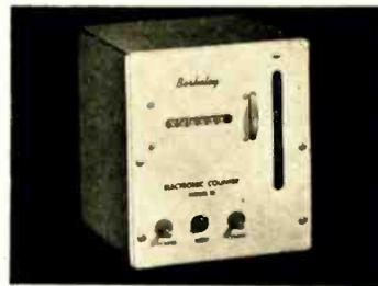
Model 10 is unique in the fact that all circuits have been developed around a single tube type, the 12AU7, to facilitate replacement. Selenium rectifiers provide d.c. power supply. Manufactured by Berkeley Scientific Corporation, 2200 Wright Ave., Richmond, Calif.
