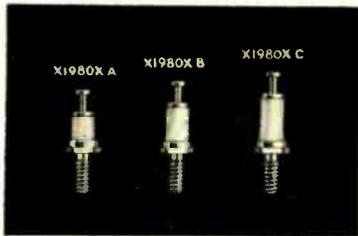
ing marketed by Cambridge Thermionic Corporation, 464 Concord Ave., Cambridge 38, Mass. The smallest of the new series, Type X1980XA, has an overall height of only three-eighths of an inch including terminal. Terminals are available in various lengths with voltage breakdown ratings up to 5800 volts. Additional data will be supplied by the manufacturer.
