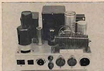
Fig. 4. Power supply used for the preamplifier unit.
