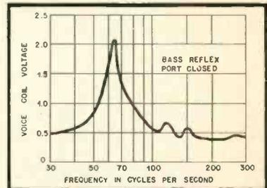
Fig. 5. This was the speaker impedance curve with the port completely blocked.
