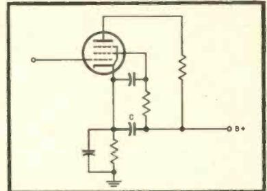
Fig. 15—14. Circuit for cancelling plate-supply ripple and regeneration due to inadequate filtering and decoupling. The value of  $C_1$  in relation to the cathode-to-ground impedance determines the value of the cancelling voltage. (After Wen-Yuan Pan)
