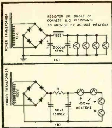
Fig. 15-9. A—Low voltage d.c. heater supply. B—Low current d.c. heater supply. R provides the correct voltage drop for the tube section and is preferably of the negative-temperature-coefficient type to protect the heaters from initial current surges.
