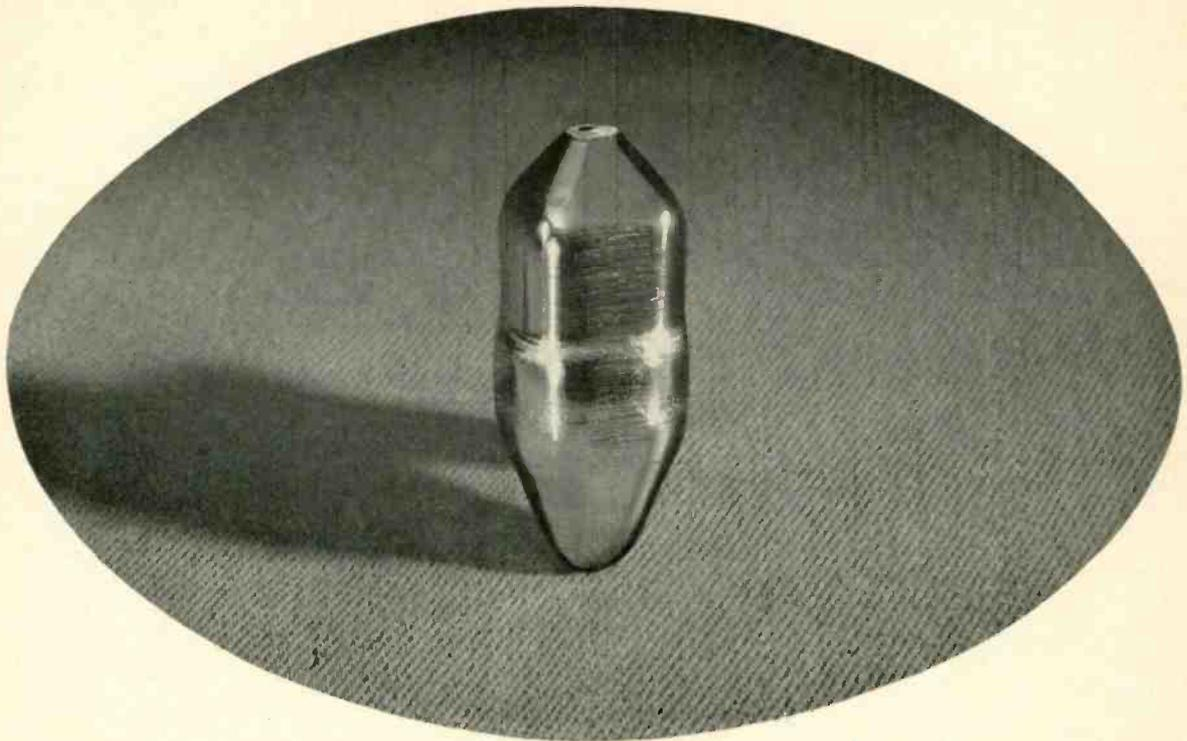
Germanium crystal grown at Bell Telephone Laboratories (life size). It is sliced into hundreds of minute pieces to make *Transistors*. Transistor action depends on the flow of positive current-carriers as well as electrons, which are negative. Arsenic—a few parts per 100,000,000—added to germanium produces prescribed excess of electrons. With gallium added, positive carriers predominate. Latest junction type *Transistor* uses both kinds of germanium in the form of a sandwich.
