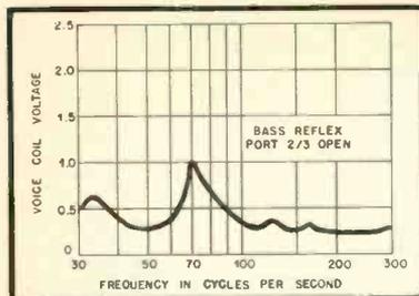
Fig. 7. A 48-square-inch port produced this curve.
