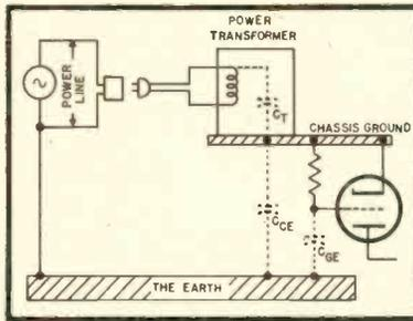
Fig. 15-8. Hum pick-up from the line due to grid-to-earth capacitance.  $C_T$  = capacitance between transformer primary and case,  $C_{CE}$  = capacitance between chassis and earth,  $C_{CE}$  = capacitance between grid and earth. For relief,  $C_{CE}$  must be shorted out by earthing the chassis, or the grid must be shielded from earth.
