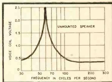
Fig. 2. Impedance curve of the unmounted speaker shows its 58-cps resonance.
