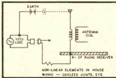
Fig. 15—13. Introduction of modulation hum in antenna circuit.
