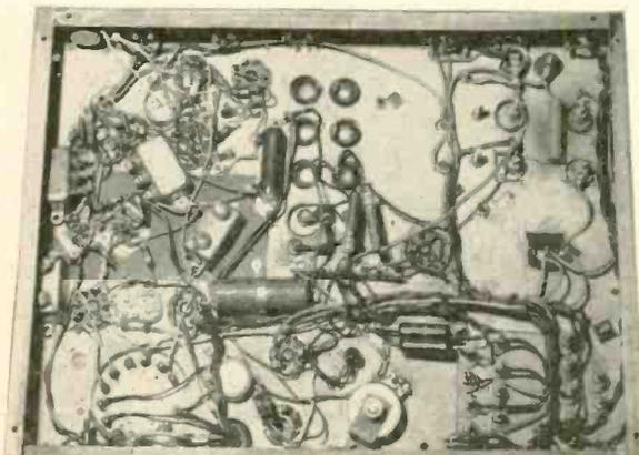
Fig. 3. Underside of the power amplifier chassis.
