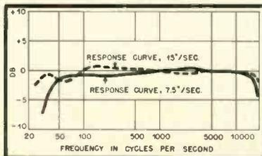
Fig. 10. Response curves of the M-80 at 7.5 and 15 inches per second.
