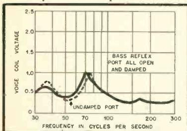
Fig. 9. Placing damping material over the port did not produce very great change, as these comparison curves indicate.
