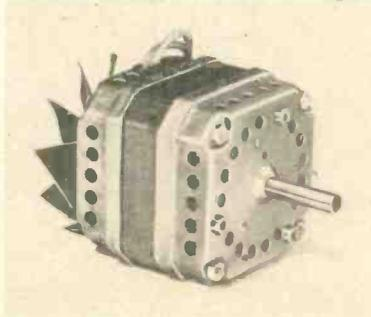
to withstand high temperature, yet is low-priced for application in mass-produced equipment. Built for continuous-duty operation, it is equipped with self-aligning oil-impregnated sleeve bearings and dynamically balanced rotor. Shaft diameter and length may be specified by the customer. Provision for two-speed operation is available on order. Complete information may be obtained from Electro Engineering Products Company, Inc., 609 W. Lake St., Chicago 6, Ill.
