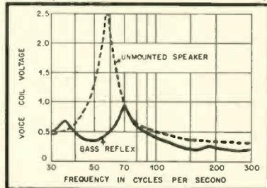
Fig. 10. These two curves show the results of the final bass-reflex enclosure.
