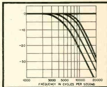
Fig. 8. Curves of low-pass filter action.
