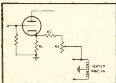
Fig. 15—15. Circuit for cancelling line-frequency hum. A capacitor in series with  $R_2$  can be used for corrective phase shift to bring the phase of the cancelling voltage opposite to that of the voltage being cancelled.
