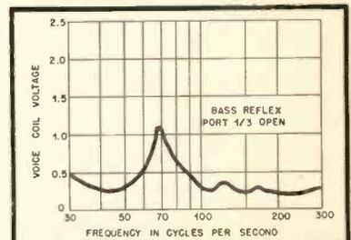
Fig. 6. Impedance curve with port area reduced to 24 square inches.
