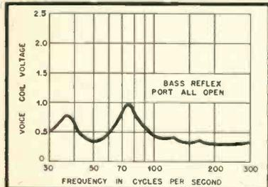
Fig. 8. Using the entire port area produced this impedance characteristic.
