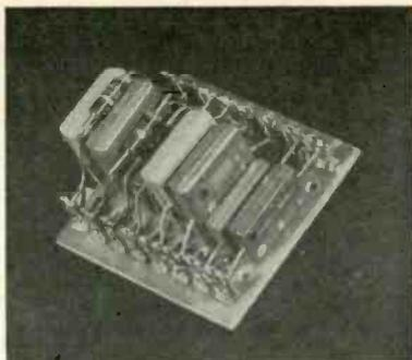
Fig. 7. Mounting of the components for the low-pass filter circuit. The input impedance-adjusting resistors  $R_{21}$  to  $R_{26}$  are mounted on the switch.
