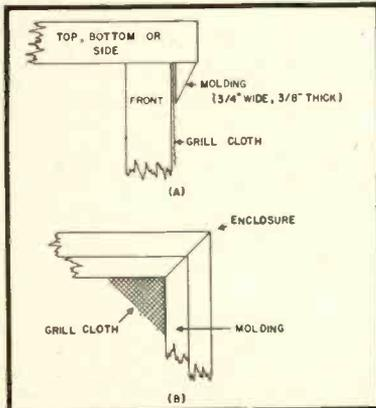
Fig. 4. Side view (A) and front view (B) show how the grill cloth was attached to give a professional appearance.
