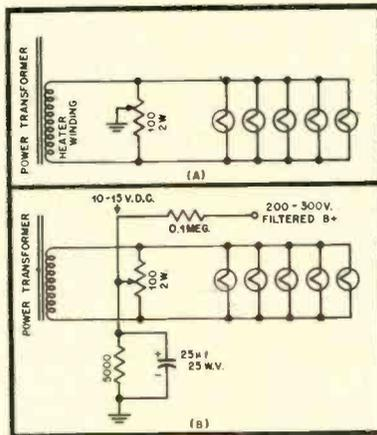
Fig. 15-11. A—Effective circuit for reducing hum resulting from a.c.-operated heaters. B—Elaboration of method shown in A, including positive bias on heater to prevent heater-to-cathode emission.
