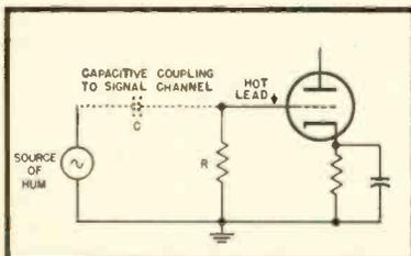
Fig. 15-7. Voltage divider formed by coupling path between the grid and hum source as upper arm, and grid-to-ground impedance as lower arm. The lower the relative value of  $R$ , the less the hum.
