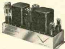
Frequency Response: 10 to 100,000 cycles  $\pm 1$ db. Power Response: 20 to 20,000 cycles  $\pm .25$ db. Intermodulation Distortion is less than .15%, and Harmonic Distortion less than .1%, at 15 watts. Class A-1 operation. Power supply is self-contained, with outlet for furnishing power to a preamp unit. Uses KT-66 output tubes.
