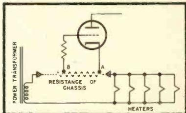
Fig. 15-12. Introduction of hum voltage between grid and cathode due to flow of a.c. return current through chassis.
