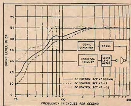
Fig. 6. Curves showing the effect of amplifier  $DF$  on distortion generated by loudspeaker system. 5% harmonic distortion contours are shown. (NORM.  $DF$  is equal to  $+30$ .)
