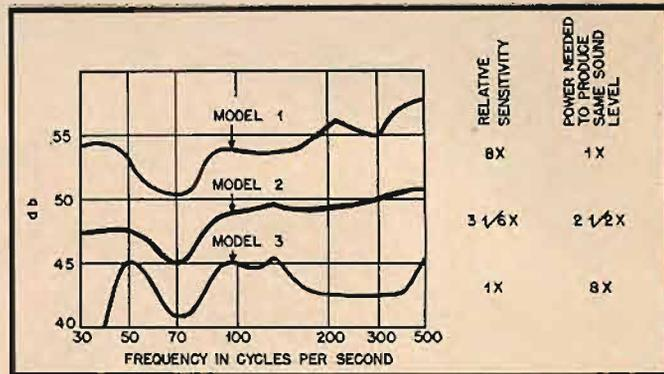
however, permit more space to be available in the voice coil gap which increases the power handling capacity of the loudspeaker. Therefore, to be able to estimate the relative conversion efficiency of a loudspeaker it is more important to know the number of gauss units in its voice coil gap than to know the size of the magnet being used with it.
