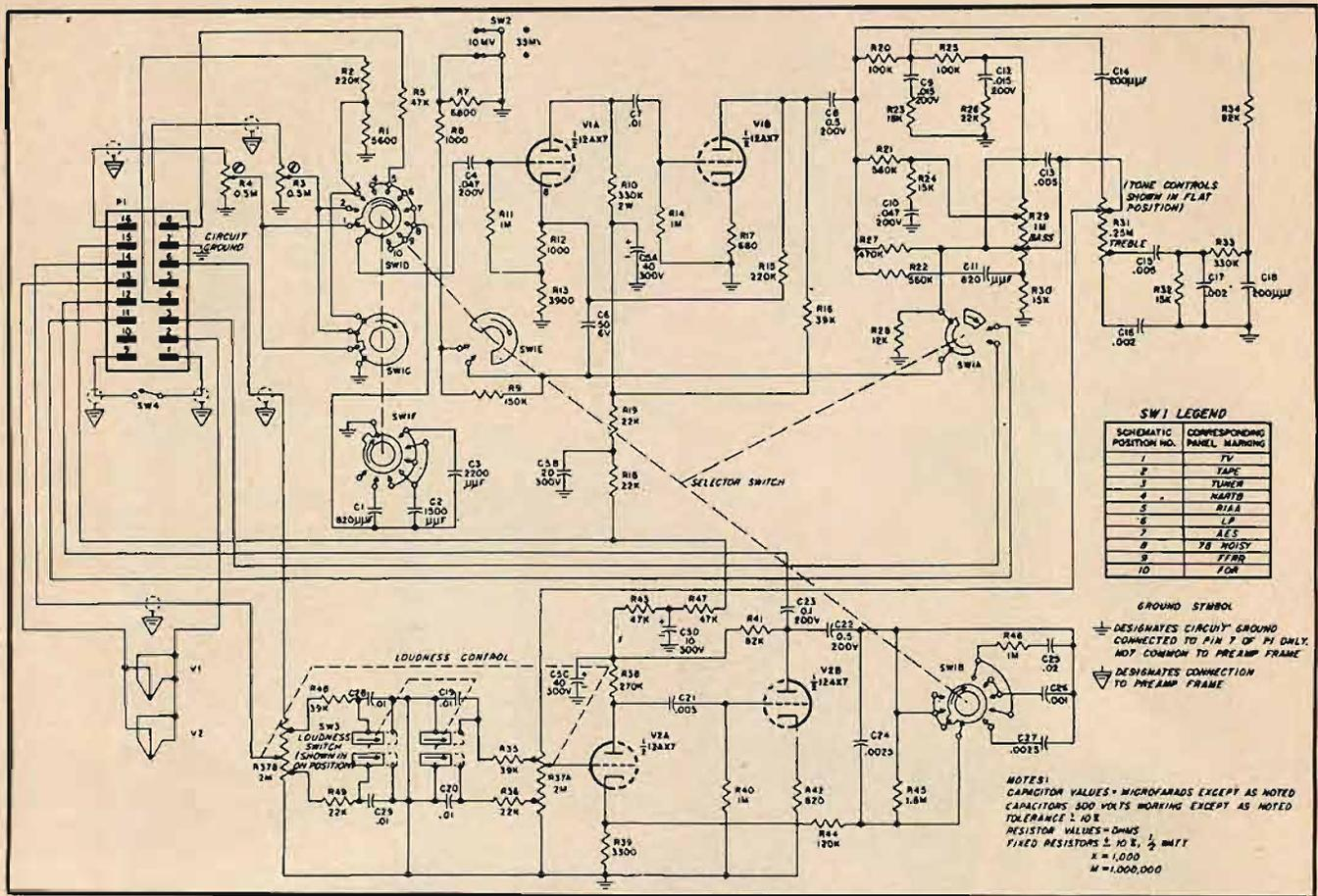
Fig. 3. Complete schematic of the Horizon 5 preamplifier.
