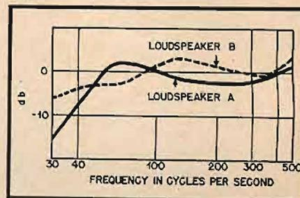
Fig. 3. Same loudspeakers as in Fig. 2 but plotted for equal output at 350 cps. Note difference such a plotting would cause.
