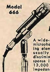
A wide-range, unidirectional microphone with a single moving element and featuring unusually high front-to-back discrimination. Frequency response is uniform from 50 to 13,000 cycles. The output impedance is 50 ohms with internal provision for easily adjusting to 150 or 250 ohms. Output is —57 db (Ref. 0 db = 1mw/10 dynes/cm<sup>2</sup>).
