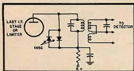
Fig. 1. Where the area is very noisy or the i.f. amplification is insufficient to saturate the limiters with the available signal, two crystal diodes make a very effective additional limiter.
