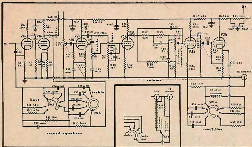
Fig. 4. Schematic of the Audio Console, with input switching eliminated to reduce size. The insert shows the switching for tape recorder feed and monitor output.
