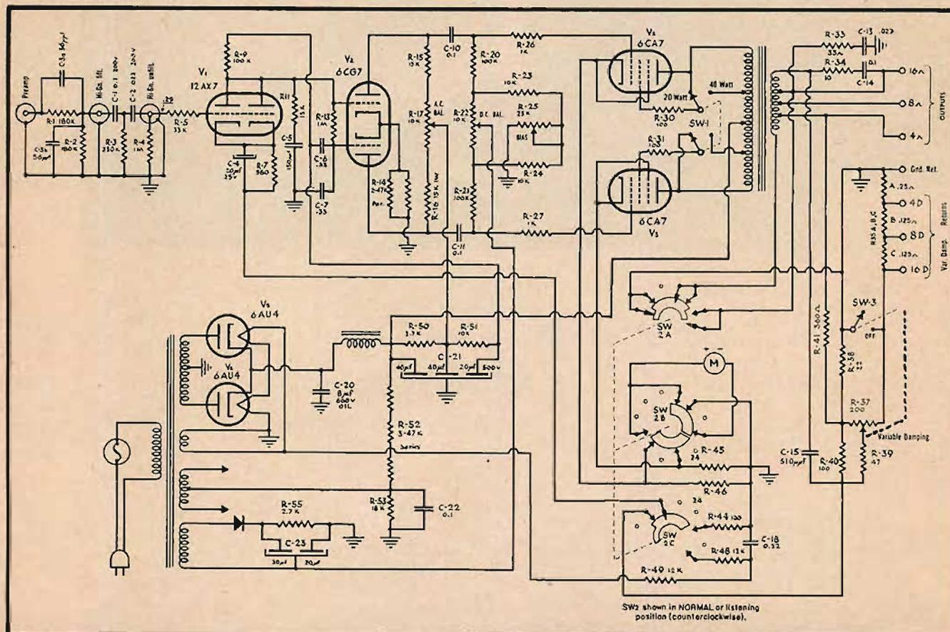
Fig. 5. Schematic of the Power Amplifier. The switch in the plate circuit of the output stage adjusts for maximum outputs of 40 or 20 watts, yet without changing gain.
