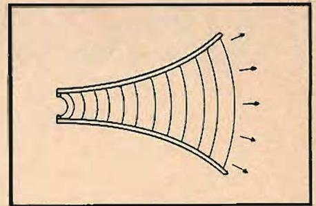
Fig. 10-6. Increase of effective radiating area of a small diaphragm at the throat of a horn to that of the mouth.
