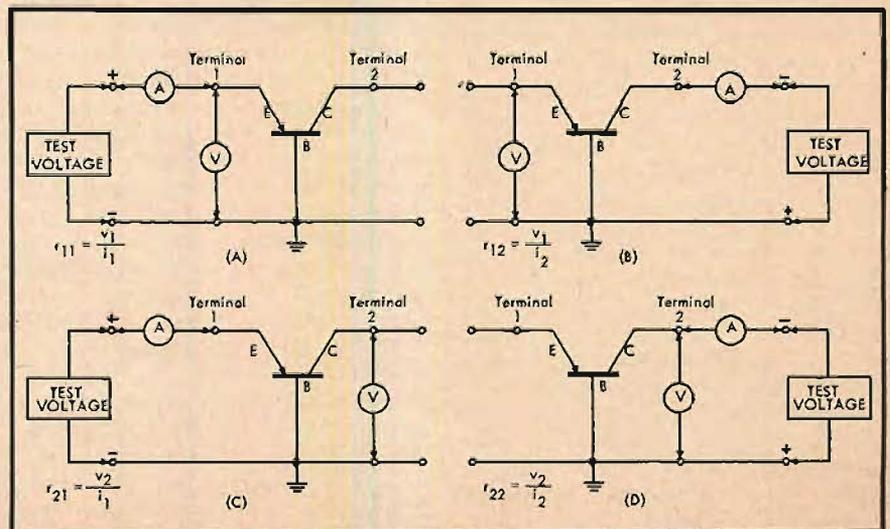
Fig. 2. Circuit connections for making static tests on a transistor.
