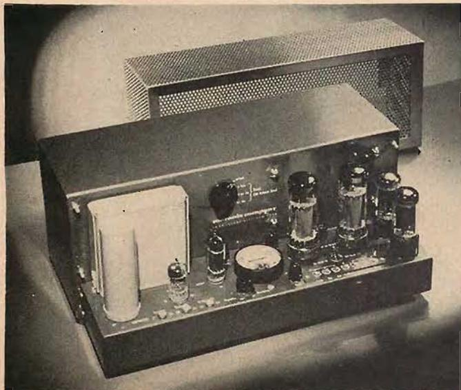
The two Marantz units—Fig. 2 (left) the 40-watt power amplifier with the perforated grille cover removed to show the meter and test switch as well as the adjustable controls. Fig. 3 (below) The Audio Console in its wood housing.
