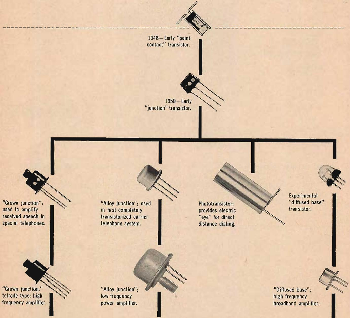
In 1948 Bell scientists announced their invention of the transistor—a tiny device able to amplify signals a hundred thousand times using a small fraction of the power of an electron tube.
