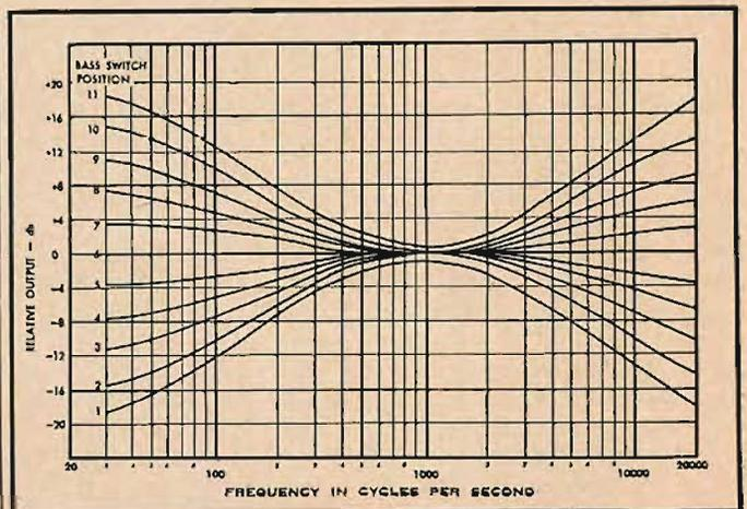
Fig. 2. Curves illustrate the wide range of slope control obtainable with the circuit of Fig. 2. The turnover frequencies are fixed.
