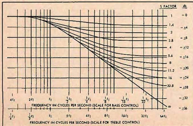
Fig. 9. These universal frequency curves are used in conjunction with the material in the text to calculate variations on the basic circuitry.
