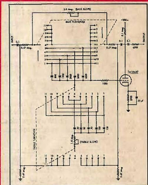
Two new types of tone controls—one with constant turnover and variable slope and one with both turnover and slope variable. See page 18.
