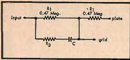
Fig. 6. Equivalent circuit for bass boost.
