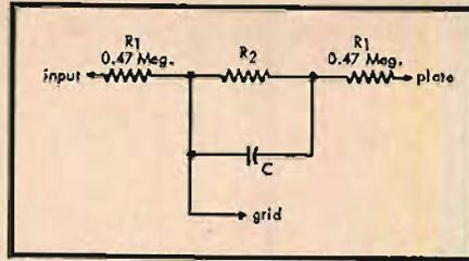
Fig. 7. Equivalent circuit for treble boost.
