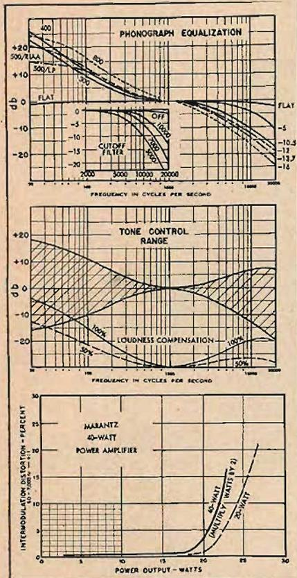
Fig. 1. Performance curves for the Marantz amplifier and Audio Console.
