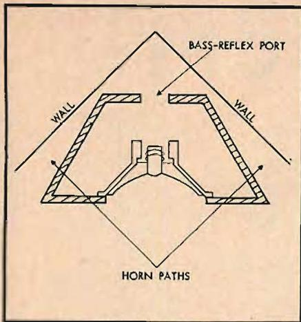
Fig. 10-8. Corner bass-reflex system with horn-loaded ports.
