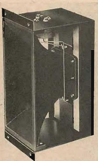
force, resulting in remarkably smooth response with freedom from resonance. The Kelly tweeter has a power capacity of better than 10 watts and input impedance is 15 ohms. Distributed in the United States by Ercona Corporation, Electronic Division, 551 Fifth Ave., New York, 17, N. Y. **B-1**
