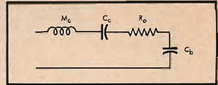
Fig. 6. Analogy of the closed box mounting.
