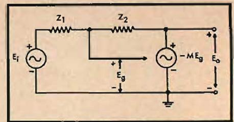
Fig. 5. Equivalent circuit of the tone control.
