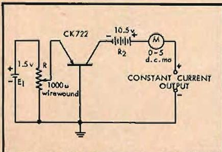
Fig. 5. Constant-current supply using a transistor.
