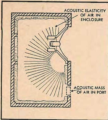
Fig. 10-5. Illustration of mass-elasticity system of bass-reflex Helmholtz resonator, and how it is coupled to the rear of the speaker cone.
