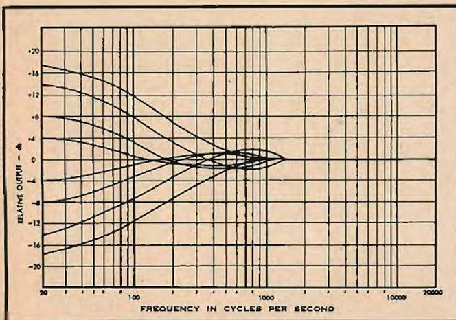
Fig. 1. These curves, taken from a Baxandall tone control, show the overshoot obtained with continuous controls.
