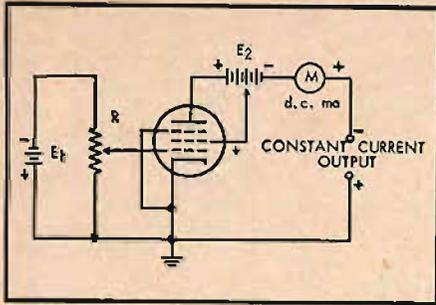
Fig. 4. Pentode vacuum-tube current regulator circuit.
