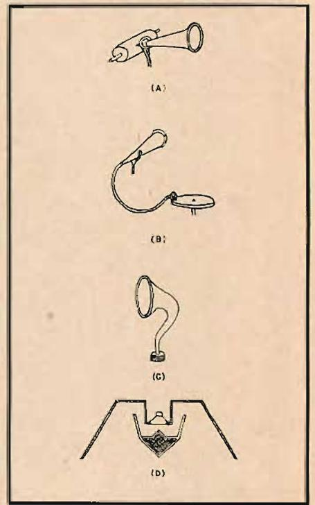
Fig. 10—7. Use of the horn as an acoustic coupler over the last seventy-five years (A) rigidly attached to phono pickup (Edison); (B) attached by flexible tubing (Berliner); (C) curved to conserve space; and (D) folded bass horn with direct-radiator type driver.
