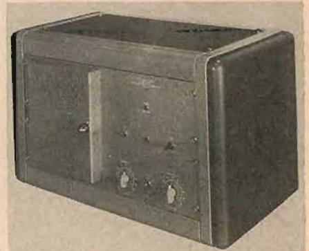
pensation is also provided. The new MagneLoop is designed to record and playback any message, musical program, or sound effect up to 60 minutes in length. Unusual recording and playback possibilities are created because speed control over an 8-to-1 ratio is now built into a single unit. The MagneLoop is available in single-, dual-, and triple-channel models. Complete technical specifications may be obtained by writing to Amplifier Corp. of America, 398 Broadway, New York 13, N. Y. **B-11**
