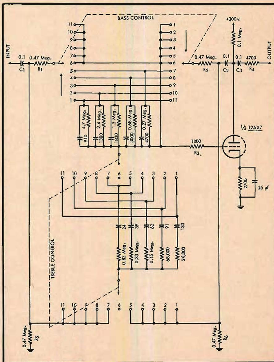
Fig. 3. The author's tone control. The switches allow optimum component-value selection for each condition and give good resettability.
