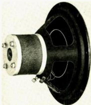
watts. It employs a single, sectioned cone and a mechanical crossover which provide excellent linearity throughout the audible range. Cloth suspension permits cone excursion of one-half inch. Distributed by Hartley Products Co., 521 E. 162nd St., New York 51, N. Y. **F-9**
