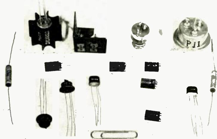
Fig. 1. Various transistors and components. The five Raytheon transistors have been adapted to fit into subminiature tube sockets, two of which are shown mounted in a universal power transformer mounting bracket, upper left. Two tantalum electrolytic capacitors are at extreme right and left positions. The rear row shows power transistors, the foreground common low-power transistors.
