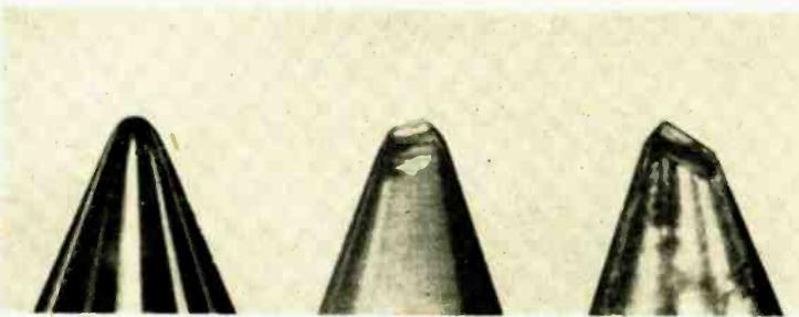
Fig. 4-6. One mil microgroove needles after 15 plays of a 12-inch Vinylite record, with 8 grams vertical tracking force. Left to right: diamond, sapphire, and osmium. (After Marcus.)
