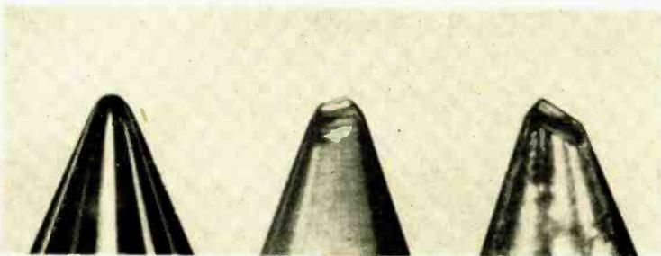
Fig. 4-6. One mil microgroove needles after 15 plays of a 12-inch Vinylite record, with 8 grams vertical tracking force. Left to right: diamond, sapphire, and osmium. (After Marcus).
