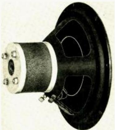
watts. It employs a single, sectioned cone and a mechanical crossover which provide excellent linearity throughout the audible range. Cloth suspension permits cone excursion of one-half inch. Distributed by Hartley Products Co., 521 E. 162nd St., New York 51, N. Y. **F-9**
