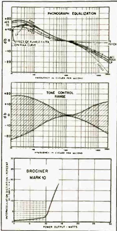
Fig. 1. Performance curves for the Brociner Mark 10 amplifier.
