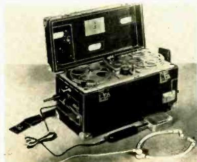
Fig. 14. The EMI broadcast-quality portable recorder.
