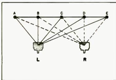
Fig. 9. Moving sound source recorded with two microphones.
