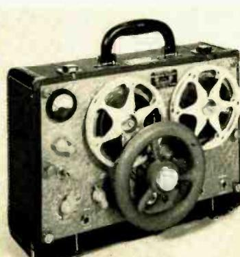
Fig. 15. Spring driven motor and battery powered amplifier are used in this Amplifier Corporation of America portable.
