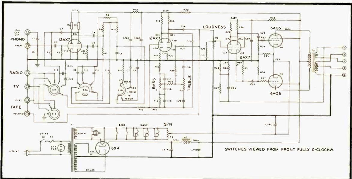
Fig. 2. Schematic of the Mark 10. Parts values are tabulated above.
