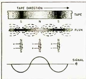
Fig. 1. Tape magnetization.
