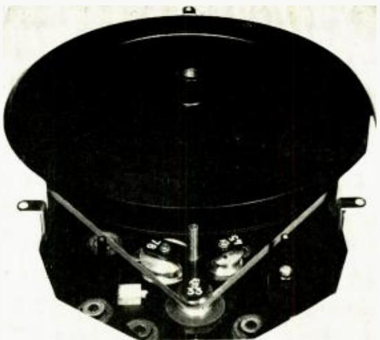
which way the plate is rotated, nor does it ever come up against a stop pin. The pulleys are always in line and the belt is handled with the greatest gentleness, so speed shifts have no effect on the life of the belt. It also makes possible a simple indicator of operating speed, since the speed can be indexed to the pulley in use and the pulley is visible through a transparent piece of lucite which forms part of the dress plate. The
