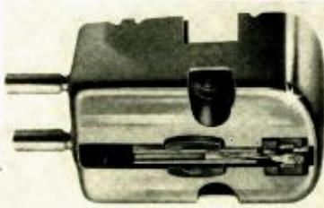
Fig. 4-2. The G. E. variable reluctance pickup. There are two gaps: when the iron in the stylus assembly is moved out of one gap it is simultaneously moved into the other.
