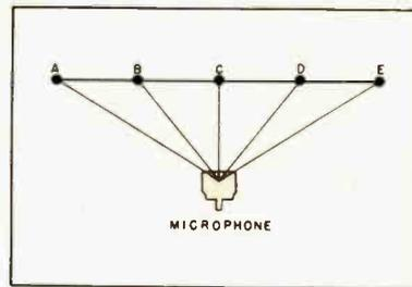
Fig. 7. Moving sound source recorded with one microphone.
