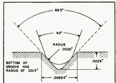
Fig. 4-5. A 3-mil stylus tip in the record groove. (After F. Langford Smith).
