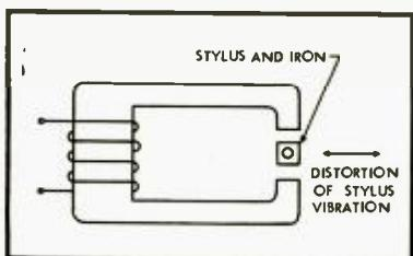
Fig. 4-1. Simplified diagram of the variable reluctance pickup.
