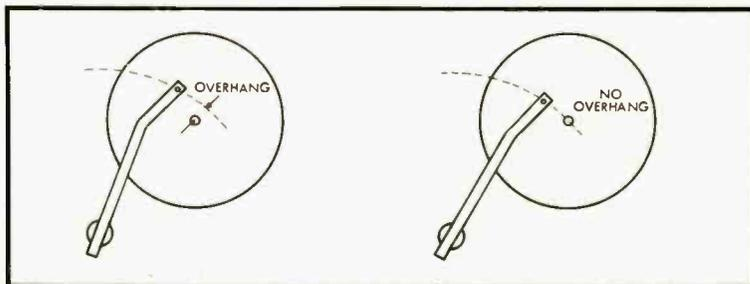
Fig. 4-7. Mounting position of the offset tone arm, showing overhang.
