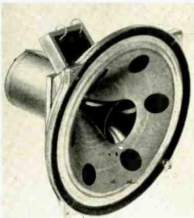
system weighing 11½ lbs., said by the maker to be the largest used commercially. A British Alcomax-3 high-efficiency magnet ring is used. Bass resonance is 35 cps and frequency response is 20 to 20,000 cps. Power rating is 15 watts undistorted. For complete information write Beam Instruments Corp., 350 Fifth Ave., New York 1, N. Y. **F-15**
