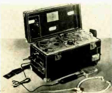
Fig. 14. The EMI broadcast-quality portable recorder.
