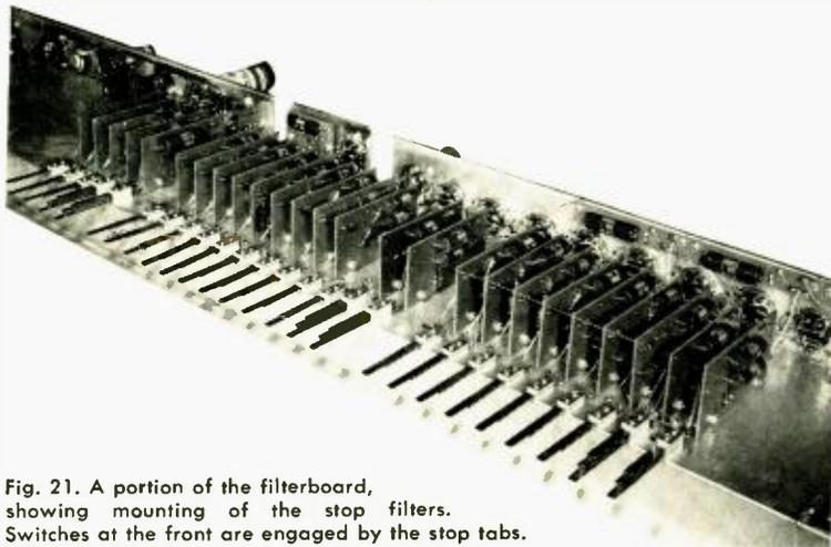
Fig. 21. A portion of the filterboard, showing mounting of the stop filters. Switches at the front are engaged by the stop tabs.
