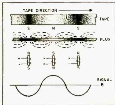
Fig. 1. Tape magnetization.
