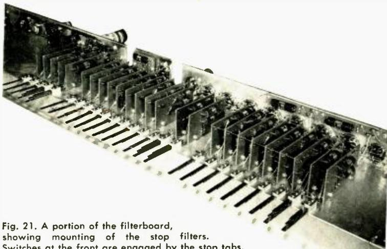
**Fig. 21.** A portion of the filterboard, showing mounting of the stop filters. Switches at the front are engaged by the stop tabs.
