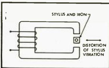
Fig. 4—1. Simplified diagram of the variable reluctance pickup.
