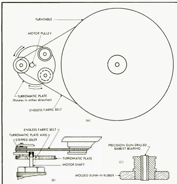
Fig. 2. Basic construction of the Turromatic turntable.
