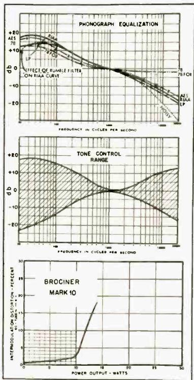
Fig. 1. Performance curves for the Brociner Mark 10 amplifier.
