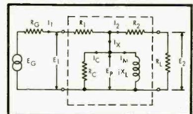
Fig. 1. Low-frequency equivalent circuit.
