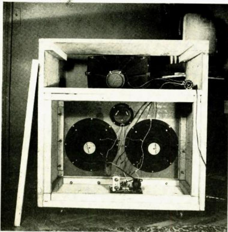
Fig. 6. Sub-vital statistic: Orderliness of cabled wire-up is recommended, but curl-paper wire-do is practised. T-pad for treble attenuation on top shelf, crossover on bottom. Note bolts holding baffle for woofer-mid-range speaker array.
