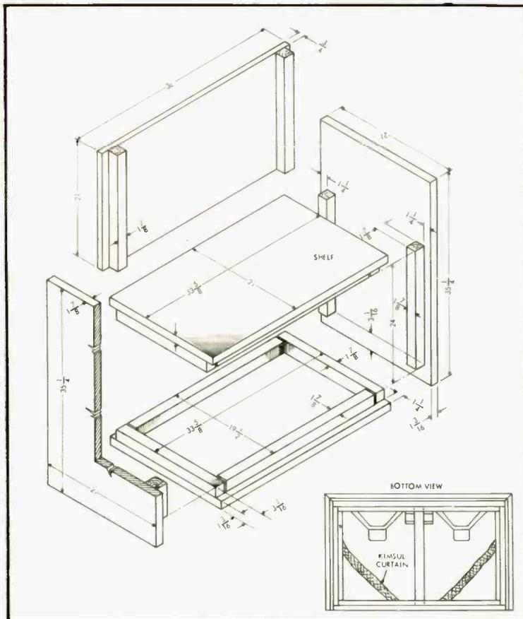
Fig. 3. Isometric view highlights simple building method. Heavy strips are secured to flats as in pallet or skid type construction. They reinforce corners when panels are fitted together. Inset shows placement of Kimsul curtains to eliminate internal standing waves.
