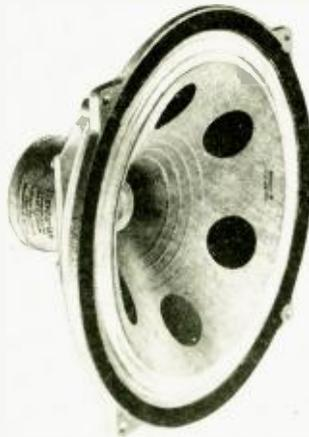
the new Model HP-1214 also incorporates six stabilizing discs of long-staple fibre which are impregnated into the front of the cone to improve mid-register response, particularly in the 1000-3000 cps range. Bass resonance is 39 cps and over-all frequency response is 25 to 14,000 cps. Power rating is 15 watts. Complete information will be supplied on request by Beam Instruments Corp., 350 Fifth Ave., New York 1, N. Y. **M-17**
