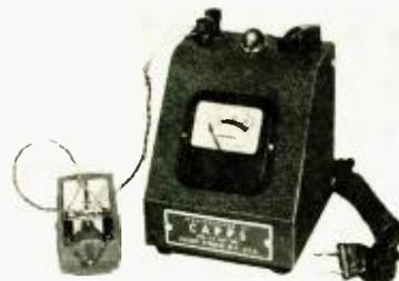
which fastens to the cutting head of the recorder, and a control panel. The terminal block features a unique quick-disconnect feature for ease in changing styli. The control panel includes stylus-heat control, pilot lamp, on-off switch, and a meter for precise heater-current indication. The unit operates from a standard 117-volt 60-cycle a.c. line. Capps and Company, Inc., 20 Addison Place, Valley Stream, N. Y. **M-12**
