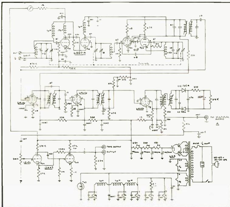
Fig. 6. Schematic of the Scott 311 FM Tuner.
