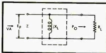
Fig. 3. Low-frequency impedance.
