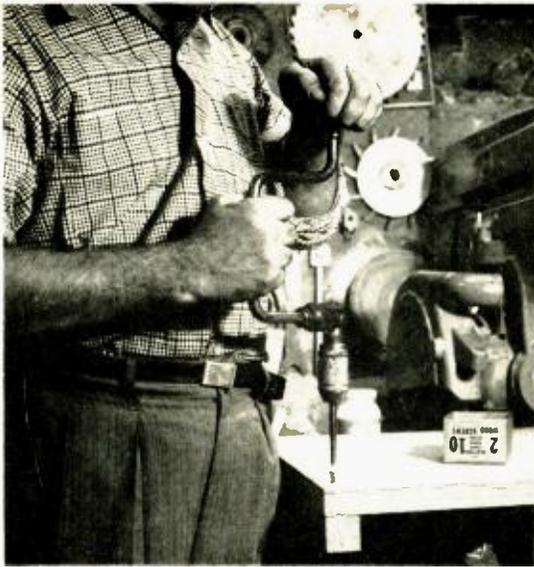
Fig. 8. Glue-screw procedure for firmness is feature of this speaker housing job. Owner uses brace-operated screwdriver for easier handling. Note bench is at comfortable working height just below bent elbow.
