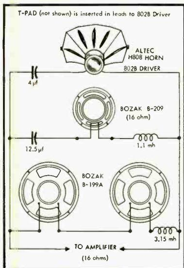
Fig. 11. Schematic of three-way speaker system shows wire-up and values of components. It is also plan of physical placement of speakers within and atop of infinite baffle.
