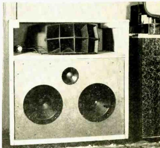
Fig. 5. Bozak assembly in place, with Altec-Lansing tweeter on shelf over. Non-resonant baffle is monolithic Chemstone fitted to framing over gasket, secured with bolts.
