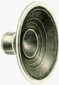
Philips of the Netherlands precision-built full resonance speakers are a special twin-cone design which provide energy transmission almost independent of frequency. Sound pressure within an angle of 90° does not vary by more than ± 6 db. in an ordinary room. Choice of coupling factor between high range and low range cones is responsible for the excellent spatial distribution of the acoustic energy even at highest frequencies.
