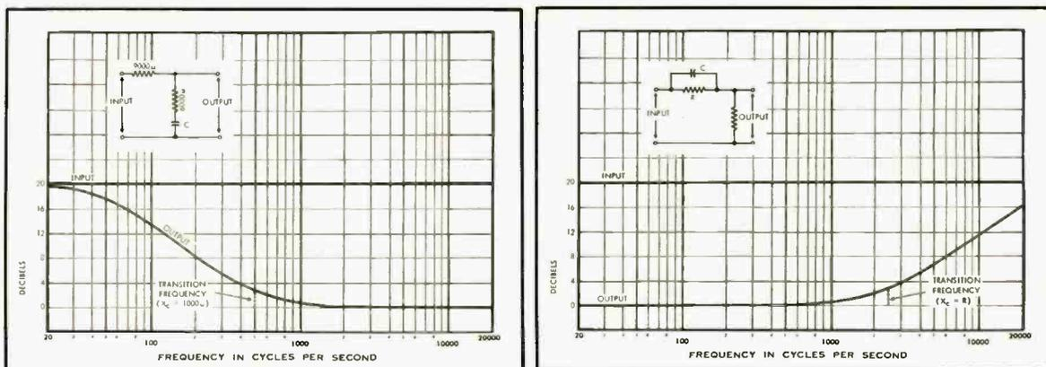
Fig. 6-2 (left). Resistor-capacitor voltage divider, and resulting bass boost. Fig. 6-3 (right). Treble boost circuit.
