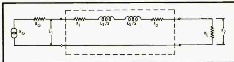
Fig. 4. High-frequency equivalent circuit.
