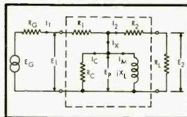
Fig. 1. Low-frequency equivalent circuit.
