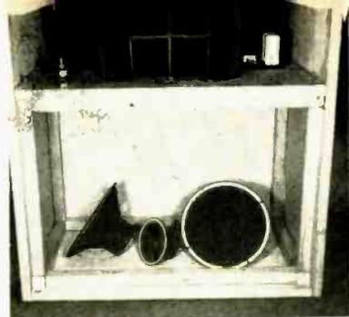
Fig. 2. Mock-up of installation in cabinet of extra-heavy veneer lumber. Lower compartment is full size Bozak enclosure; upper has been added to hold hold-over tweeter. T-pad on shelf, at left.
