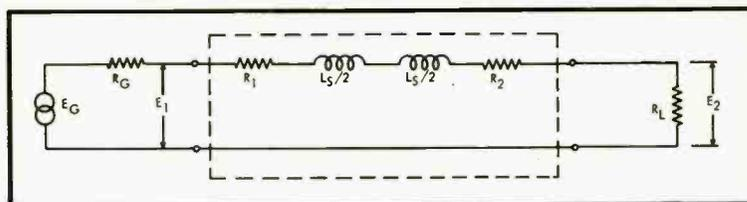
Fig. 4. High-frequency equivalent circuit.
