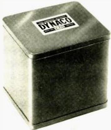
types. Undistorted power-handling capacity is 50 watts from 20 to 20,000 cps, and 100 watts from 30 to 15,000 cps. The transformer has excellent square-wave transmission at all audio frequencies, and its phase characteristics permit substantial feedback without inducing amplifier instability. Complete data on the Dynaco A-430 and circuitry for converting Williamson-type amplifiers to high power are available on request from Dyna Company, 5142 Master St., Philadelphia 31, Penn. **M-9**
