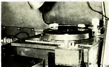
Fig. 4. Disc recorder for location cutting of test discs. Note remote control buttons for the tape recorders in mounting just to left of console.
