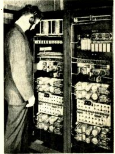
Fig. 4. The amplifiers and equalizers for the binaural system were adapted for use at the Century of Progress Exposition by L. B. Cooke.
