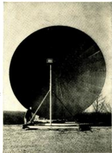
Experimental antenna used in early over-the-horizon UHF radio transmission research. Research extended transmission from 30 miles line-of-sight to 200 miles.
