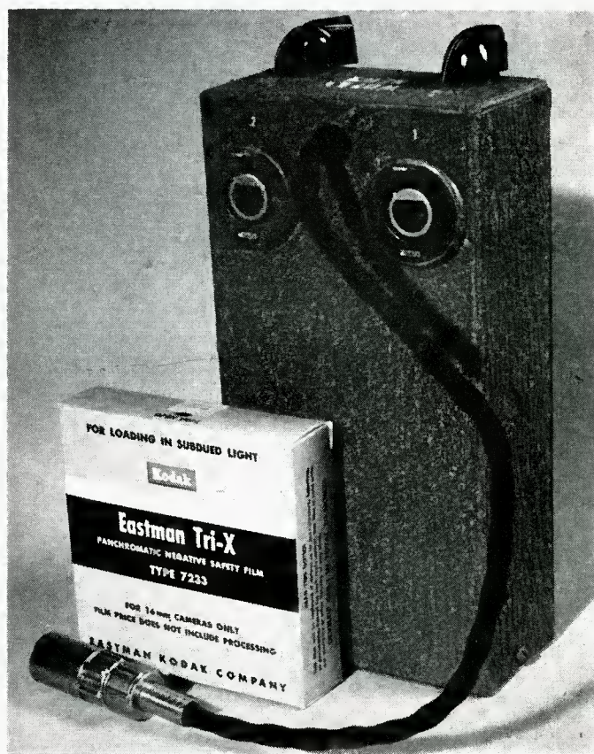
Fig. 1. External view of the two-channel sound-camera mixer unit—completely self contained, and suitable for employing two microphone inputs with a recording amplifier with only a single input.
