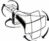
Horn bell rotates full 360° on its axis, while the "U" mtg. bracket provides better than 180° vertical and 360° horizontal adjustment of projector positioning. Thus, sound can be distributed in any direction regardless of projector location.
