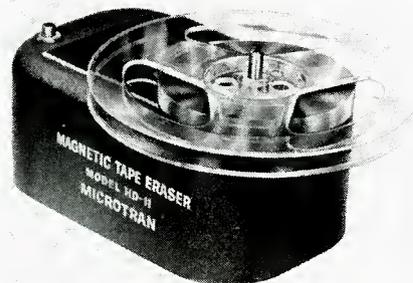
dle mounting of the reel to be erased permits rapid, thorough coverage. The device is useable with all standard tape reels from five to ten inches in diameter. It may also be used for demagnetizing record-playback heads, small tools and other metal objects. Supplied with baked enamel finish. Dimensions are 3" x 5" x 8" and weight is 8½ lbs. Manufactured by Microtran Company, Inc., 145 E. Mineola Ave., Valley Stream, N. Y. **J-11**
