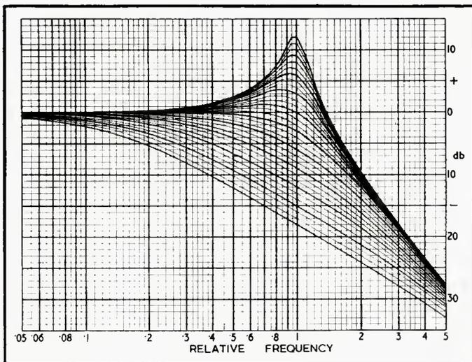
Fig. 12. The possible response curves for the network of Fig. 10. The chart of Fig. 11 identifies the required curve by the boost or attenuation at reference frequency (shown here as 1), which is  $f_0$  of equation (19).
