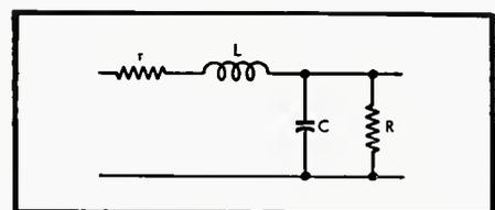
Fig. 10. Basic network for interstage high-frequency peaking roll-off.
