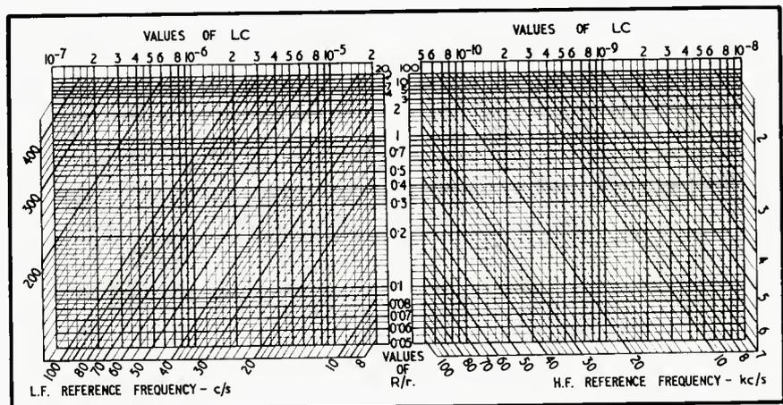
Fig. 13. Charts for giving the value of reference frequency  $f_0$ . The right hand chart applies to high-frequency peaking networks as at Fig. 10. The left part applies to low-frequency peaking networks as at Fig. 19, and the charts of Figs. 11 and 12 can also be applied for this, by taking reciprocal value of relative frequency (Fig. 12).
