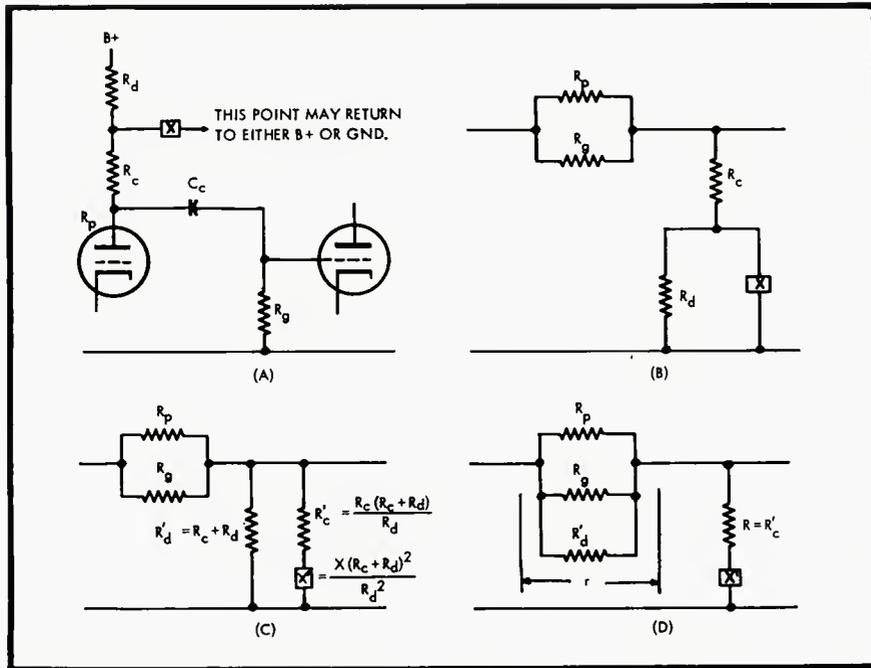
Fig. 17. An alternative practical circuit that also reduces to the same basic networks, (B) in Fig. 1 or (B) or (D) in Fig. 7. Notice in this case the conversion between (b) and (c) from  $R_c, R_d$  and  $X$  to  $R'_c, R'_d$  and  $X'$ .
