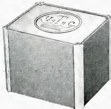
and 16 ohms. The LS-65 transformer is a similar unit with 60-watt rating, designed for use with Type 6550 tubes. Both transformers are furnished with a recommended circuit which provides maximum fidelity and stability. **J-8**
