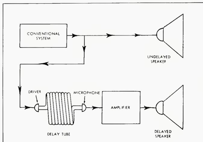
Fig. 3. Function diagram of the "Xophonic" reproducer.
