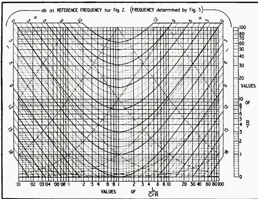
Fig. 11. Chart for determining the response shaping for known values of  $L$ ,  $C$ ,  $r$ , and  $R$  in the network of Fig. 10, and for estimating the effect of varying values. The dotted lines show typical paths represented by changing just  $r$  or  $R$  with the other values held constant.
