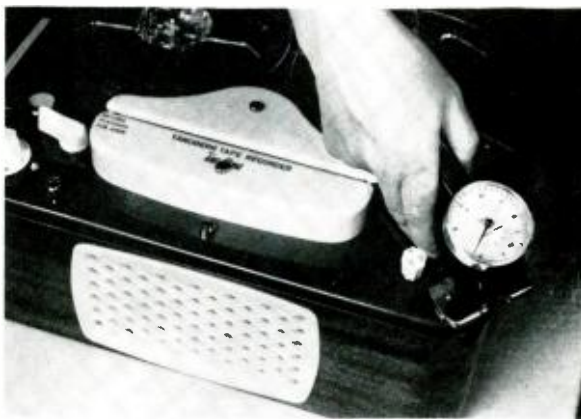
Fig. 3. Checking operating tension in a typical tape recorder. (Courtesy Reeves Equipment Corp.)
