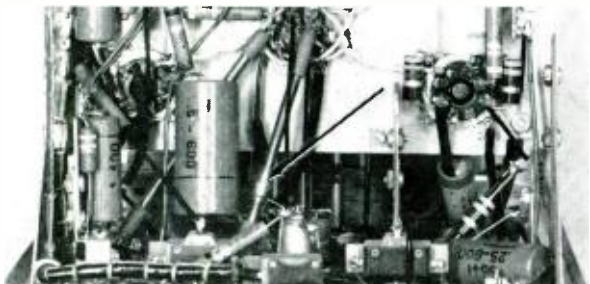
Spiral metal shield applied to oscilloscope lead. This gives very effective shielding, but at the cost of top a.f. response.
