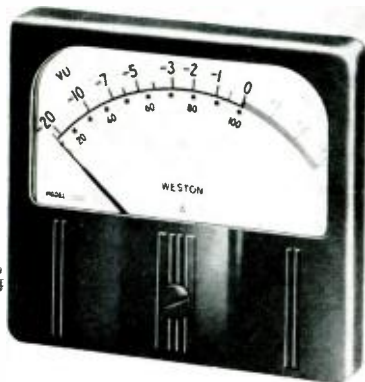
Fig. 3. Photo of a Weston VU meter with the "A" scale. (Courtesy Daystrom, Inc.)
