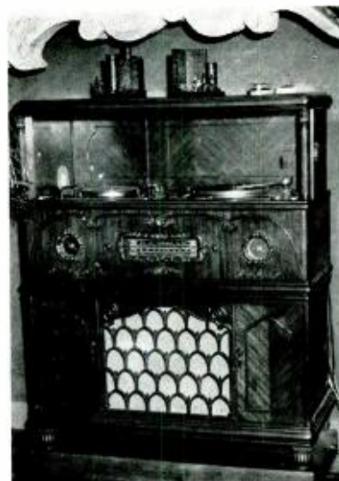
Records spin on high-quality transcription turntables in a glass-enclosed cabinet, which also houses an all-wave tuner and dual AM tuners. The latter pick up weekly stereo broadcasts by two Japanese government AM stations.
