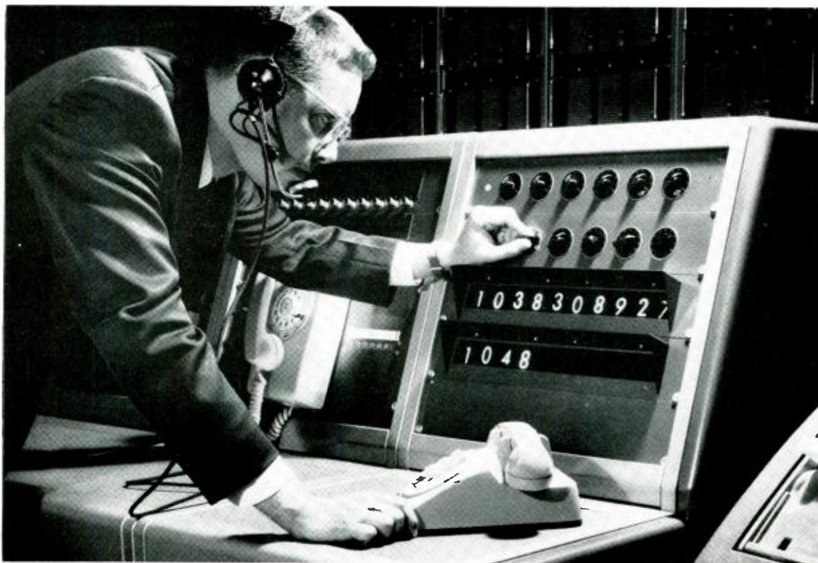
At monitoring console, designer H. D. Irvin watches performance of "Sibyl" during test of user-reaction to experimental telephones. A computer-like machine, Sibyl simulates the functions of future communications devices and records interplay between phones and users. Sibyl is named after the women oracles of ancient Greece.
