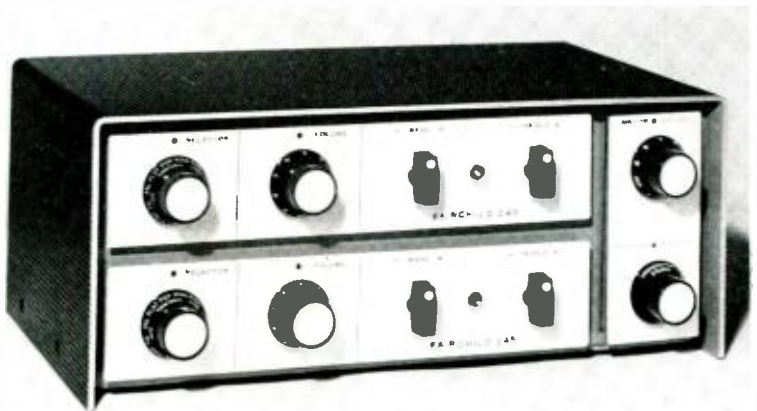
Fig. 6. Fairchild Model 248 Stereo Preamplifier-Equalizer, which combines two separate monophonic units with a stereo control unit to provide a complete console.
