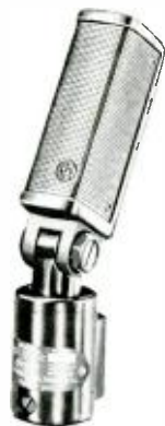
Fig. 5. Shure "Unitron" microphone—a ribbon type with a cardioid characteristic.
