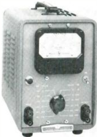
Fig. 6. A typical audio voltmeter. Although the scale is marked "Decibels," the reference level indicated on the meter is given as 1 mw/600 \omega . Observe that 0 on the db scale is directly under 0.775 volts on the rms voltage scale. The meter is in reality a dbm meter. (Courtesy Hewlett-Parkard Co.)
