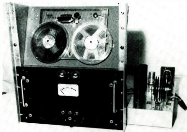
Fig. 6. The tape deck is attached to the amplifier by means of two "Tee" bars. Although the power supply is shown next to the amplifier it should be no closer than three feet when it is being used.
