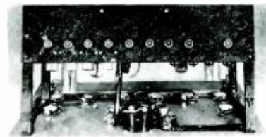
Fig. 13. Rear view of chassis showing audio chassis connectors, with output at left. Switches over four mike inputs at right are intended for input level matching.
