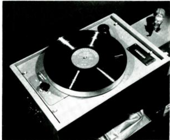
Fig. 2. Top view of turntable showing flush mounting of counter.
