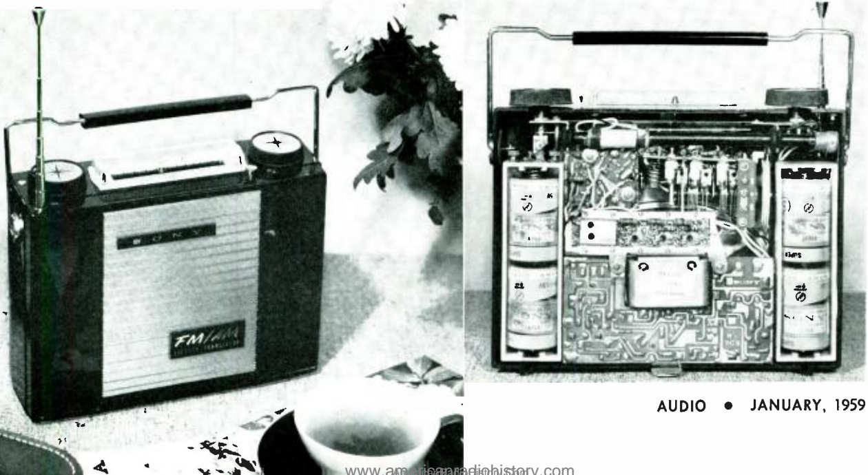
Fig. 1 (left). Sony TFM-151 AM/FM transistorized portable. Fig. 2 (right). Interior of 15-transistor receiver. Note speaker magnet frame projecting through opening in printed-circuit panel.
