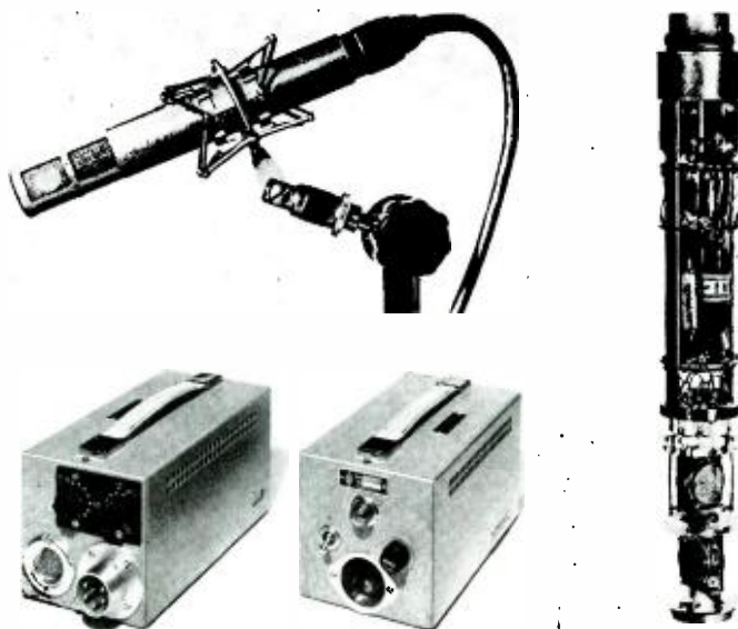
Fig. 11. (A) Internal and (B) external views of Telefunken SM-2 stereo condenser microphone and (C) power supply. (Courtesy Gotham Audio Sales Co. Inc.)
