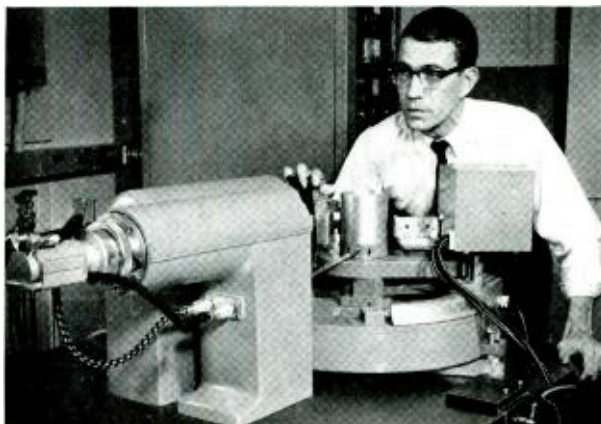
Chemist Jack Wright developed the use of this X-ray fluorescence machine for testing the concentration of preservatives in wood. Here he bombards a boring from a test telephone pole with X-rays.
