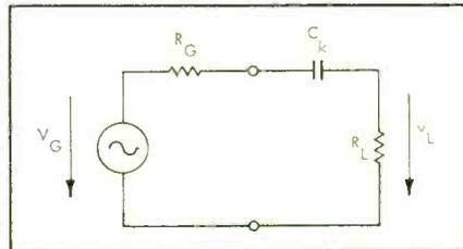
Fig. 15. Four-terminal network.
