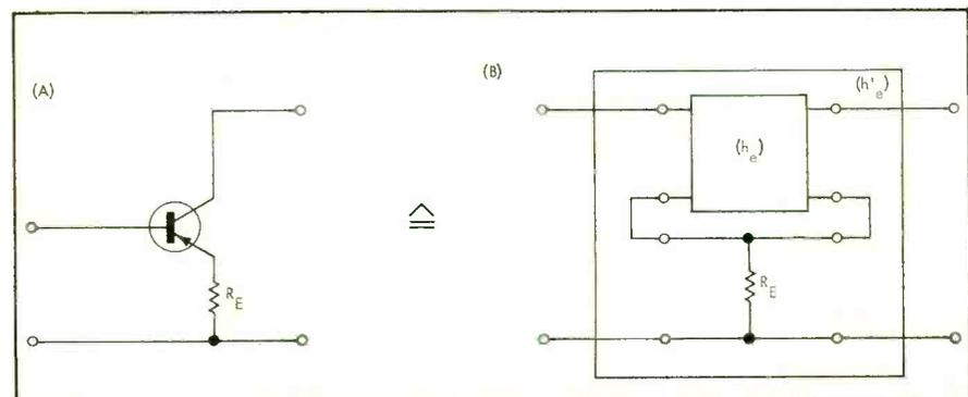
Fig. 16. Common emitter stage with series feedback: (A) a.c. equivalent network; (B) four terminal network representation.
