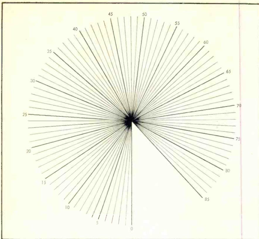
Fig. 3. Dial face for the tuner. A reproduction of this figure should be carefully prepared and applied to the tuner-oscillator panel. A hole should be made at the exact center for the shaft of  $R_1$ , and a large-diameter knob used with a sharp pointer.
