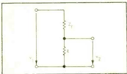
Fig. 22. Voltage-divider network.
