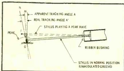
Fig. 7. Increase of vertical tracking angle by longitudinal elasticity of the rubber stylus mount.
