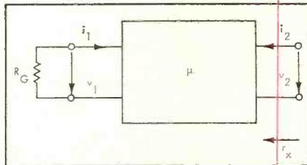
Fig. 20. Output resistance of amplifier without feedback.
