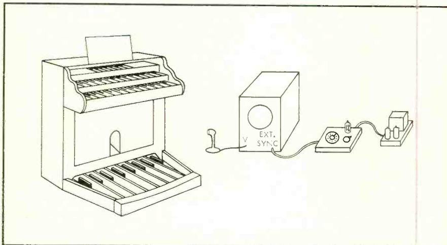
Fig. 1. Setup for the electronic tuning of musical instruments. A crystal microphone connected to the vertical input of the oscilloscope picks up a single tone from the organ. The scope is synchronized by the tuner-oscillator, which is powered by the regulated supply on the right.
