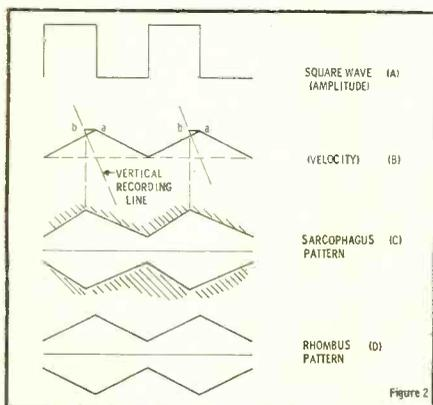
Fig. 2. (A) Square wave applied to the cutter amplifier. (B) Motion of recording stylus. (C) Sarcophagus pattern produced by slanted cut. (D) Rhombus pattern with 0-deg. modulation slant.
