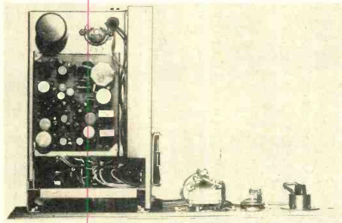
Fig. 2. Entire electronics and control chassis of Sony EM-1.
