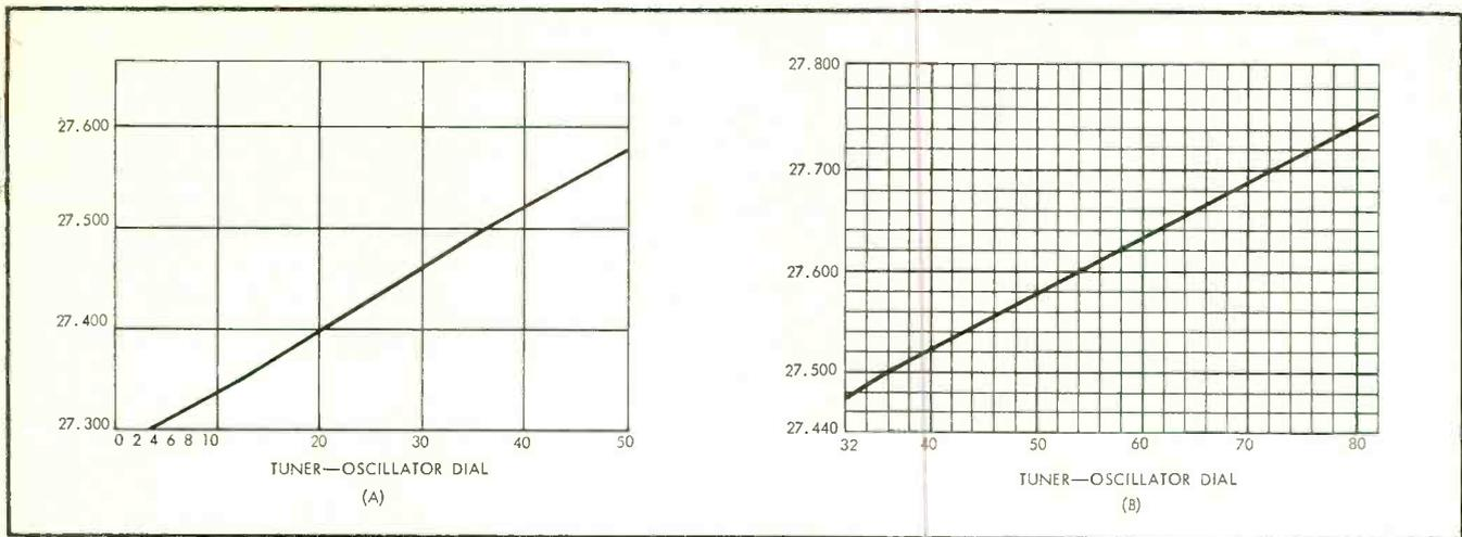
Fig. 6. Two sheets of 8-by-10-inch graph paper are used to plot the calibration curve for the tuner-oscillator dial. This expanded scale provides the definition required for accuracy to three decimal places at 27 cps.
