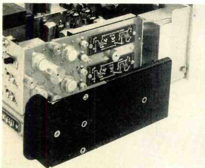
Fig. 5. Closeup of the transistorized stages of the "Astro." Input transistors, together with associated printed circuitry, are on the right; the driver transistors are mounted in a vertical line in the center; the four power transistors are at the left. The large metal spacers transmit heat to the large black heat sink (shown removed).
