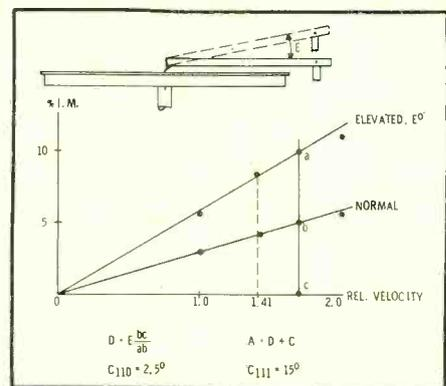
Fig. 8. Method for measurement of vertical tracking angle with STR-110 or STR-111 records.
