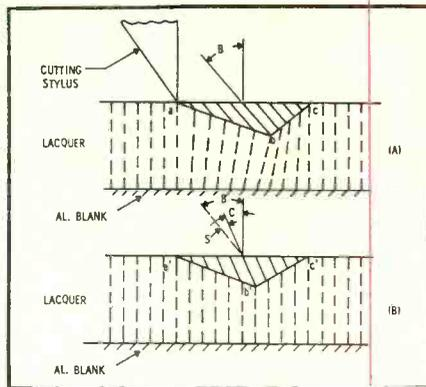
Fig. 3. Stressing of lacquer during cut. (A) Followed by springback after cut. (B) The resulting modulation  $a'-b'-c'$  is less slanted than the line of cutter motion  $a-b-c$ .
