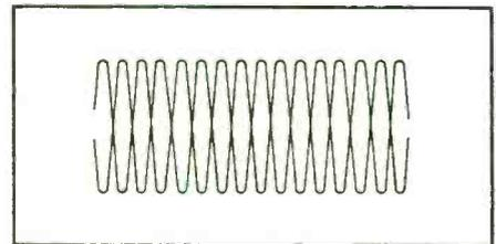
Fig. 8. Pattern obtained when D#5 is tuned at the dial setting for 27.656 cps. When tuned exactly, the starting points for the two traces at the left end of the pattern should stand still.
