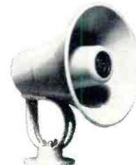
**SPECIFICATIONS:** Frequency Response 400-13,000 cps, Sound Pressure Level 119 db (at 4' on axis, 7.5 watts input, 2-4 kc), Power Handling Capacity 7.5 watts, Impedance 8 ohms, Dispersion 120°, Size 6 1/2" diameter x 6" deep, Weight 2 lbs.
