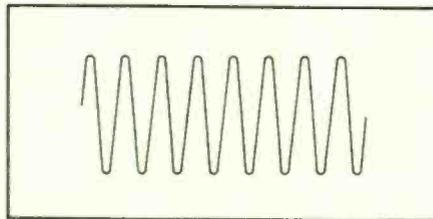
Fig. 5. Pattern obtained when scope is synchronized with the tuner-oscillator at 27.500 cps, and the organ A3 is tuned to 220 cps. In tuning organs, an 8' flute stop is used to obtain a sine-wave pattern.
