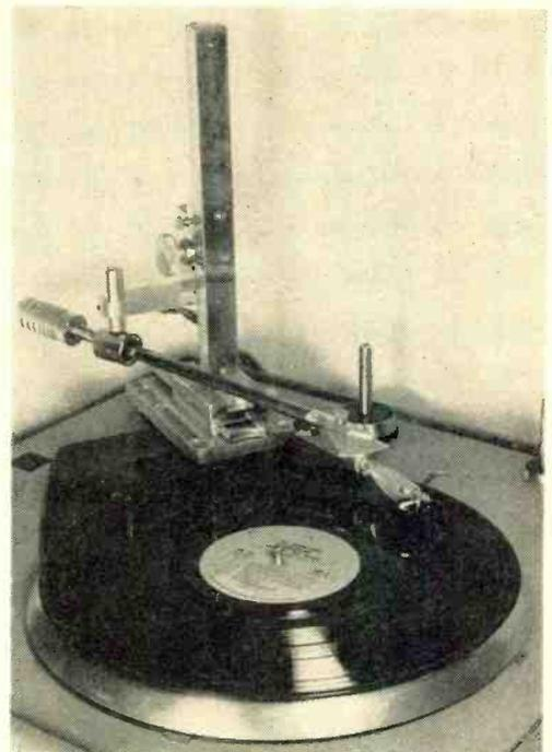
Fig. 6. Adjustable arm for measurement of modulation slant and pickup vertical tracking angles.
