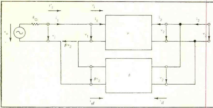
Fig. 19. Block Diagram of amplifier with negative voltage series feedback.
