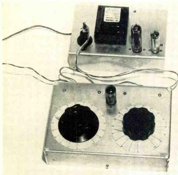
Fig. 7. Photograph of the tuner-oscillator and power supply.
