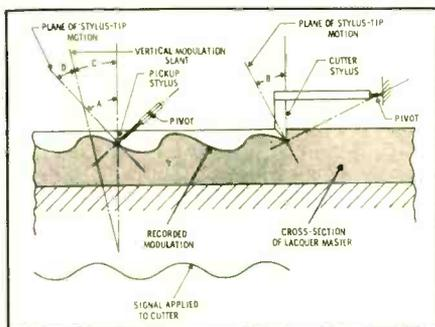
Fig. 1. Diagrammatic representation of vertical tracking angle, A, vertical recording angle, B, and vertical modulation slant, C. Because of lacquer springback, C is smaller than B.
