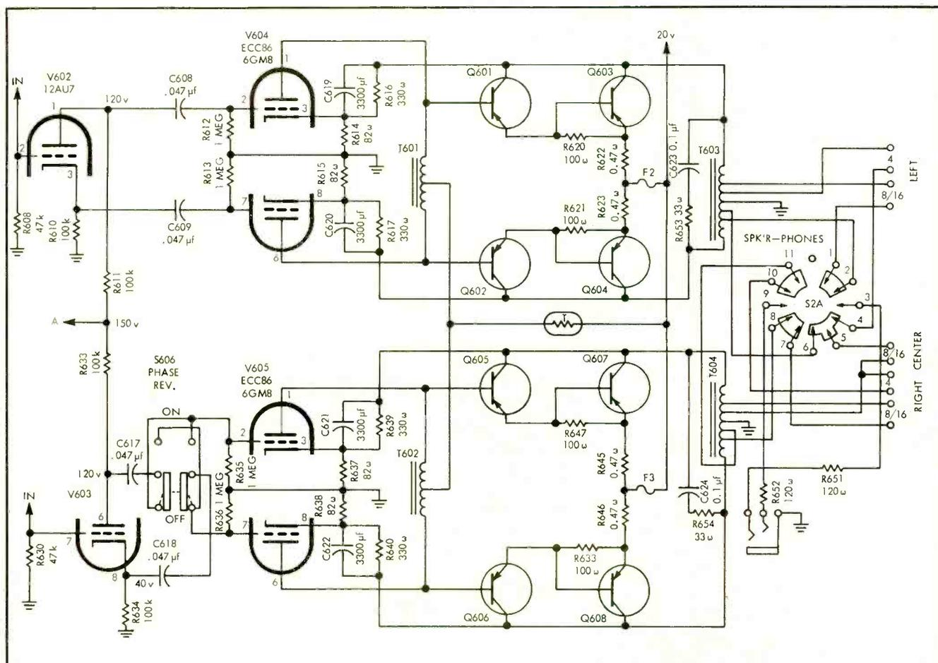
Fig. 4. Schematic of the output and driving stages of the "Astro."
