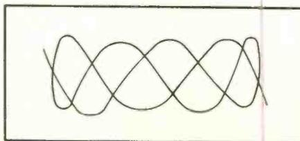
Fig. 4. Pattern obtained when the organ A is tuned to 220 cps and when a 60-cps signal from the a.c. line scans the scope horizontally. The identifying features of this pattern are the six central areas, each bounded by three sides.
