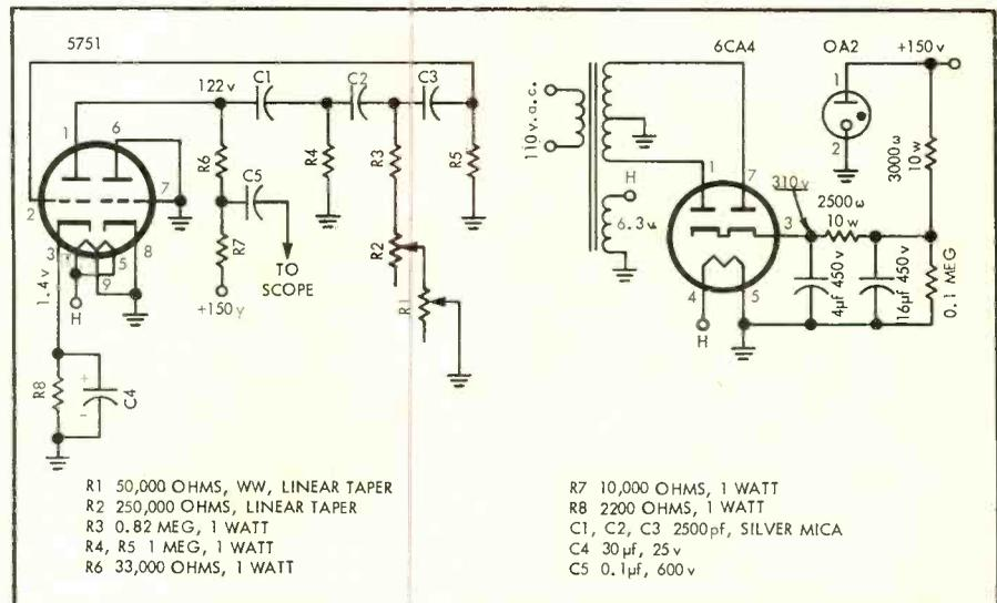
Fig. 2. Circuit of the tuner-oscillator and power supply. Oscillator stability is improved by the use of a premium-type 5751, by voltage regulation from the OA2, and by separation of the oscillator from the power-supply. This latter precaution minimizes temperature drift.
