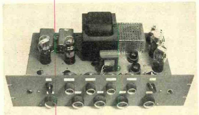
Fig. 4. Close-up view of thyatron amplifier chassis and control panel.
