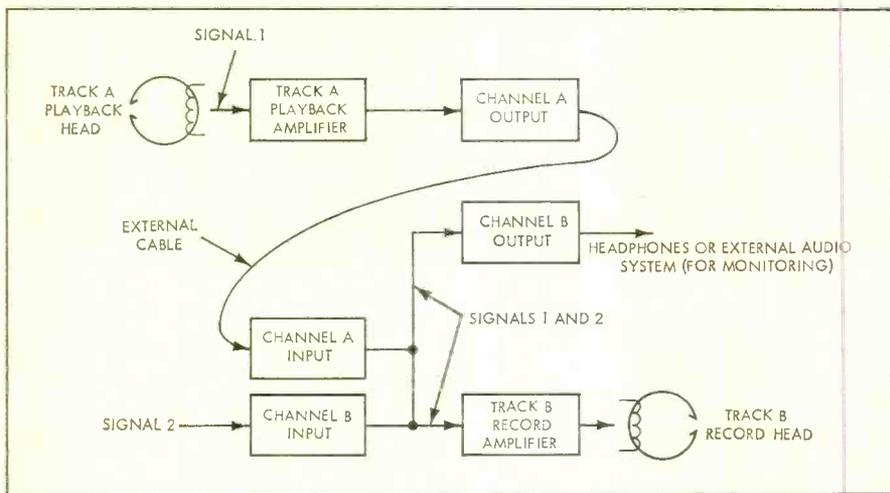
Fig. 2. Sound-on-sound recording with the Model 64.
