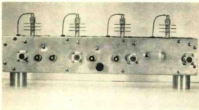
Fig. 3. Battery of silicon rectifiers and their heat sinks. Note use of screen grid caps as anode connectors.
