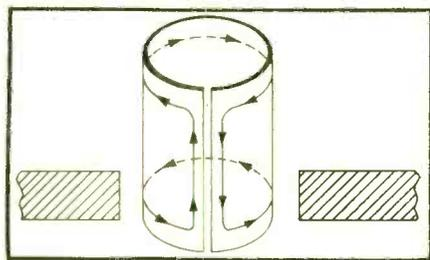
Fig. 4. Voice-coil former with the electrical circuit indicated.
