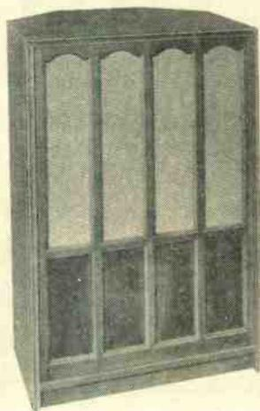
the Patrician 800 can be placed in almost any room location without seriously hampering its performance. It has a frequency response of 20 to 35,000 cps and a program power handling capacity of 100 watts. Above 100 cps a 12-inch mid-bass speaker is used and above 800 cps treble is handled by the new T250 treble driver. A T350 driver, operating from 3500 cps to beyond audibility, handles the "super-tweeter" frequencies. Electro-Voice, Inc., Buchanan, Mich. **C-4**
