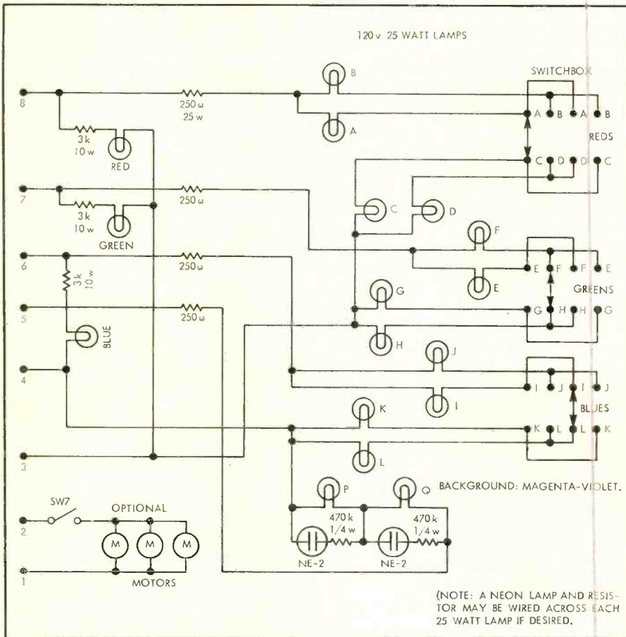
Fig. 9. Alternate lamp circuit used in this model.
