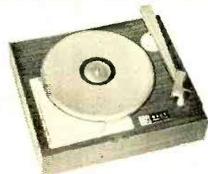
An easy-to-assemble stereo LP turntable kit of professional quality and performance. Rumble better than 50 DB down . . . flutter 0.08% . . . wow 0.2%. Polyurethane drive belt; hysteresis-synchronous drive motor.
