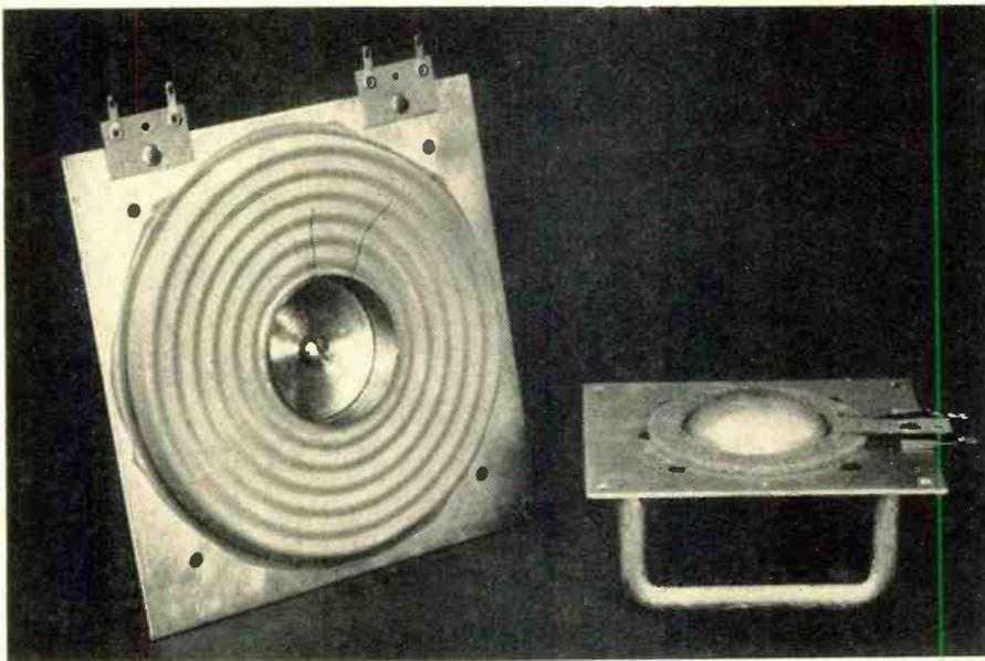
Fig. 2. The hemispherical-dome tweeter (on the right) and the spider and voice-coil assembly of the woofer. Note the metal former.
