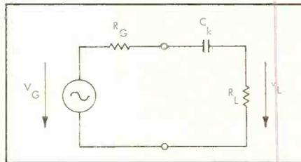
Fig. 25. Capacitive coupling.
