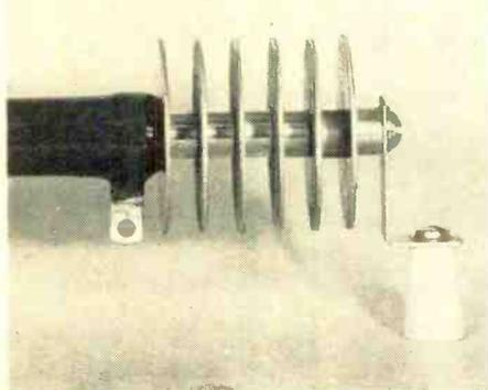
Fig. 4. Experimental cooling assembly.
