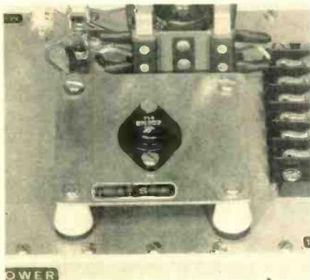
Fig. 1. "Direct coupled" heat sink.
