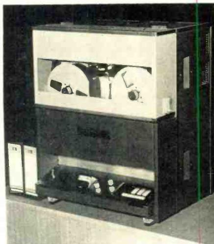
New Sony video recorder is not much larger than two audio tape recorders.
