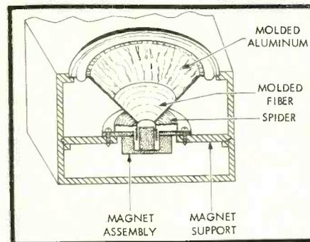
Fig. 3. Mounting of the woofer cone and magnet assembly in the enclosure.
