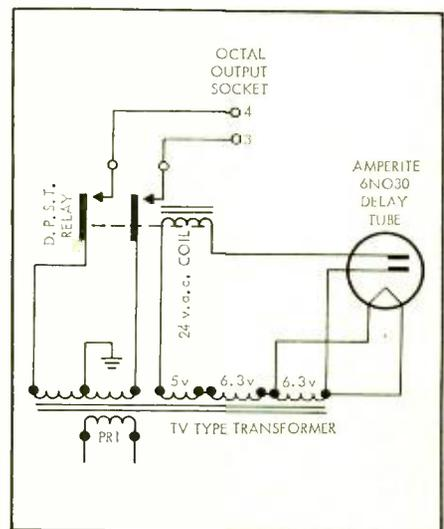
Fig. 8. Thermal-tube method of applying delayed plate voltages.
