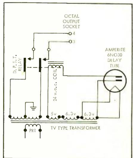
Fig. 8. Thermal-tube method of applying delayed plate voltages.
