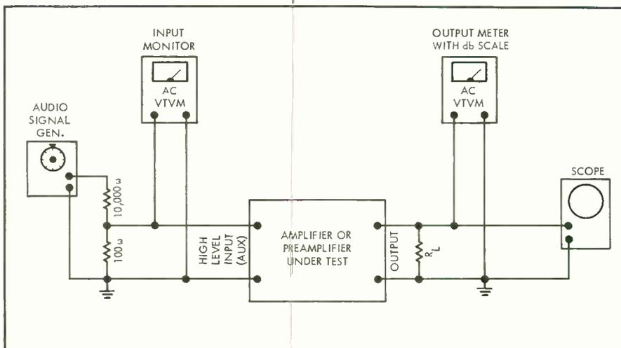
Fig. 1. Test circuit.  $R_L$  is equal to the characteristic load resistance at the output transformer of the power amplifier. Do not use a resistor when testing a preamplifier.
