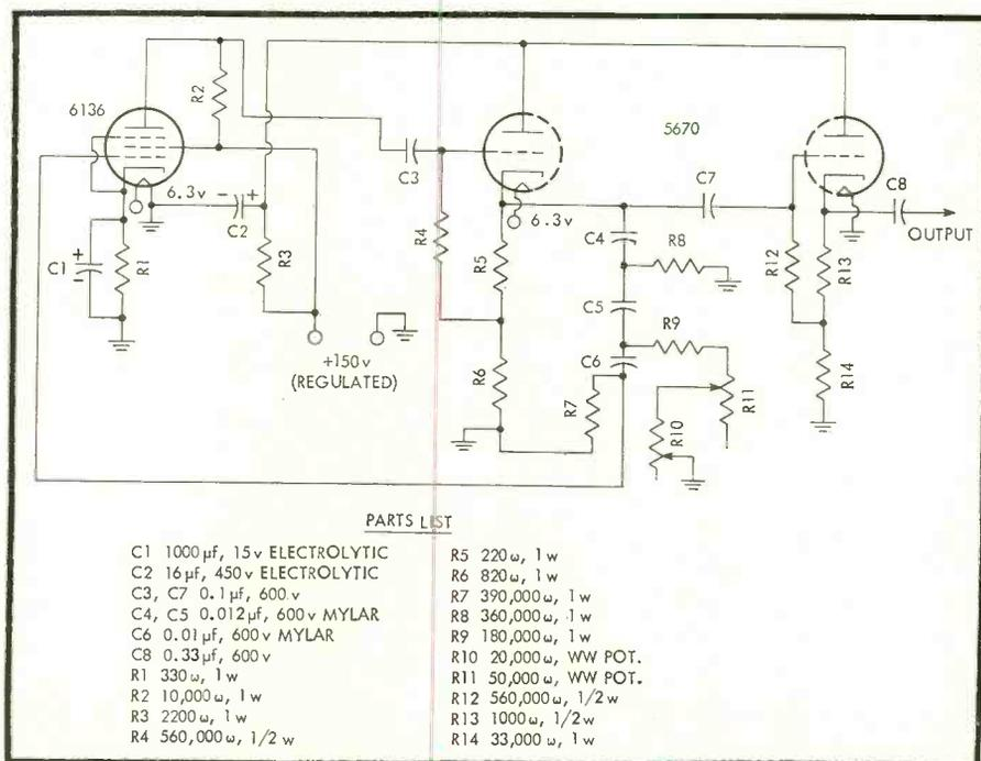
Fig. 1. Circuit diagram for the 20-cps electronic tuner. The location of the components is not critical, but R<sub>7</sub> through R<sub>11</sub> and C<sub>4</sub> through C<sub>6</sub> should be placed where heat from the tubes is not excessive.
