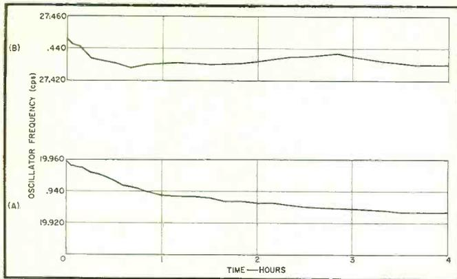
Fig. 4. (A) shows that the 20-cps tuner changes frequency from the time it is turned on until it approaches temperature equilibrium; (B) shows the behavior of the 27.5-cps oscillator. The rate of frequency drift was required to determine tuning accuracy.
