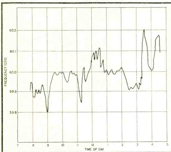
Fig. 5 (left). Measured frequency variation of a 60-cps line; points on the curve represent average values for one-minute intervals. Frequency variation was less than 0.1 cps for 75 per cent of the time, and less than 0.05 cps for 50 per cent of the time.
