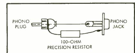
Fig. 6. Connector for measuring head current.
