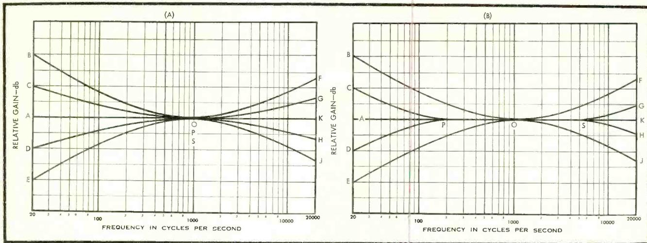
Fig. 2. Typical tone control curves resulting from: (A) A losser circuit, and (B) a Baxendall circuit. A-O-K is the "flat" line, B-O-K is maximum bass boost, E-O-K is maximum bass cut, A-O-F is maximum treble boost, and A-O-J is maximum treble cut. Other curves represent intermediate settings of the tone controls.
