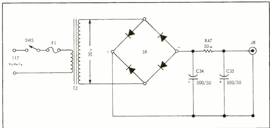
Fig. 5. Schematic of power supply.
