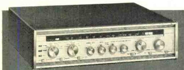
If you want a component that combines tuner and 80-watt stereo amplifier in one compact chassis . . . see the new S-8000 III FM Stereo MX Receiver. Has zero-centered professional tuning meter and Stereo Indicator Light.
