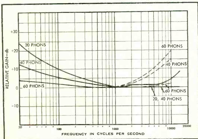
Fig. 10. Compensation for Robinson-Dadson curves. 70 phons is standard playback level (—age 20, --- age 60).
