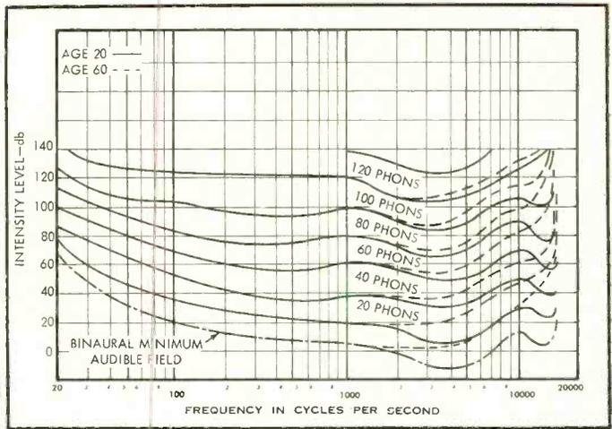
Fig. 8 (left). Compensation for Fletcher-Munson curves, 70 phons is standard playback level. Fig. 9 (right). Equal-loudness contours (Robinson and Dadson).
