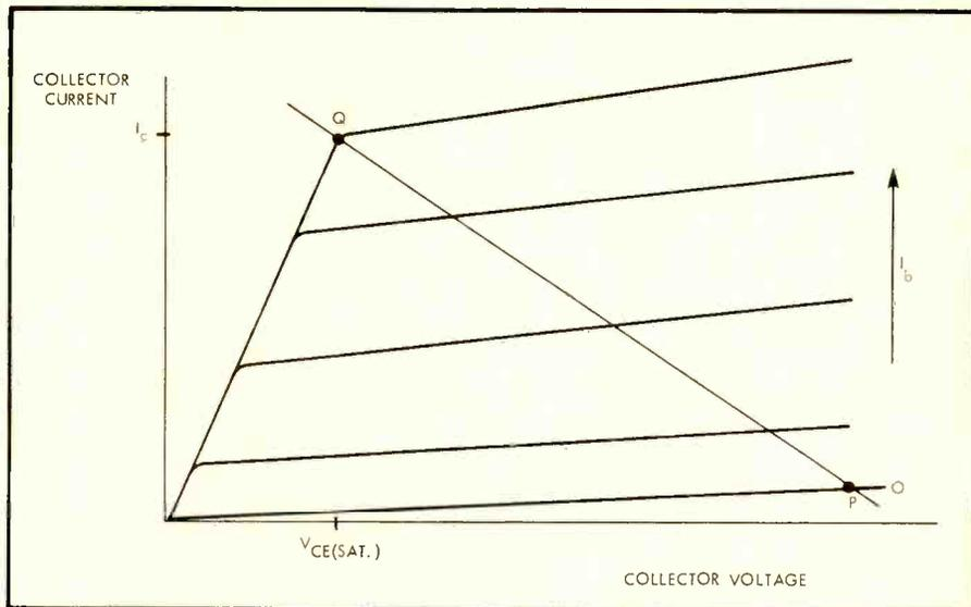
Fig. 2. Transistor characteristics and load line.
