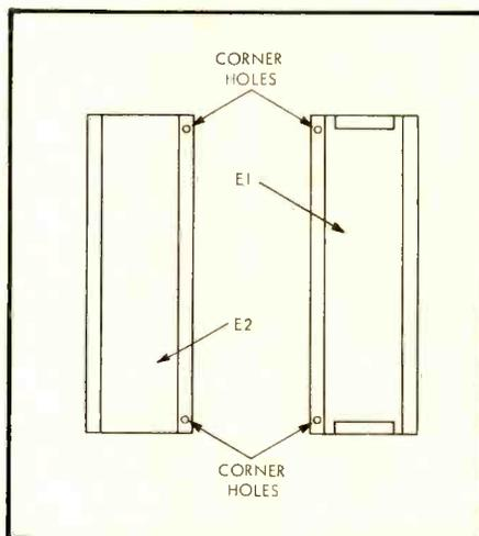
Fig. 4. Use corner holes to bolt electrodes together.
