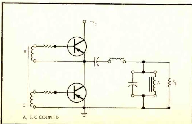
Fig. 11. Baxandall voltage-switching oscillator.
