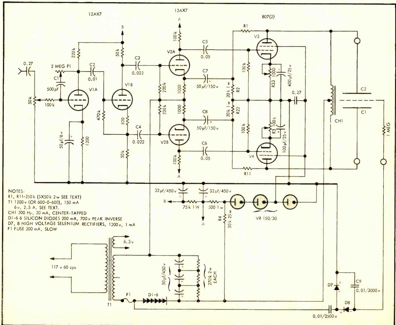
Fig. 12. Schematic of amplifier.
