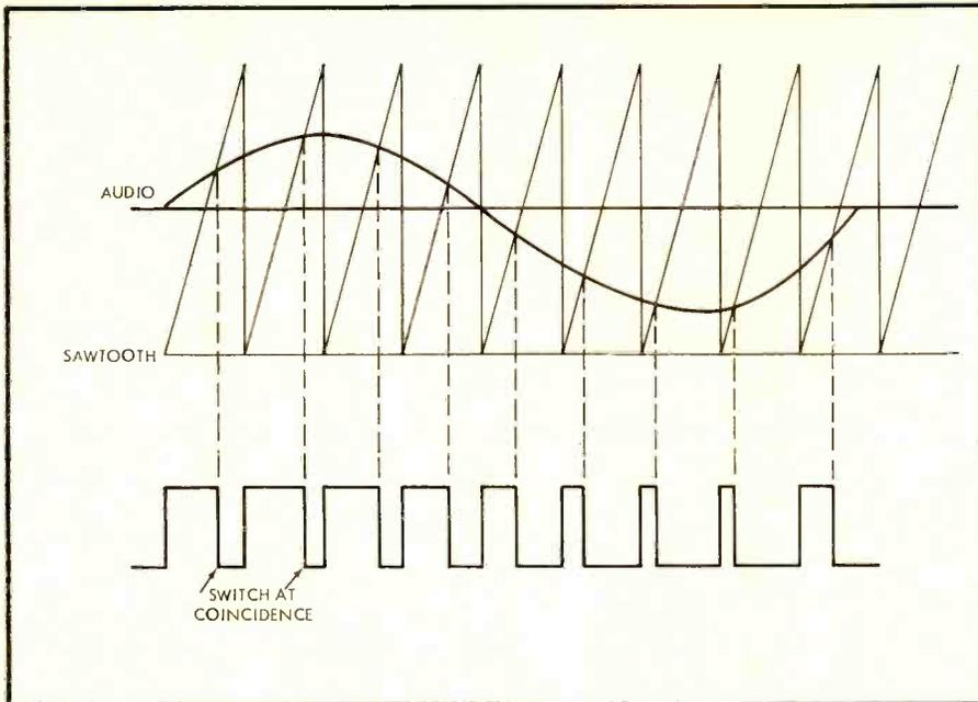
Fig. 7. Waveform produced by oscillator-modulator of type shown in Fig. 6.
