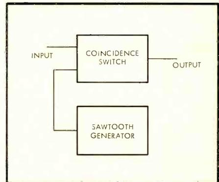
Fig. 6. Oscillator-modulator.
