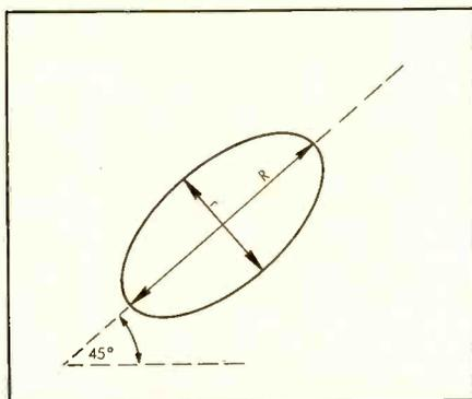
Fig. 2. Phase shift can be determined roughly by measuring the two axes of the ellipse and comparing with the table in the text.
