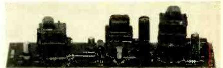
Fig. 2. View of one of the circuit boards showing the encapsulated modules.
