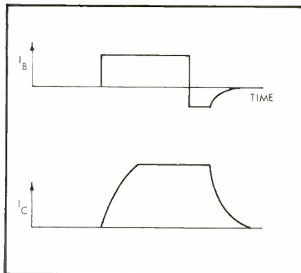
**Fig. 11.** "Classical" response of a transistor switched on and off at the base.
