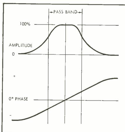
Fig. 7. Response of low-distortion filter. (Top of curve should be rounded instead of flat as shown.)
