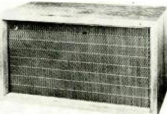
**Specifications:** infinite baffle enclosure; speakers—13 $\frac{1}{2}$ " x 8 $\frac{1}{2}$ " l.f., and m.f., (2) 3 $\frac{1}{2}$ " h.f., power handling capacity 20 watts rms; L-C crossover network; impedance 4 ohms; frequency response  $\pm 3$  db from 40 to 15,000 cps; finishes available and prices: walnut \$159.00; unfinished walnut \$154.00. Scope Electronics.
