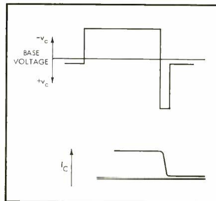
**Fig. 12.** The pulse recommended by Birt.
