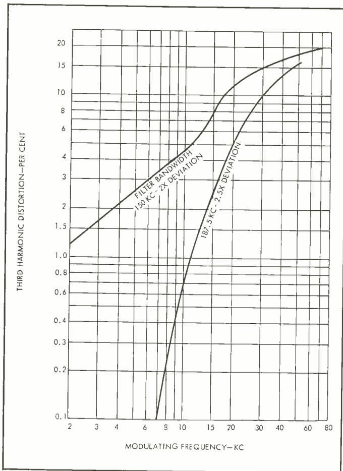
Fig. 6. Percentage third harmonic distortion of an FM carrier passing through an ideal filter as a function of modulating frequency, 75 kc deviation.
