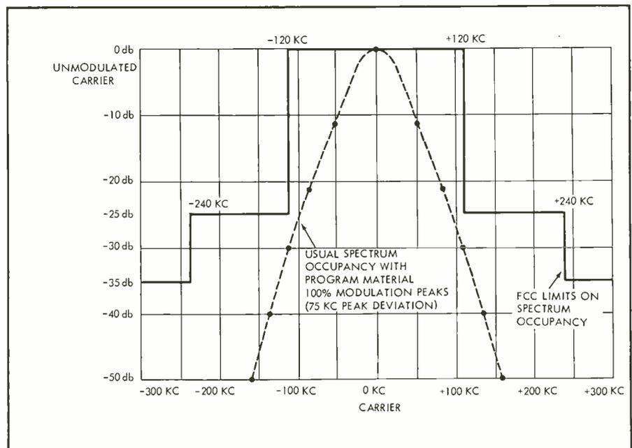
Fig. 2. FM spectrum occupancy. (Note unmodulated carrier refers to 0-db line.)
