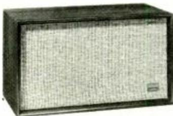
**Specifications:** acoustically-sealed enclosure; speakers—12" l.f., horn-loaded compression driver m.f., 5" h.f.; power handling capacity 30 watts; three-way etched circuit board crossover network; impedance 8 ohms; frequency response 30 to 20,000 cps; sensitivity
