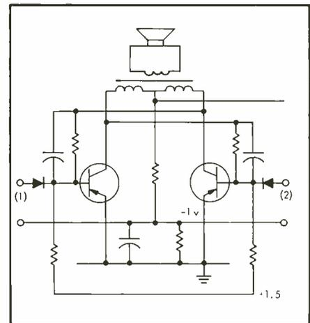
Fig. 13. Regenerative output stage.
