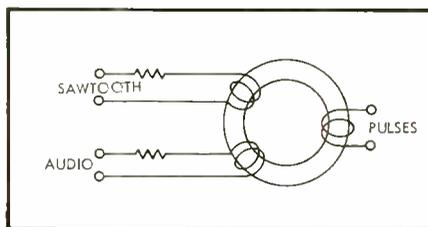
**Fig. 10.** This method gives short pulses, the 'sense' being opposite for the leading and trailing edges of the 1-m pulses.
