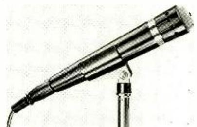
Specifications: dynamic; cardioid pattern; Mylar diaphragm material; aluminum case; anodized finish; output impedance variable; freq. resp. ±3 db from 50 to 12,000 cps; sensitivity -55 db; cable connection 3-pin; length of cable furnished 18 ft.; Cannon XLR-3-11 plug; dimensions—7½" by 1¾"; weight, 11 ozs.; standard ¾-27 mounting; other features: quick-detach microphone stand connector. Price, \$85.00. American Microphone.
