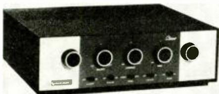
18 watts per channel; power output, rms, 15 watts per channel; harmonic distortion, 1% at 15 watts from 40 to 15,000 cps; 1M distortion, 2% at 15 watts; hum and noise, 75 db below 15-watt output; sensitivity input for rated output—phono, 5 mv, tuner, 0.15 volts; damping factor 8; output impedances, 4, 8, 16 ohms; input—1 phono, 1 tape head, 1 tuner, 1 aux, 1 xtal. Dimensions, 13 3/4" wide, 4 3/4" high, 11" deep. Price \$119.95. Grommes.
