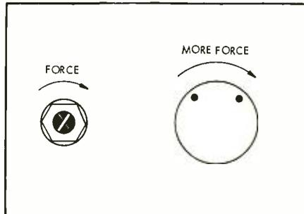
Fig. 1 Diagram showing the torque-amplifying characteristics of a properly chosen knob.
