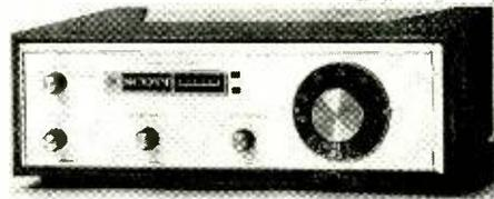
IHF usable sensitivity 1.9  $\mu$ v; AM suppression 60 db; harmonic distortion (100% mod.) 0.5%; stereo separation 30+ db; time-switching stereo circuit; drift 20 kc; dimensions in case: 15 1/2" wide, 15 1/4" high, 13 1/4" deep; weight, 14 lbs. Price \$279.95. H. H. Scott, Inc.
