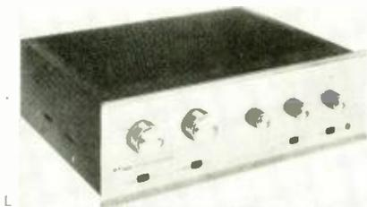
watts per channel; power output, rms, 17.5 watts per channel; harmonic distortion, 1% at 35 watts  $\pm 1$  db from 20 to 20k cps; 1M distortion, 1% at 35 watts; hum and noise, 80 db below 17-watt output; sensitivity, input for rated output—phono, 4 mv, tuner, 1 volt; damping factor 10; output impedances, 4, 8, 16 ohms; inputs—6 phono, 2 tape head, 2 aux, 2 radio; weight, 20 lbs. Dimensions, 13" wide, 4" high, 10" deep. Price \$139.95. Dynaco, Inc.
