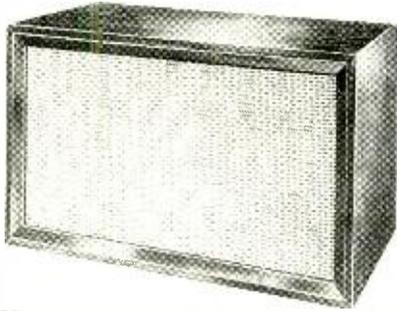
**Specifications:** Type of enclosure ducted port; speakers—12" l.f., 3" h.f.; power handling capacity 20 watts; type of crossover network LC; impedance 8 ohms; frequency response from 40 to 15,000 cps; magnet weight: l.f., 20 oz. Dimensions: 23 7/16" wide, 14" high, 13 5/16" deep; weight, 35 lbs; finishes available and prices: mahogany, walnut, blonde \$64.50; oil walnut, unfin. birch \$59.50. Lafayette Radio Electronics.
