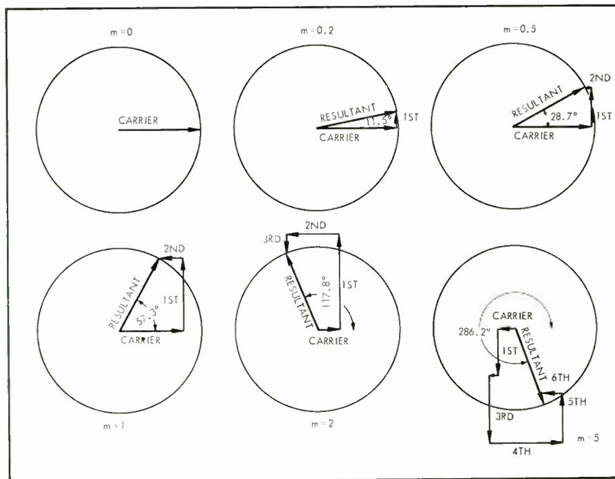
Fig. 3. Vectorial representation of a FM signal showing relation of carrier and its sidebands as a function of modulation index. (In representation of  $m = 5$ , the 7th and 8th sidebands have been omitted for clarity.)
