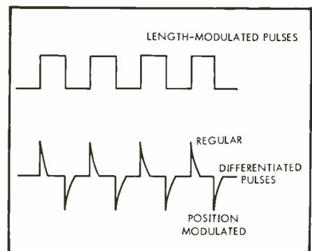
Fig. 14. Differentiated waveform needed to switch regenerative output stage.
