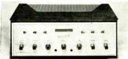
channel; harmonic distortion, 0.8% at 25 watts from 20 to 15k cps; 1M distortion, 0.8% at 25 watts; hum and noise 70 db below 35-watt output; sensitivity, input for rated output—phono, 3 mv, tuner, 0.5 volts; damping factor 4; output impedances 4, 8, 16 ohms; inputs—2 phono, 1 tape head, 1 tape amp, 1 aux, monitor; weight, 35 lbs. Dimensions, 17 1/2" wide, 6 1/4" high, 16 3/4" deep. Price, \$295.00. Cases in various woods and metals from \$17.95 to \$29.95. H. H. Scott, Inc.
