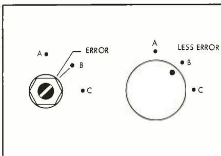
Fig. 2. Diagram showing how accuracy of resettability is increased by increasing the diameter of the indicating element of the torque-amplifying shaft turner.
