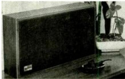
**Specifications:** ducted-port enclosure; speakers—10" l.f., 8" m.f., dome-radiator h.f.; power handling capacity 25 watts; L-C crossover network; impedance 8 ohms; frequency response 50 to 20,000 cps; magnet weights: l.f. 12 oz.; dimensions: 23 $\frac{1}{4}$ " wide, 13 $\frac{1}{2}$ " high, 5 $\frac{3}{4}$ " deep; weight, 25 lbs. Kit, \$52.50, wired \$62.50. EICO.
