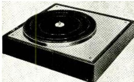
**Specifications:** Speeds—33½ rpm; rim drive; hysteresis-synchronous motor; turntable diameter, 12"; turntable weight, 12 oz.; turntable material, aluminum; Ring support mat; wow and flutter 0.1%; dimensions including base, 16½×15×3; provision for arm mounting, 2¼" internal clearance. Price, \$59.95. Weathers Ind.
