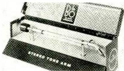
**Specifications:** Over-all length of arm, 12"; distance from arm axis to turntable spindle,  $8\frac{1}{4}$ "; height range of turntable, 0" to 2"; gimbal suspension; stylus force range, 0 to 4 gms; arm material, aluminum; pickup mounting, plug-in; overhang,  $\frac{1}{2}$ "; over-all weight, 1 lb. Price \$49.95, Dynaco.
