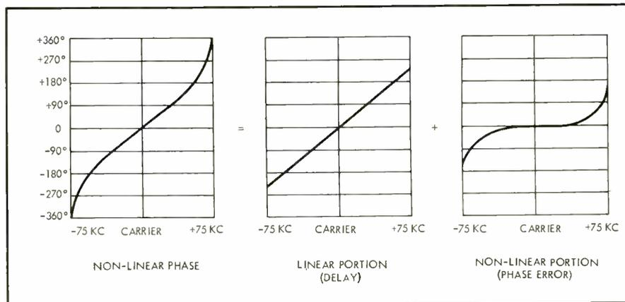
Fig. 4. Phase response of a non-linear phase filter.
