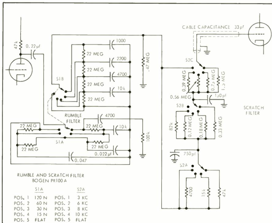
Fig. 1. Rumble and scratch filter.
