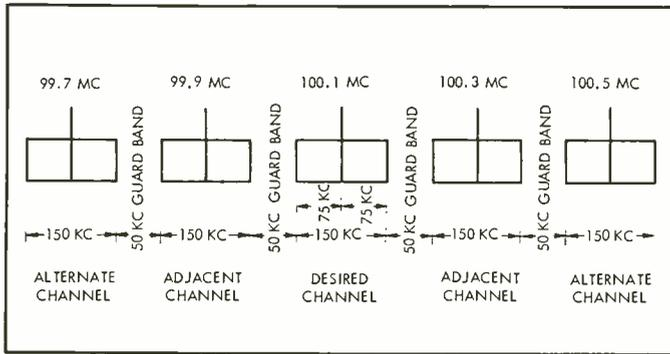
Fig. 1. FM channel assignments.
