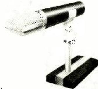
**Specifications:** dynamic; uni-directional pattern; output impedance 600/50k ohms; freq. resp.  $\pm$  1.5 db from 100 to 14,000 cps; sensitivity, -75  $\pm$  3 db (600 ohm); dimensions—1 $\frac{1}{4}$ " x 6 $\frac{7}{16}$ ". Primo Co.
