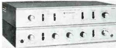
rms, 32 watts per channel; harmonic distortion, 1% at 25 watts from 30 to 25,000 cps; hum and noise, 75 db below 32-watt output; sensitivity, input for rated output—phono, 1.5 mv, tuner, 0.1 volts; damping factor 20; inputs—2 phono, 1 tape head, 1 tape amp, 2 aux, weight, 27 lbs. Dimensions, 15 $\frac{1}{4}$ " wide, 5 $\frac{1}{2}$ " high, 12 $\frac{1}{4}$ " deep. Price, \$199.95. A5-8.
