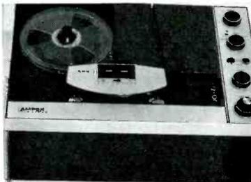
track mono; reel size 7"; 1 motor; timing accuracy 99.97%; freq. resp.—7 $\frac{1}{2}$  ips,  $\pm 2$  db from 30 to 18k cps; 3 $\frac{3}{4}$  ips,  $\pm 3$  db from 40 to 12k cps; 1 $\frac{1}{2}$  ips,  $\pm 3$  db from 40 to 6k cps; signal-to-noise ratio, 52 db; wow and flutter, 0.8% at 7 $\frac{1}{2}$  ips, 0.12% at 3 $\frac{3}{4}$  ips; rewind time, 1200-ft. reel, 115 sec. Inputs—2 microphone, 2 high level; amplifier outputs—2, high impedance. Price, less than \$439.00. A18-1.
