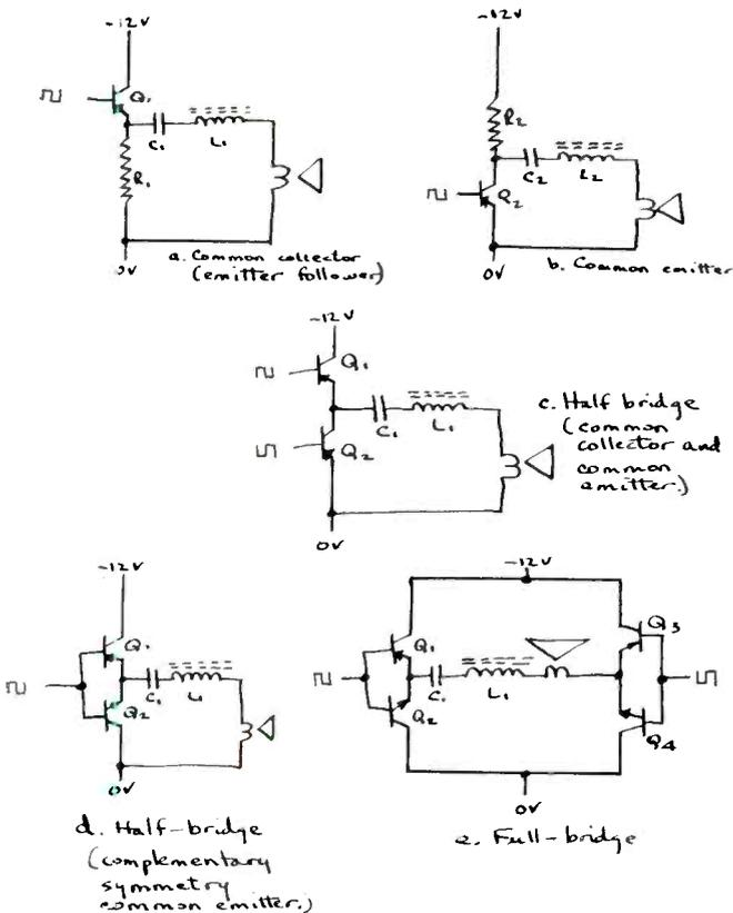
Fig. 20. Possible output stage circuits.
