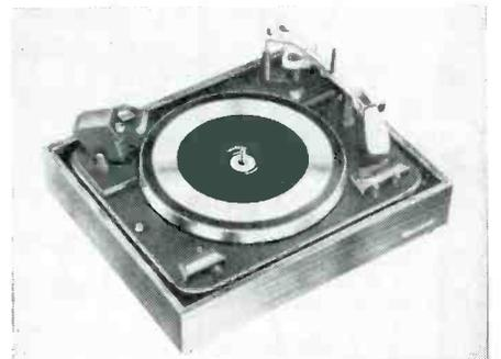
ribbed with chrome insert mat; dimensions of chassis, 16¾" x 14½"; clearance required above mounting board, 6"; below, 2¾"; type of mounting, barrel springs; controls, manual and auto on/off; automatic cycling time, 10 secs at 33½ rpm, 3½ sec at 78 rps; type of pickup head, plug-in 4 pin; material, plastic;
