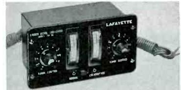
speaker levels. Does not load circuit. Individual attenuation controls, calibration switch. Size 6" W x 3/4" H x 2 7/8" D. Shpg. wt., 3 lb. Price \$7.95. A21-27.
