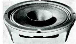
(watts input for +85-db level 10 feet on axis) 0.8 watts; magnet weight 6.0 oz. ceramic; voice-coil diameter 1 in.; free air resonance frequency 75 cps; recommended enclosure volume 1 $\frac{1}{4}$ -cu. ft. min. Dimensions 8 $\frac{1}{4}$ " dia. 3 3/16" deep; mounting dimensions, (4)  $\frac{1}{4}$ -in. holes on 7 $\frac{3}{8}$ " circle; cutout diameter 7"; weight, 4 lbs. Price \$15.00. A15-13.
