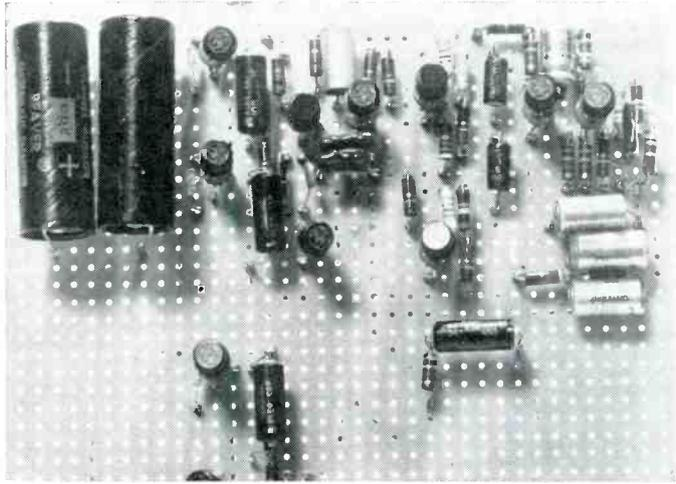
Fig. 26. Astable multivibrator amplifier.
