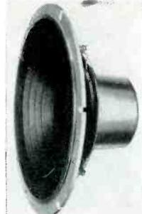
ohms; frequency response,  $\pm 3$  db from 30 to 2k cps; magnet weight 18 oz.; voice-coil diameter 1.3 in.; free air resonance frequency 40 cps; recommended enclosure volume 2.2 cu. ft. Dimensions: 11 $\frac{1}{4}$ " dia. 5" deep; mounting dimensions, 6 holes on 10 13/16" circle; cutout diameter 11 5/16"; weight, 10 lbs. Price \$37.00. A15-14.
