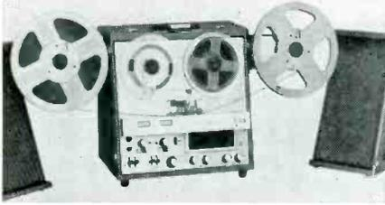
ratio, 50 db; wow and flutter, 0.2% at 7½ ips, 0.25% at 3¾ ips; rewind time, 1200-ft. reel, 45 sec. Inputs—2 microphone, impedance 3 meg; sensitivity 3 mv; 2 high level, impedance 1 meg; sensitivity 3 mv; amplifier outputs—2 preamp, impedance 22k ohms; speaker outputs 2, impedance 8 ohms; output power 8 watts per channel, A18-2.
