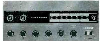
**Specifications:** Freq. resp. 50 to 15k cps db at 100 watts output; power output 100 watts per channel; harmonic distortion, 5% at 100 watts at 1000 cps; hum and noise, 83 db below 100 watt output; sensitivity, input for rated output-phonos, 3 mv; mic, 4 mv;
