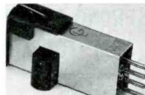
above 5k ohms; recommended tracking force professional arms, 1 gm, changers, 6 gms, effective stylus mass, 0.5 mg; compliance—lateral and vertical  $25 \times 10^{-6}$  cm/dyne; d.c. resistance, 1500 ohms; 4 terminals; mounting dimensions, std.; price, diamond, \$37.50. A11-8.
