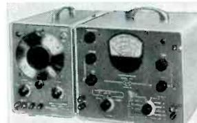
an amplifier of extremely low distortion. The Model 410 distortion meter measures harmonic distortion, noise level, audio gain or loss, and a.f. voltages. The circuit consists of a variable-frequency Wien bridge, followed by a calibrated attenuator and a vacuum-tube voltmeter. A21-7.
