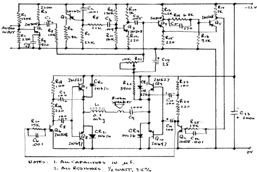
Fig. 21. Schmidt-trigger modulator amplifier schematic.
