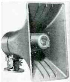
ohms; frequency response, 250 to 14k cps; EIA sensitivity 59 db; magnet weight 11.3 oz; voice-coil diameter 1.5 in.; dimensions 11" h x 6½" w x 8½" d; mounting, universal swivel bracket; weight, 5 lb. 9 oz. Price \$20.70. Accessories: TR3-2 25-volt line transformer, \$9.00; TR3-7 70.7-volt line transformer, \$9.00. CS4-2.
