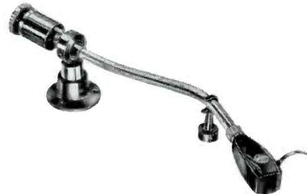
screw spacing, std; offset angle, 22.7 deg; overhang 5/8"; cartridge weight for zero adjustment preset 31 grams; maximum tracking error 1.19 deg; additional features, plug-in audio cables; arm resonance—8 cps, lateral and vertical; over-all weight 1 lb.; mounting dimensions, 3 hole, 1 1/2" centers. Price \$54.95; extra pickup beads, \$5.00. A12-8.
