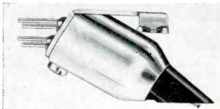
*Specifications:* Freq. response 20 to 20k cps  $\pm 3$  db; 1.5 mv/cm rec. velocity; channel separation, 30 db at 1 kc, 20 db at 10 kc; recommended load, 47k ohms; recommended tracking force—professional arms, 1.5 gms, chang-
