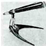
**Specifications:** Dynamic; omni-directional dir. pattern; mylar diaphragm material; die cast alum. case; satin black finish; output impedance 50, 150 or 250 ohms; freq. resp. 40 to 15k cps; output -57 db; cable connection Cannon XLR-3 lock latch; length of cable furnished 20 ft.; cable end serviced; dimensions—9 11/32" x 1 1/32" dia.; weight 8 3/4 oz.; stand adaptor for 3/8" x 27 thread and lavalier furnished. Price, \$150.00. A19-4.
