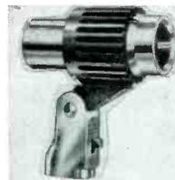
**Specifications:** Dynamic; cardioid dir. pattern; metal case; black and silver finish; output impedance 50k and 600 ohms; freq. resp. 90 to 10k cps; cable connection 2-conductor shielded; length of cable furnished 10 ft.; weight 2 lb.; standard 3/8"-27 mounting. Price, \$21.50. A19-11.
