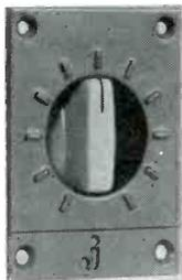
Load to 10-watts. Recessed flush knob. Paintable neutral sand finish. Ten 3-db stops of attenuation and off. Suitable for panel thicknesses up to ¾". CS5-3.
