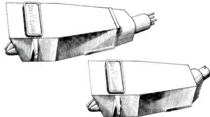
**Specifications:** Freq. response 20 to 17k cps  $\pm 2$  db; output 2 mv; channel separation, 35 db at 1 kc; recommended load, 47k-100k ohms; recommended tracking force—professional arms, 1-3 gms, changers, 3 gms; inductance, 245mh; d.c. resistance, 410 ohms; capacitance, 250 pf; 4 terminals; mounting std.; weight, 14 gms. Price, diamond, \$52.50; replacement styl, \$17.00. A11-14.
