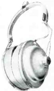
**Specifications:** freq. resp. 25 to 18k cps  $\pm 5$  db; impedance 8 ohms; sensitivity 0.1 mw; maximum power handling 250 mw; plug, standard phone; cord 6 ft.; price \$26.95. A20-4.
