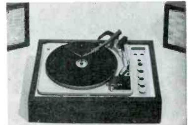
ance KLH speakers (2 in each enclosure). Solid-state stereophonic amplifier with an output of 15 watts music power and more than 30 watts peak. Other components include a new KLH changer built by Garrard, and a Pickering V-15 magnetic pickup with a diamond stylus. Controls are provided for vol-
