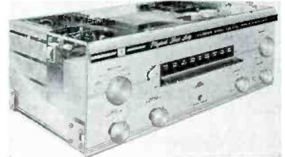
**Specifications:** Freq. resp. 20 to 20,000 cps  $\pm$  1 db; IHF music power output, 35 watts per channel; harmonic distortion, 1.5% at 25 watts from 20 to 10,000 cps; hum and noise, 84 db below 25 watts output; sensitivity, input for 25-watt output—phono, 4 mv, tuner, 400 mv; damping factor greater than 10; output impedances, 4, 8, 16 ohms; input—phono, tape head, tape amp, mic; weight, 24 lbs. Dimensions, 15" wide, 5 1/2" high, 11 3/8" deep. Price \$389.00. A5-2.
