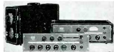
+1 db; power output, +18 dbm or 50 v. open circuit; input impedance 1 meg. channels 1-25 meg channels; source impedance 30/50 and 120/200 ohms with plug-in mic. transformer; load impedance, line out: 15 k ohms to infinity; noise level; input -123 dbm, output -68 dbm. Controls: 5 mixer, master, bass, treble, VU range, power; weight, 10¾ lbs. Dimensions. 19" wide, 5¼" high, 6¾" deep. Price, \$189.00. CS1-1A.
