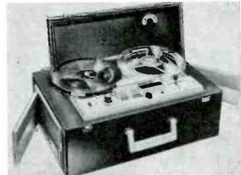
7½ ips; rewind time, 1200-ft. reel, sec. Inputs—2 microphone, impedance 50k ohms, 2 high level; monitor and speaker outputs, impedance 50k & 4 ohms; output power 1.5 watts. Dimensions, 16½" wide, 7½" high, 11" deep; weight, 27 lbs. Other features: two 4x6 oval speakers, vinyl case; complete with 2 dynamic mikes, patch cords, 7" reel. Price, \$129.50. A18-17.
