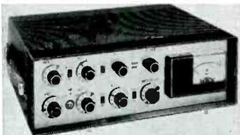
**Specifications:** Inputs: Mic 1, Mic 2, Mic 3, Mic 4, Mic 5, Mag, Xtal. Aux controls: Vol. 1, Vol. 2, Vol. 3, Vol. 4, Vol. 5; switches: selector, power; outputs: main, 10k ohms, freq. resp. 20 to 20k cps ±2 db; sensitivity, input for 1 volt output, phono, 4 mv, tuner, 0.5 volts; hum and noise, 70 db below 10 volt output. Weight, 21 lbs.; dimensions, 16 1/4" wide, 5 3/8" high, 13" deep. Price, \$246.25. CS1-2B.
