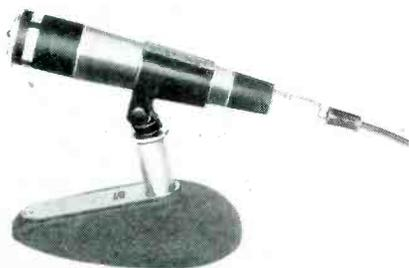
**Specifications:** dynamic; cardioid dir. pattern; baked enamel finish; output impedance 30/50, 150/250, 20k ohms; freq. resp. 45 to 15,000 cps; length of cable furnished 15 ft.; dimensions—1 1/2" dia., 7 1/4" long; weight 11 oz. Slip-on adapter mounting. Price, \$72.00. A19-2.
