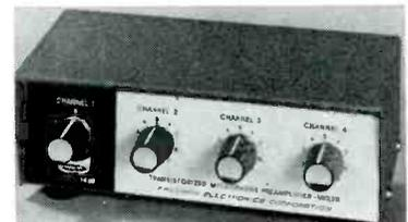
rehearsals. Four high-impedance channels, four independent controls; gain, 6 db; uses single 9-volt battery. Inputs—four standard phone jacks; output, one phono socket. Dimensions: 6" wide, 2 1/4" high, 3 1/2" deep, weight, 1 1/4 lbs. Price \$24.95. A21-18.
