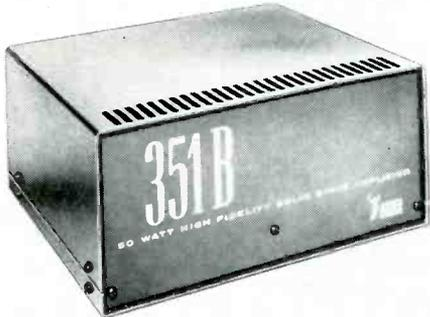
**Specifications:** Freq. resp. 20 to 20k  $\pm 1$  db; IHF music power output, 50 watts; harmonic distortion, 1.5% at 40 watts from 25 to 10k cps; hum and noise, 90 db below 50-watt output; sensitivity, input for rated output, 0.45 volts; damping factor, 7.5; output impedances, 4, 8, 16, 125 ohms, 70v; controls, level; switches, protective circuit; weight, 15 lbs; dimensions, 9 $\frac{3}{4}$ " wide, 5" high, 9 $\frac{1}{4}$ " deep; price, \$252.00. A1-2.
