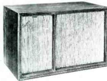
lbs.); m.f. and h.f. 20 oz. (1 $\frac{1}{4}$  lbs.) voice coil diameters: l.f. 2"; m.f. and h.f.  $\frac{3}{4}$ "; other features—sand filled panel to eliminate cabinet resonance, wire-wound "L" pad to balance high frequencies. Dimensions: 24" wide, 14 $\frac{1}{4}$ " high, 13" deep; weight, 50 lbs.; oiled or polished walnut \$122.50; utility model sanded birch \$106.50. Accessories B67 Universal Mounting Base in oiled or pol. walnut \$10.50; in sanded birch \$9.50. A17-37.
