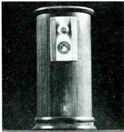
response  $\pm 3$  db from 20 to 20k cps; sensitivity (watts input for +85-db level 10 feet on axis) 1.0 watts at 1 kc.; magnet weights: l.f., 9 lb.; m.f., 2 1/2 lb.; h.f., 1 lb.; voice-coil diameters: l.f., 4"; m.f., 2 3/4", h.f., 1"; die cast wide angle acoustic lens for mid and high frequency direct radiators. Dimensions: 29" H, 22" diameter; weight 85 lbs.; hand-rubbed satin walnut \$250.00. A16-5.
