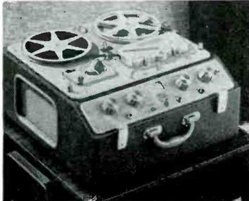
to 10k cps; signal-to-noise ratio, 52 db; wow and flutter, 0.16% at 7.5 ips; rewind time, 1200-ft. reel, 60 sec. Inputs—2 microphone, impedance 1 meg, sensitivity 2 mv; 2 high level, impedance 0.5 meg, sensitivity 50 mv; amplifier outputs—2, low level, impedance 1k ohms. Dimensions, 18½" wide, 9¾" high, 17½" deep; weight, 48 lbs. Provision for monitoring, re-recording from track to track. Price, \$595.00. A18-13.
