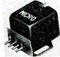
recommended load, 100 ohms; recommended tracking force—professional arms, 1-1.5 gms, changers, 2.5-3 gms; compliance—lateral and vertical  $6.0 \times 10^{-6}$  cm/dyne; d.c. resistance, 800 ohms; 4 terminals; mounting dimensions, EIA; weight, 10 gms. A11-10.
