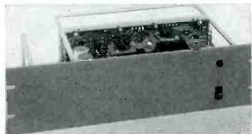
**Specifications:** Inputs: (2) mic (2) line; controls: (4) vol., bass, treble; switches: pwr., limit, outputs: main 0.25 ohms; freq. resp. 15 to 15k cps  $\pm 3$  db at 0.25 volts; IM distortion, 0.5% at 0.25 volts; sensitivity, input for 1 volt output, phono, 170 mv, tuner, 0.170 volts; hum and noise, -68 db below 0.25 volt output. Weight, 8½ lbs; dimensions, 19" wide, 7" high, 6" deep. Price, \$184.00. CS1-7B.
