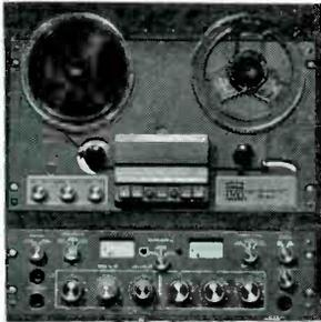
and flutter 0.2% at 7.5 ips, 0.25% at 3.75 ips; rewind time, 1200-ft. reel 80 sec. Inputs—2 microphone, impedance 50k ohms, sensitivity 2 mv; 2 high level, impedance 100k ohms, sensitivity 0.076 volts; amplifier outputs—2 emitter follower, impedance 2200 ohms. Dimensions, 19" wide, 15 3/4" high, 12" deep; weight, 47 lbs. Mic. jacks on front panel, mic. & line inputs mix & have master control. Price, \$595.00. Accessories: cases (1 for mechanism & 1 for amplifier) ea. \$30.00. A18-18.
