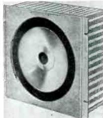
**Specifications:** metal cone concentric; power handling capacity 12 watts; impedance 16 ohms; frequency response  $\pm 3$  db from 30 to 17k cps; magnet weight 40 oz.; voice-coil diameter 1.5 in.; free air resonance frequency 55 cps. Dimensions 4" dia. 2" deep; mounting dimensions, 5 $\frac{1}{2}$ " x 5 $\frac{1}{2}$ " (rectangular); weight, 4 lbs. Price \$60.00. A15-21.
