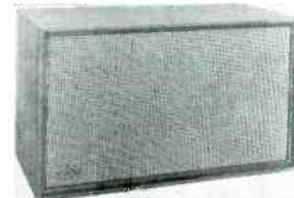
**Specifications:** infinite baffle enclosure; speakers—12" l.f., (2) 5" m.f., 2" dome h.f.; power handling capacity 60 watts; L-C air-core coils crossover network; impedance 8 ohms; frequency response 28 to 20k cps; voice coil diameter: l.f., 2"; eddy-current damping of woofer, hemispherical tweeter. Dimensions: 24.5" by 14" by 12" deep; weight, 60 lbs.; Scandinavian walnut, mahogany, cherry \$199.50; unstained birch \$189.50. A17-14.
