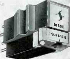
mended load, 47k ohms; recommended tracking force—professional arms, 1.25 gms, changers, 1.5 gms, effective stylus mass, 1.1 mg; compliance—lateral and vertical,  $25 \times 10^{-6}$  cm/dyne; inductance, 680 mh; d.c. resistance, 650 ohms; 4 terminals; mounting dimensions, std.; weight 7 gms. Price, diamond, \$35.00. A11-15.
