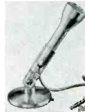
output impedance 250k ohms; freq. resp. 50 to 10k cps; sensitivity -58 db; length of cable furnished 7 ft.; phone plug; dimensions—1 9/16" dia., 5 1/4" long; weight 0.4 lbs; hand held unaffected by heat or moisture. Price, \$18.50. Accessories: CMS-10 stand (die-cast). Price, \$5.00. A19-19.
