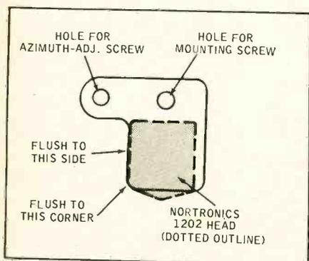
Fig. 12. Sketch of Nortronics 1202 head mounting on the head plate to indicate location. Head is epoxied onto the plate in the position shown.
