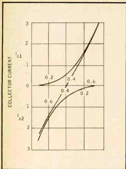
Fig. 4. Push-pull stage improves linearity by complementary matching of curves.
