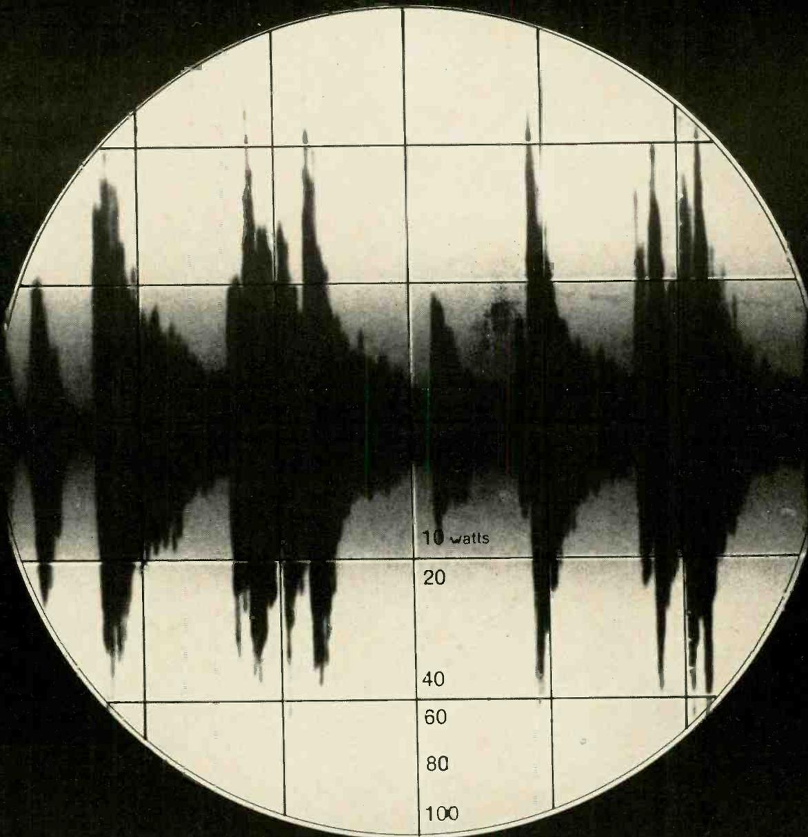
segment of oscillographic recording of Beethoven piano music displayed on screen of Hewlett-Packard 175a
