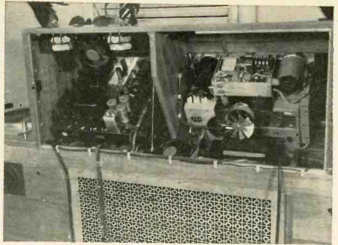
Rear view of the tape recorder-and-tuner panel. The smaller preamp is completely obscured by the tuner.
