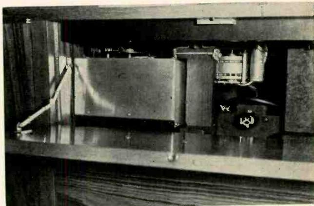
Electronic drive compartment under right turntable, with the drive unit shown at the left and the Papst turntable motor at the right.
