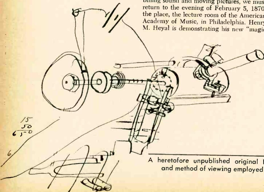
A heretofore unpublished original Edison sketch illustrating the construction and method of viewing employed in an early moving picture machine.
