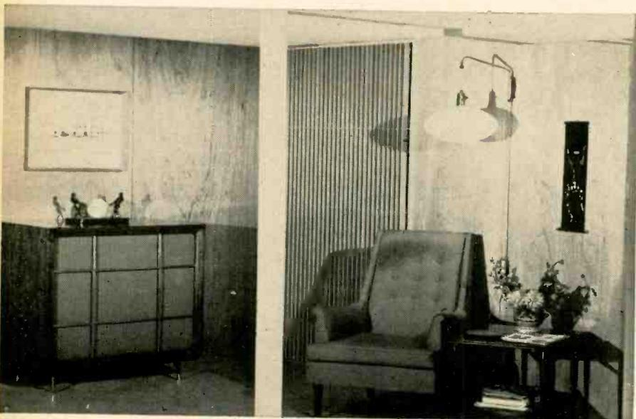
Fig. 3. Interior of listening room, showing mouth of horn. Grille discourages walking into the horn.
