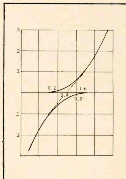
Fig. 5. Quiescent current (and dissipation) are reduced by lowering bias on stage of Fig. 4.
