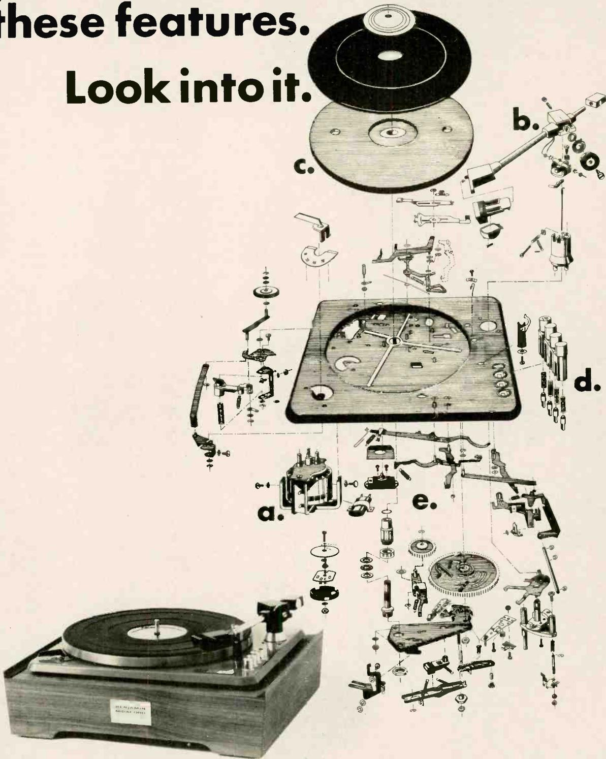
**a.** Hysteresis Motor. The 40H is the only automatic so equipped. Maintains accurate speed even with extreme voltage variations. Uses famous Papst motor, found in professional turntables and tape transports.
