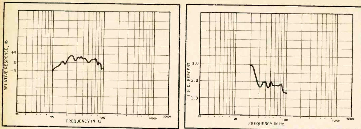
Fig. 4 (left). Averaged frequency response of bass-horn measured at a number of points in the listening room. Fig. 5, (right). Curve of harmonic distortion with 10-watt input.
