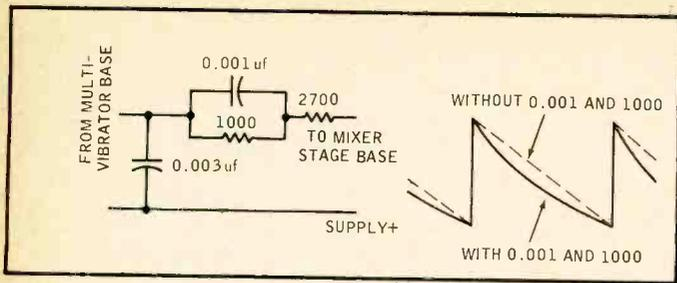
Fig. 2-10. Shaping the multivibrator pulse output to get sharper point, to better control the minimum pulse duration, at quiescent.
