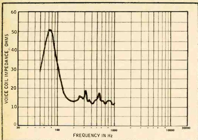
Fig. 6. Voice-coil impedance of bass-horn driver.
