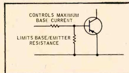
Fig. 2-6. A base-to-emitter shunt (resistor) can speed the delay due to storage time, in some transistors.
