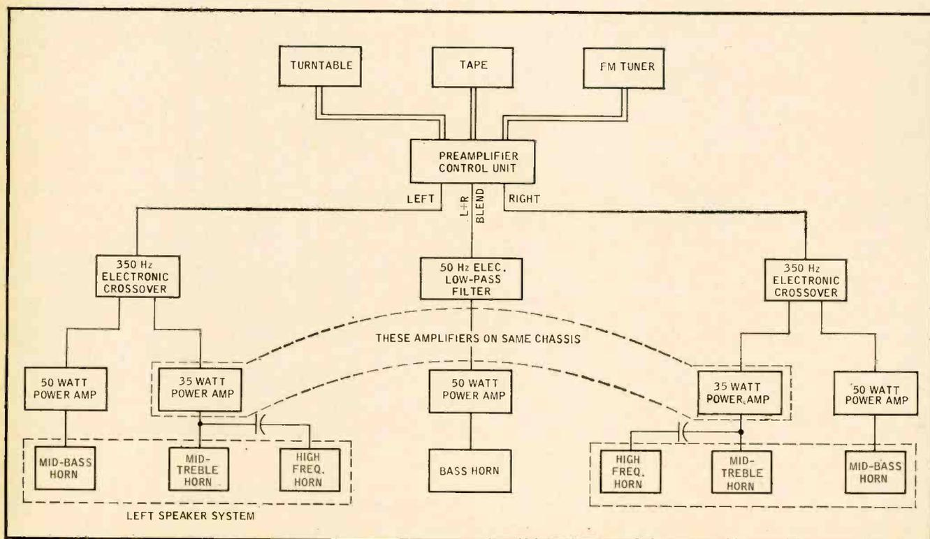
Fig. 7. Block diagram of complete audio system.
