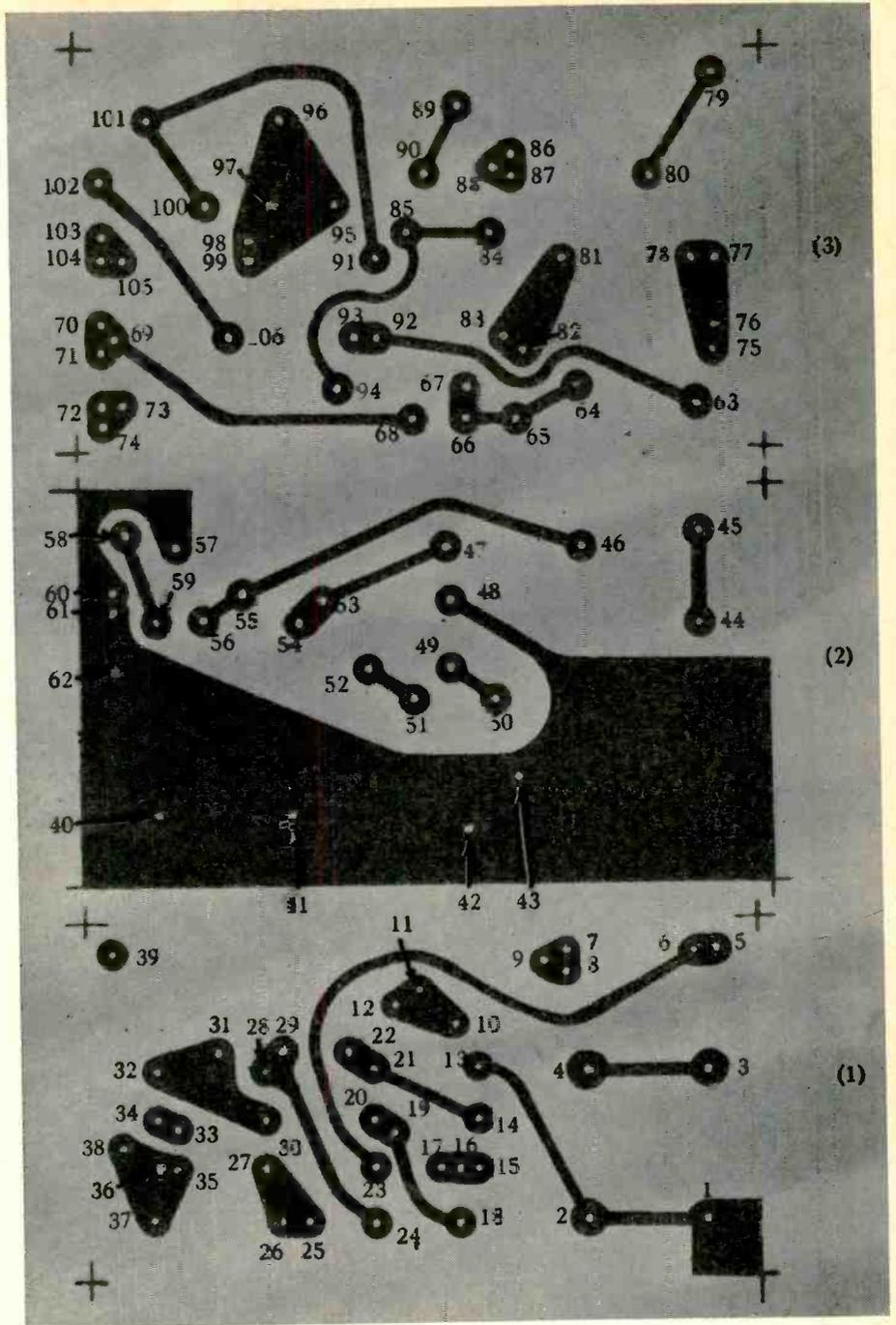
Fig. 5. Enlarged layout of printed circuit boards with the holes identified by number.
