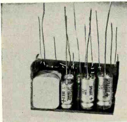
Fig. 10. Final view of left side of amplifier before putting top board in place.
