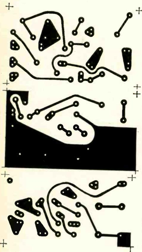
Fig. 4. Layout of the three printed circuit boards in the exact size required. Boards are identified from top to bottom as 3, 2, and 1.
