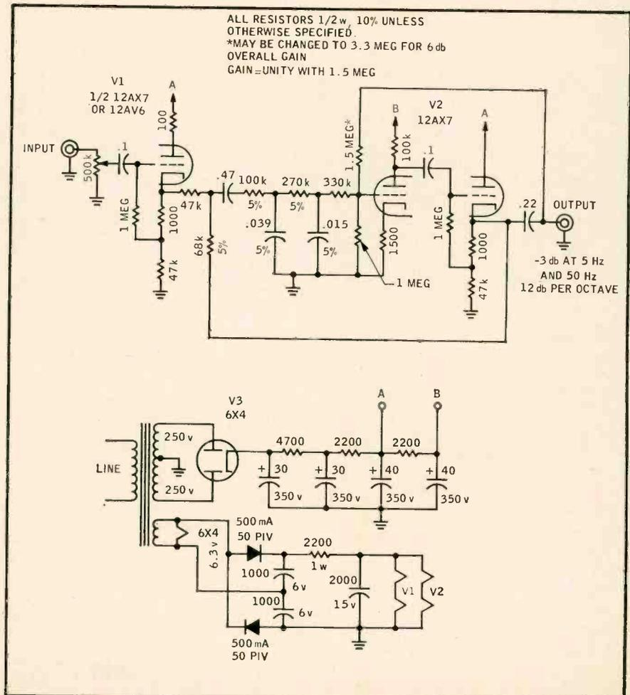
Fig. 9. 50-Hz low-pass filter in bass-horn circuit.
