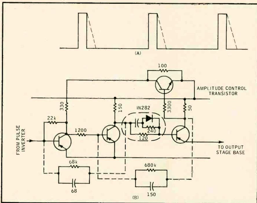
Fig. 2-12. Some details in development of satisfactory pulses: a. sloping trailing edge that occurs with no positive feedback to sharpen switching (dashed line); solid line shows effect of positive feedback; b. alternative ways of connecting positive feedback (values are those successfully used in those locations); in dashed ellipse is modified coupling between mixer and drive stage, to sharpen trailing edge of drive-stage pulse.
