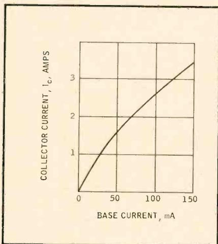
Fig. 2. Characteristic showing variation in small-signal current gain likely to cause excessive intermodulation.
