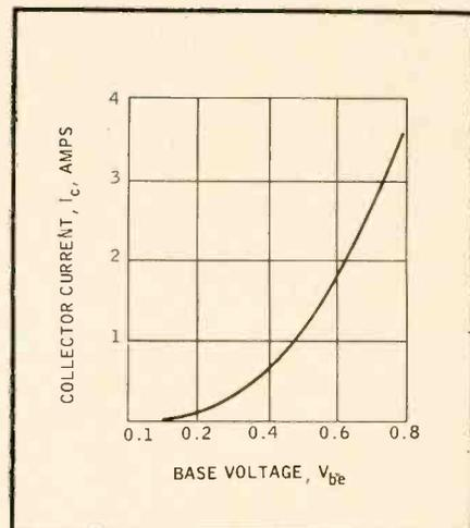
Fig. 3. Transistor similar to that of Fig. 2 driven by a high-impedance source results in this type of curve.
