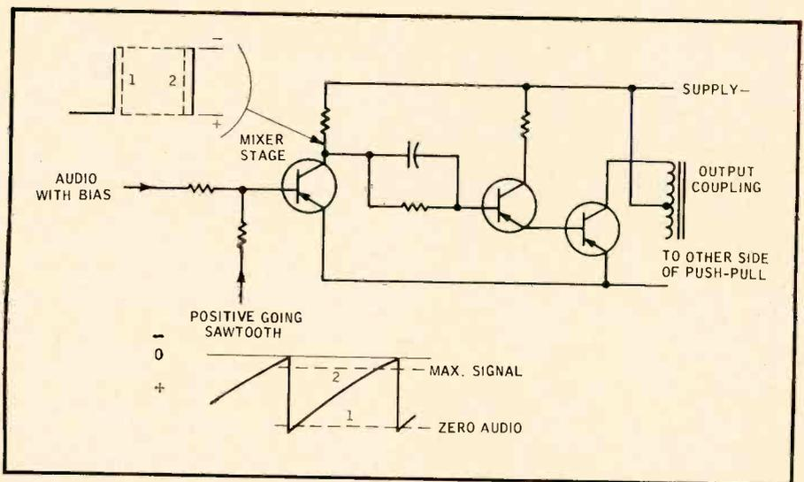
Fig. 2-9. Transmitting the modulation developed at the mixer stage to the output stage. The mixer stage (left) is normally conducting, saturated, and cuts off for pulses. The drive and output stage are normally cut off, pulse on to saturation. Variation of audio, combined with multivibrator pulses, varies the duration of the pulses transmitted.
