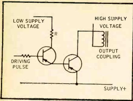
Fig. 2-7. Use of different supply voltages, when the output stage is collector coupled (grounded emitter). Resistor R limits drive-stage collector current, which is essentially output-stage base current.
