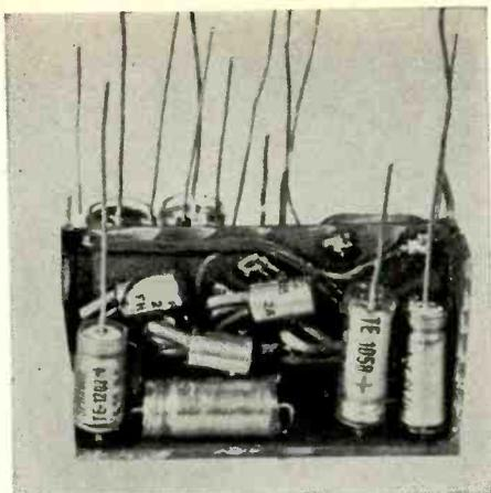
Fig. 9. View of the right side of the amplifier after all parts have been installed.
