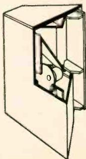
The construction of this horn is beyond compare. Nearly 288 screws, plus other fastening devices, plus high-grade adhesives, are used to make the horn as rigid as possible. Also each bass horn is checked with a water manometer to ensure absolute air tightness of the rear air chamber.
