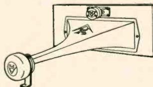
straight-axis design and is completely free of the irritating distortion which occurs in reflexed horns. The horn is mounted on a specially designed flange which effectively increases the horn's mouth area and adds measurably to its smoothness of response . . . less than 6 db variation from 400 to 5,000 cps.
