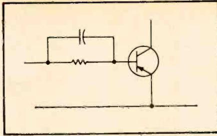
Fig. 2-3. A bypass capacitor can sometimes shorten either delay or storage time, or both.
