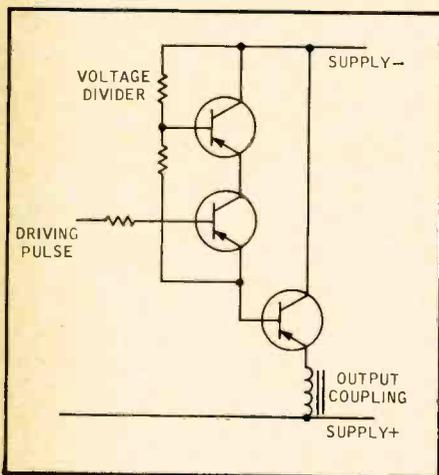
Fig. 2-8. Using two lower-voltage-rated transistors to serve on higher voltage by series connection. The two drive transistors shown here can withstand the full supply voltage needed to drive the output as an emitter follower, although their individual voltage rating is not high enough.
