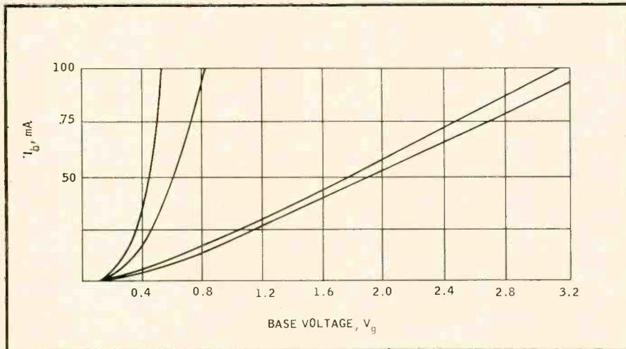
Fig. 8. By juggling source resistor values as well as emitter resistor, performance can be improved as in this set of curves.
