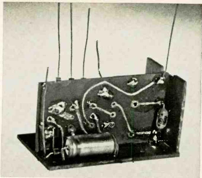
Fig. 6 (left). Initial step in construction with  $L_1$  and several of the resistors in place. Note end board, flush against  $L_1$  and the center board (1). Fig. 7 (right) earlier steps in construction as seen from the opposite side.
