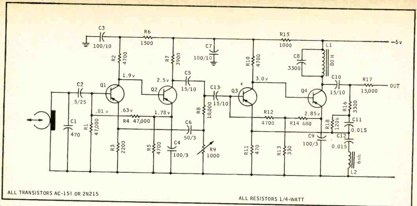
Fig. 3. Schematic of the auxiliary right-channel amplifier which is constructed on a printed-circuit-board "chassis" to fit into space required for a "D" cell.
