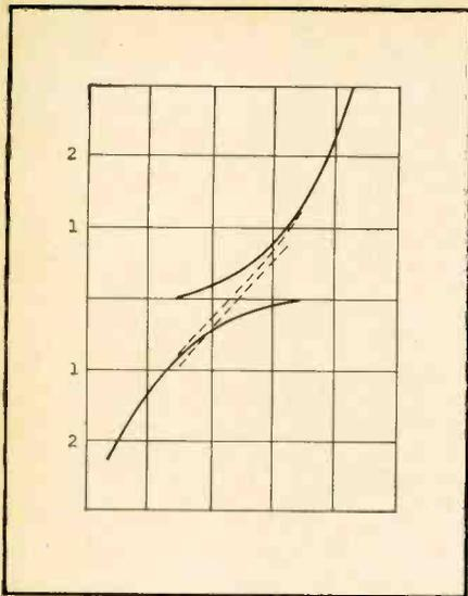
Fig. 6. Similar curve obtained with two actual transistors, in contrast to previous curves plotted from specifications for a "typical" transistor.
