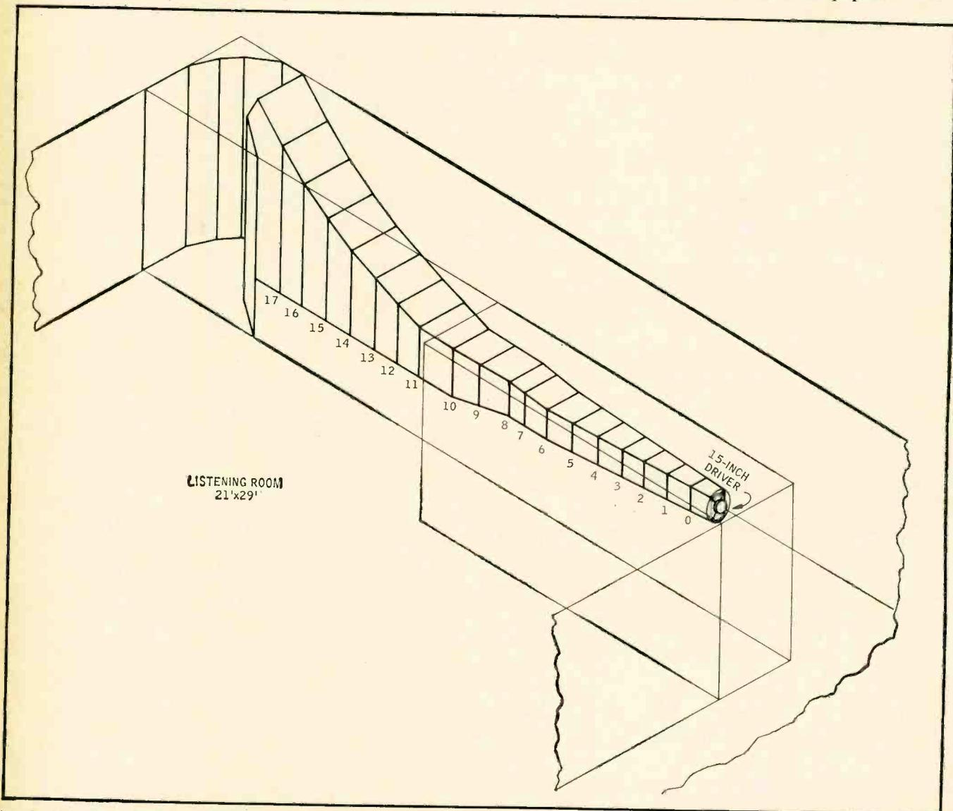
Fig. 1. Isometric diagram of bass horn and its "coupling" into the listening room. Note the 1-foot sections, each of which is a simple conical section, but together forming a hyperbolic horn.
