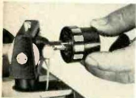
Lightweight tracking demands utmost perfection in tonearm balance. Dual achieves it with fine-thread adjust with nylon-braking, (no click stops) that takes full advantage of the virtually frictionless
