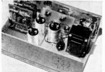
Step 1. Kit is designed so you can stop after wiring the easy-to-assemble power-amplifier stages, if you already own a hi-fi preamplifier. Construction time: about five hours.
