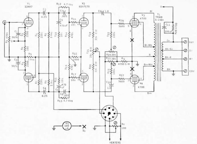
Fig. 5. Over-all schematic of the amplifier section.
