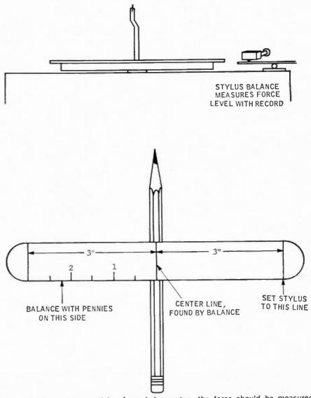
Fig. 9-1. Improvizing a stylus force balance: top, the force should be measured (balanced) with the stylus at the same level it occupies when playing the record; bottom, using a tongue depressor to make a balance that uses pennies.
