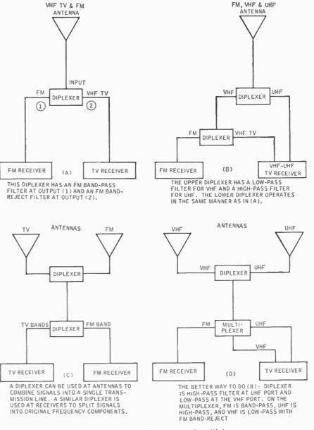
Fig. 29. Typical uses of diplexers and multiplexers.
