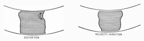
Fig. 9-7. The difference in irregularity of light pattern caused by distortion (A) or deviation in frequency response (B).
