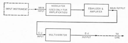
(B) TRIGGERING THE MULTIVIBRATOR WITH AN INSTRUMENT
