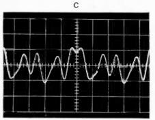
Fig. 4. Changes in phase alone can give a substantial difference in the "looks" of these three harmonic-rich waveforms.
