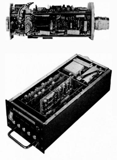
Fig. 1, showing the printed circuit modules of the GPL two-piece camera configuration. The modules in both the camera head, top, and the camera unit, bottom, are of the plug-in type and instantly replaceable.
