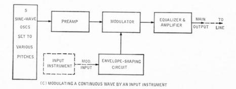
Fig. 8. Block schematics of typical applications of the complex-tone generator.
