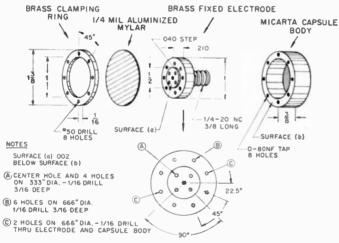
Fig. 4. Details of the author's capacitor microphone capsule.
