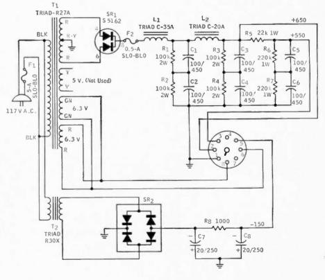
Fig. 6. Schematic of the power supply section,
