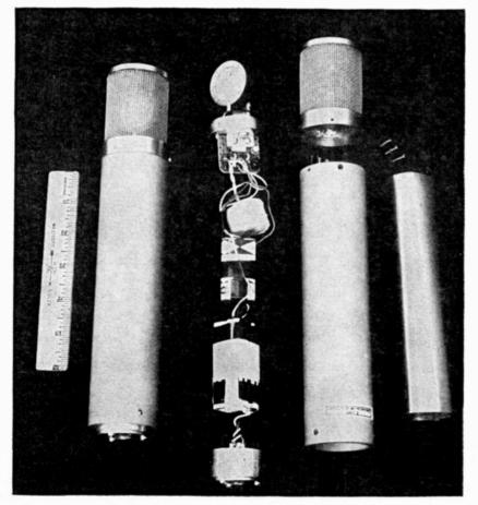
Two of the author's microphones, one of which is partially disassembled to show its internal layout.
