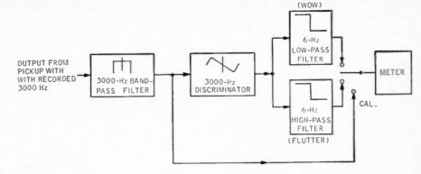
Fig. 9-12. How a flutter and wow meter works.
