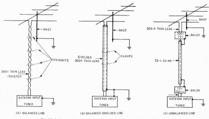
Fig. 24. Antenna system installations for three primary transmission line types.
