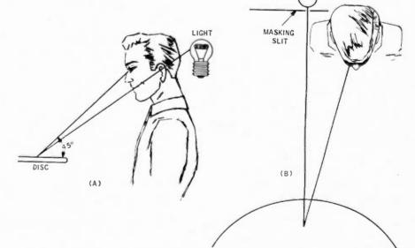
Fig. 9-5. (A) Viewing angle for observing light patterns, and (B) masking the light source to get a sharp pattern.
