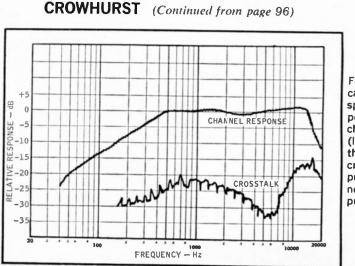
Fig. 9-10. A typical pair of responses—the upper curve is the channel response (left or right), and the lower is for crosstalk (left output in right channel or right output in left channel).
