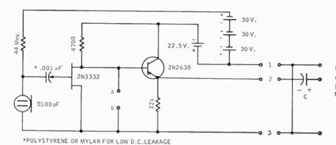
Fig. 1. The complete schematic for the author's microphone. The .001-µF capacitor marked with \* should be polystyrene or Mylar® for low d.c. leakage.
