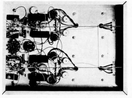
Fig. 2. Under-chassis view of the amplifier shows relatively neat construction.
