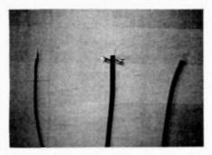
Fig. 22. Three major types of transmission lines—left, 300-ohm twin lead with a foam, weather resistant jacket; center, the same cable with an aluminum plastic outer jacket for shielding; and right, RG59/U coaxial cable, 72-ohm impedance.
