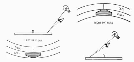
Fig. 9-6. Using the light-pattern method for stereo discs: each track may be viewed separately.
