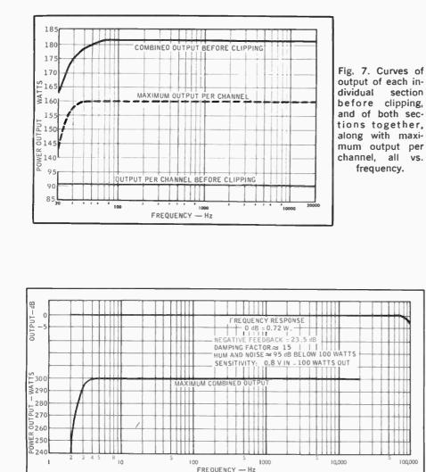
Fig. 8. Frequency response curves for 0.72 watts per channel, and for maximum combined output of both channels.
