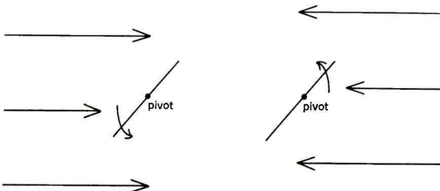
Fig. 11-6. Whichever way an air current approaches a free-floating disc at an angle from the back or front), the tendency is to turn it towards a position at right angles to the air movement. This is also true for vibrating air particles. So the disc is a means of measuring air particle velocity in a sound wave.
