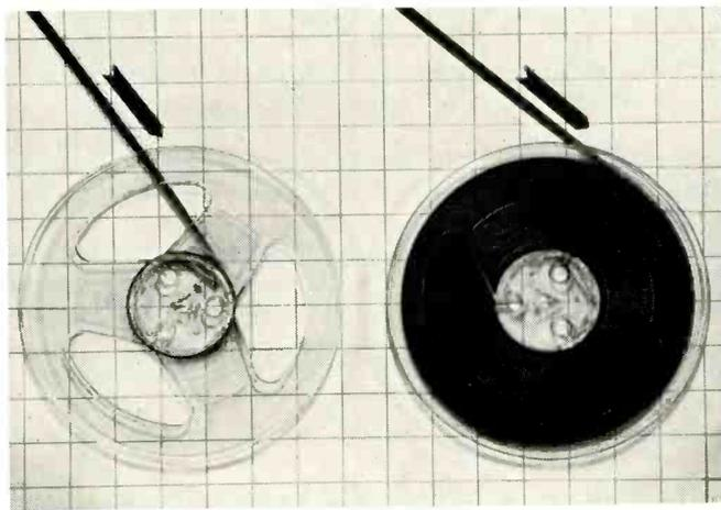
Fig. 1. If the clutch slippage of your take-up reel is poorly adjusted or sticking, the tape pull at the start of take-up (left) can be three times as strong as it becomes later in the take-up cycle.
