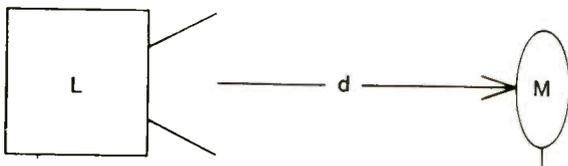
$$\begin{aligned} \text{Response C} &= \frac{L}{M} \\ A + B - C &= 2R \\ \frac{1}{2}(A + B - C) &= R \\ \frac{1}{2}(A - B + C) &= L \\ \frac{1}{2}(B - A + C) &= M \end{aligned}$$
