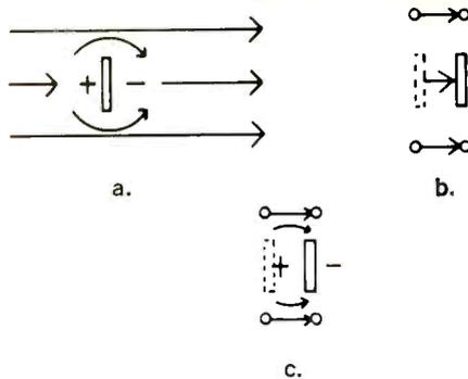
Fig. 11-3. The distinction between velocity and pressure gradient: (A) if the ribbon doesn't move, particle movement in the vicinity creates pressure gradient but not velocity; (B) if the ribbon moves with the air particles perfectly, then there is velocity without pressure gradient; (C) in practice, the ribbon doesn't move as much as the air particles around it, so both velocity and pressure gradient are present.
