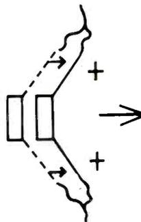
Fig. 11-4. The relationship in a free-cone speaker: movement of the diaphragm creates air pressure, or pressure gradient, which promotes particle movement or velocity.
