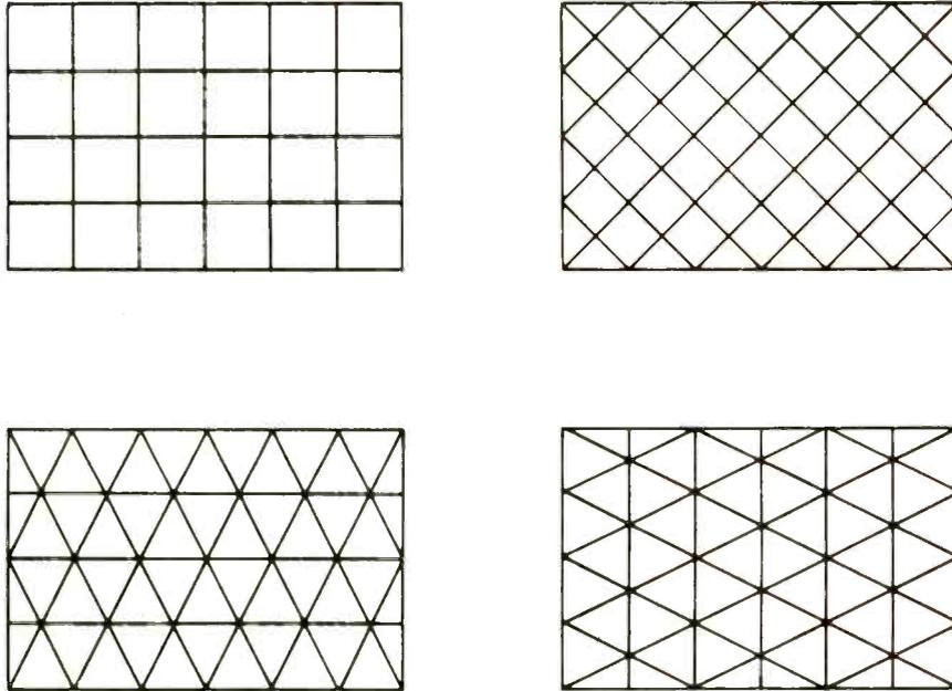
Fig. 11-1. Different standing-wave patterns that build up in the same space, due to different wavelengths corresponding to the different frequencies.
