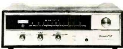
The march of transistor technology has not left the kit builder in the dust. Here is a new tuner kit from Scott that utilized an FET front end and is all-solid-state throughout. Scott states that it takes all of one afternoon to build the LT-112B FM-Stereo tuner kit. All difficult or critical circuitry is pre-wired, pre-tested, and pre-aligned at the factory.
