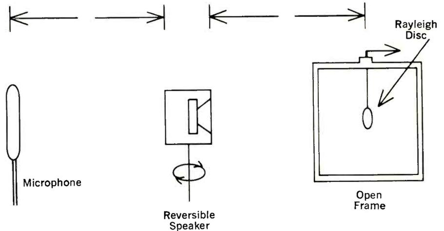
Fig. 11-7. Set-up for using a Rayleigh disc to calibrate the response of a microphone.
