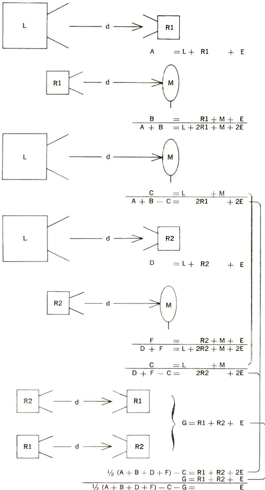
Fig. 11-9. The methods for determining room response or other environment effect.
