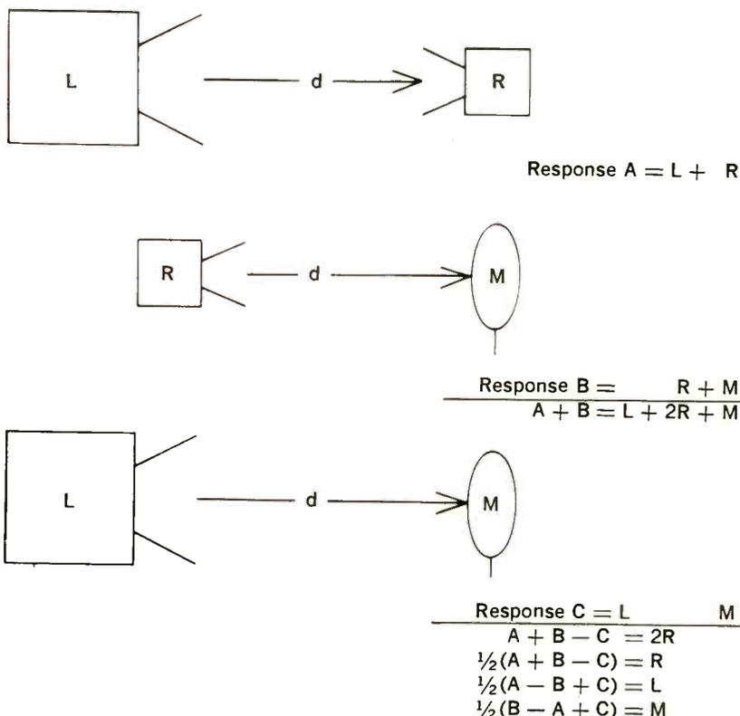
Fig. 11-8. Three measurements necessary for reciprocity test, with the basic calculations necessary to arrive at the microphone and loudspeaker responses.
