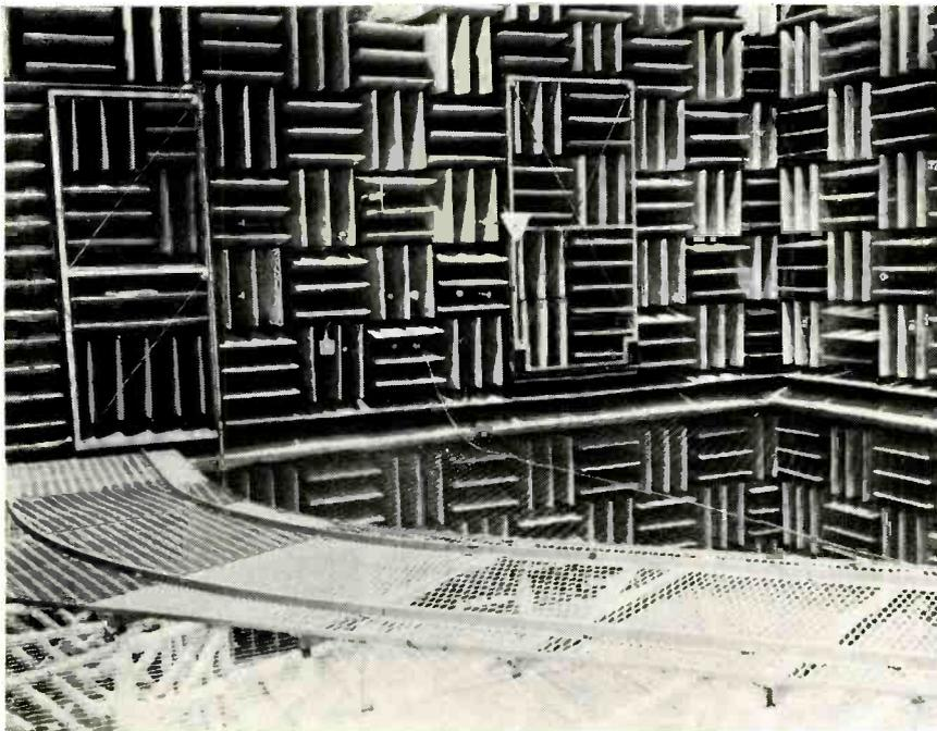
Fig. 11-2. View of a large anechoic chamber. The "dragon's tooth" wedges are made of a highly absorbent (acoustical) material. The expanded-metal or wire mesh floor provides support for equipment and anyone working on it.
