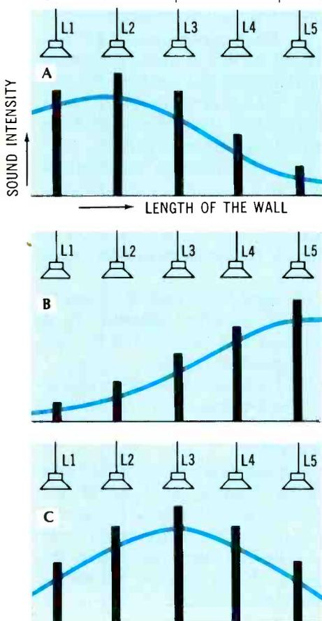
Fig. 3. Combined sound distribution patterns for the five loudspeakers.
