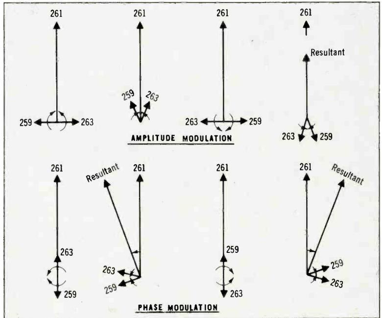
Fig. 7-4—Vectors to show the different phase relationships between the same steady-frequency components of amplitude modulation (tremolo) and frequency or phase modulation (vibrato).
