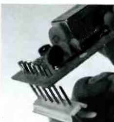
**Printed circuit modules snap into main chassis:**
