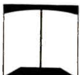
Ampex exclusive deep-gap heads consist of two *parallel* poles. Thus the gap remains constant after years of use.
