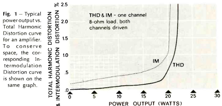
Fig. 1 — Typical power output vs. Total Harmonic Distortion curve for an amplifier. To conserve space, the corresponding Intermodulation Distortion curve is shown on the same graph.
