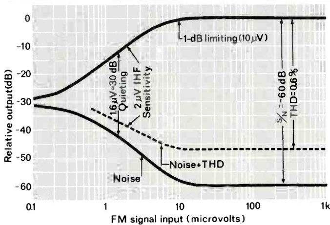
Fig. 3—FM performance characteristics of the NordMende Receiver.
